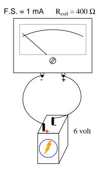
We know that connecting a sensitive meter movement directly across the terminals of a substantial voltage source (such as a battery) is a Bad Thing. So, I want you to determine what other component(s) must be connected to the meter movement to limit the current through its coil, so that connecting the circuit to a 6-volt battery results in the meter's needle moving exactly to the full-scale position:
