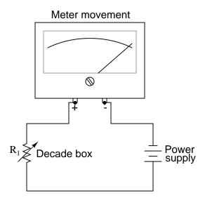
Then, connect a known resistance in parallel with the meter movement's terminals. This resistance will be known as  $R_s$ , the *shunt* resistance. The meter movement deflection will decrease when you do this. Readjust the decade box's resistance until the meter movement deflection returns to its former place. Record the decade box's resistance setting as  $R_2$ :
