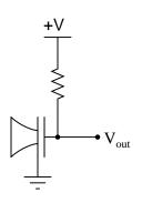
Vibrations in the air cause one metal plate to vibrate next to a stationary metal plate, rapidly changing the capacitance between the two plates. Explain how this simple circuit generates an AC voltage from this rapidly-varying capacitance, employing the mathematical relationship between charge (Q), capacitance (C)and voltage (V).
