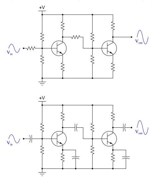
Which of these two designs would be more suitable for use in a DC voltmeter circuit (amplifying a measured DC voltage)? What applications would the *other* amplifier design be suited for?  $\frac{\text{file } 01119}{\text{file } 01119}$
