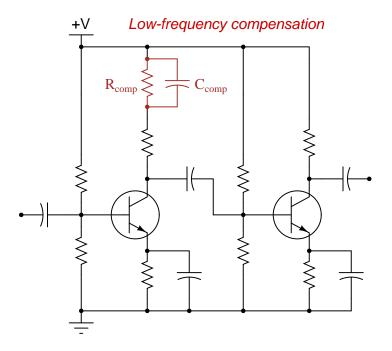
Explain how the presence of this "compensating" capacitor helps to overcome the loss of gain normally experienced as a result of the other capacitors in the circuit.  $\frac{\text{file } 01122}{\text{file } 01122}$
