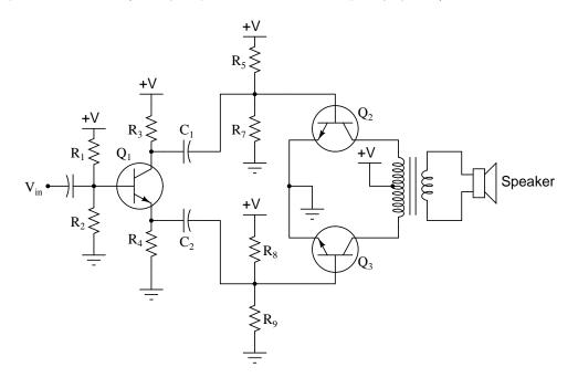
Unlike complementary-pair push-pull amplifier circuits, this circuit absolutely requires a preamplifier stage called a *phase splitter*, comprised here by transistor  $Q_1$  and resistors  $R_3$  and  $R_4$ .
