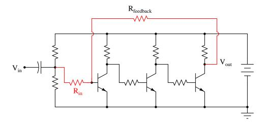
Interestingly, the voltage gain of such a circuit will be nearly equal to the quotient of the two highlighted resistors,  $R_{feedback}$  and  $R_{in}$ :
