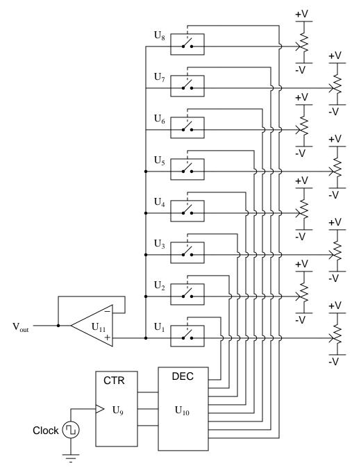
Explain what effect a shorted bilateral switch would have on the output waveform. Be as specific as possible.
