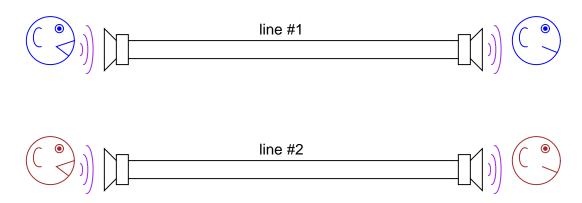
Suppose, though, we installed a set of DPDT switches that switched the two telephone conversations along the same pair of wires (only 1 telephone "line"). This general technique is known as *multiplexing*. The switches would be synchronized according to clocks at either end of the line, and cycled back and forth repeatedly:
