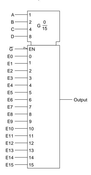
Show the wire connections necessary to make the multiplexer output the specified logic states in response to the data select (A, B, C, and D) inputs.
