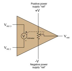
To elaborate further, imagine an extremely sensitive, analog, zero-center voltmeter inside the opamp, where the moving-coil mechanism of the voltmeter mechanically drives the potentiometer wiper. The wiper's position would then be proportional to both the magnitude and polarity of the difference in voltage between the two input terminals.
