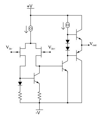
Qualitatively determine what will happen to the output voltage  $(V_{out})$  if the voltage on the noninverting input  $(V_{in+})$  increases, and the voltage on the inverting input  $(V_{in-})$  remains the same (all voltages are positive quantities, referenced to -V). Explain what happens at every stage of the op-amp circuit (voltages increasing or decreasing, currents increasing or decreasing) with this change in input voltage.
