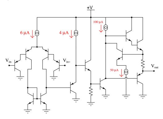
Qualitatively determine what will happen to the output voltage  $(V_{out})$  if the voltage on the inverting input  $(V_{in-})$  increases, and the voltage on the noninverting input  $(V_{in+})$  remains the same (all voltages are positive quantities, referenced to ground). Explain what happens at every stage of the op-amp circuit (voltages increasing or decreasing, currents increasing or decreasing) with this change in input voltage.
