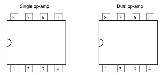
You will need to research some op-amp datasheets to find this information. Examples of single op-amp chips include the LM741, CA3130, and TL081. Examples of dual op-amp chips include the LM1458 and TL082.
