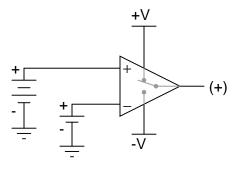
In these illustrations, I have likened the op-amp's action to that of a single-pole, double-throw switch, showing the "connection" made between power supply terminals and the output terminal.
