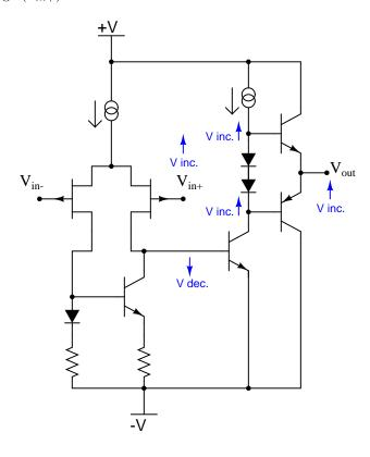
Here, I've labeled a few of the important voltage changes in the circuit, resulting from the increase in inverting input voltage  $(V_{in-})$ :
