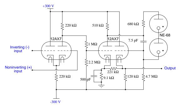
To make this opamp circuit easier for modern students to understand, I'll substitute equivalent solid-state components for all tubes in the original design:
