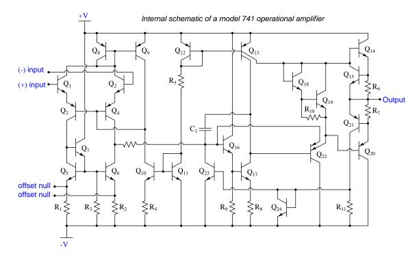
Predict how the operation of this operational amplifier circuit will be affected as a result of the following faults. Specifically, identify whether the output voltage  $(V_{out})$  will move in a positive direction (closer to the +V rail) or in a negative direction (closer to ground). Consider each fault independently (i.e. one at a time, no multiple faults):
