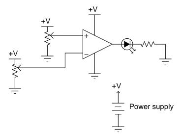
Trace the complete path of current powering the LED. Where, exactly, does the LED get its power from?
