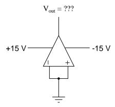
In reality, the output voltage of an op-amp under these conditions is not the same as what would be ideally predicted. Identify the fundamental problem in real op-amps, and also identify the best solution.
