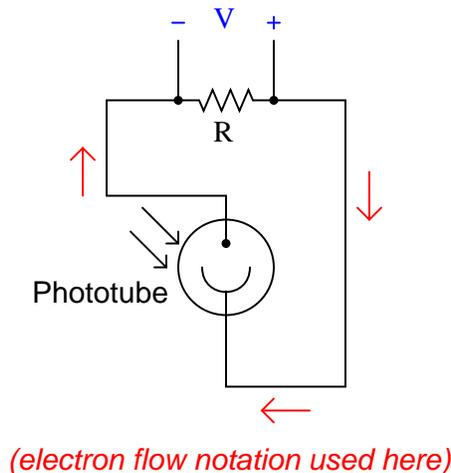
The current output by such a phototube is *very* small, and the voltage output by it is smaller yet. If we are to measure current through this device, we will have to find some way other than a shunt resistor to do it.
