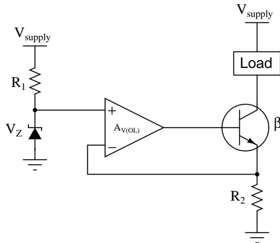
Write an equation solving for the regulated load current, given any relevant variables shown in the schematic diagram ( $R_1$ ,  $V_Z$ ,  $V_{supply}$ ,  $A_{V(OL)}$ , etc.).
