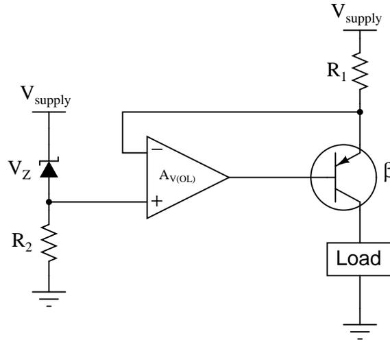
Write an equation solving for the regulated load current, given any relevant variables shown in the schematic diagram ( $R_1$ ,  $V_Z$ ,  $V_{supply}$ ,  $A_{V(OL)}$ , etc.). Also, describe what would have to be changed in this circuit in order to set the regulated current at a different value.
