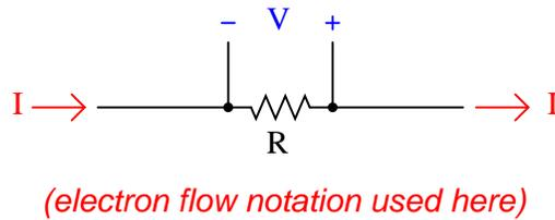
Precision resistors typically work very well for this purpose, especially when the amount of voltage dropped across it is of little consequence. This is why *shunt resistors* are frequently used in power circuitry to measure current, a low-resistance "shunt" resistance element dropping voltage in precise proportion to the current going through it.
