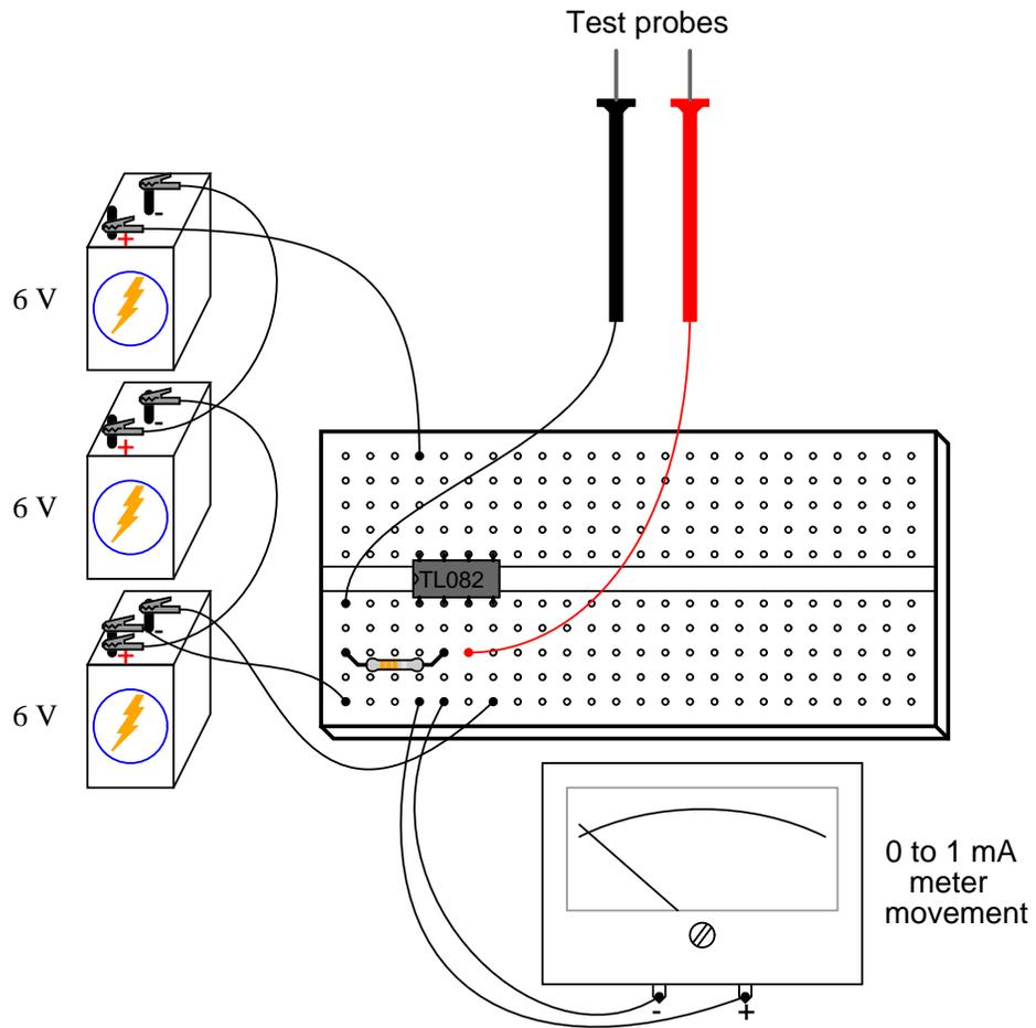
Draw a schematic diagram of this circuit, and calculate the resistor value necessary to give the meter a voltage measurement range of 0 to 5 volts.
