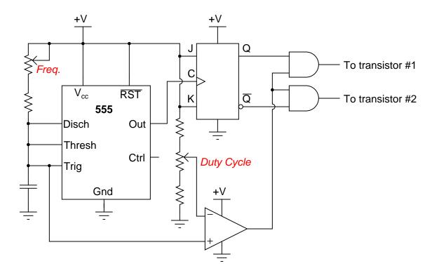
Follow-up question: which direction would you have to move the frequency potentiometer to increase the output frequency of this circuit? Which direction would you have to move the duty cycle potentiometer to increase that as well?
