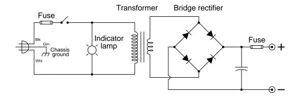
Of course, you are not restricted to using this exact design. One design feature I insist on, though, is that you build your own rectifier circuit from individual diodes, rather than use a packaged rectifier assembly. I highly recommend the use of "barrier strips" or "terminal strips" to make the electrical connections between components. These connection devices provide solid, permanent electrical connections while still allowing components to be easily installed and removed.
