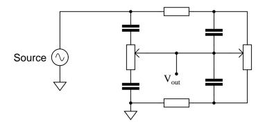
Determine which potentiometer controls the bass (low frequency) tones and which controls the treble (high frequency) tones, and explain how you made those determinations. file 03506
