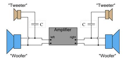
Follow-up question: what type of capacitor would you recommend using in this application (electrolytic, mylar, ceramic, etc.)? Why?
