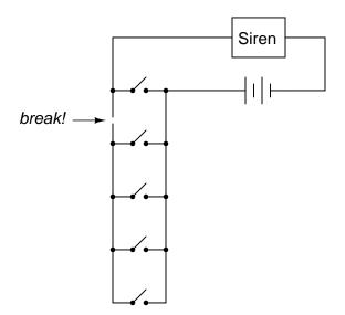
Suppose an engineer designed a fire alarm system for a large warehouse, with multiple pushbutton switches connected to a single alarm siren:
