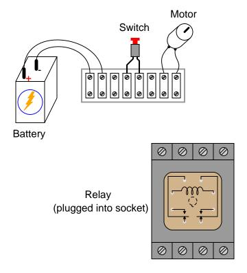
Suppose that an electromechanical relay has a coil voltage rating of 5 volts, and a coil resistance of 250  $\Omega$ . However, you desire to energize this relay with a 24 volt power supply. You know that a series-connected resistor might enable the 5-volt relay coil to be powered by the 24-volt supply without damage, but you do not know what size of resistor would be appropriate for the task.
