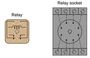
Draw the necessary connecting wires between terminals in this circuit, so that actuating the normally-open pushbutton switch will energize the relay, which will in turn supply electrical power to the motor.
