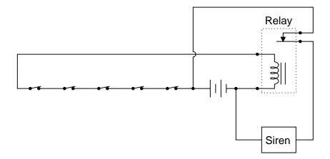
Actuating any of the normally-closed switches results in the alarm sounding. So far, so good. Now, suppose that one of the wires connecting one side of several switches to the rest of the circuit breaks open. What will the result of this failure be?
