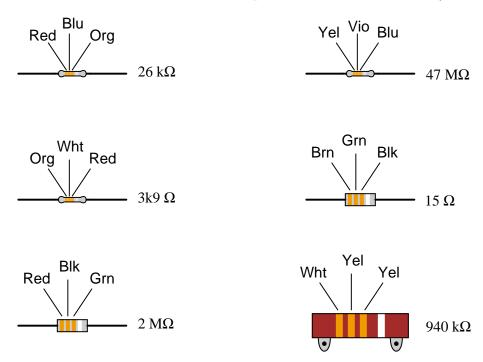
What patterns do you notice between the color codes (given as three-letter abbreviations, so as to avoid interpretational errors resulting from variations in print quality), the resistance values, and the physical sizes of the resistors?
