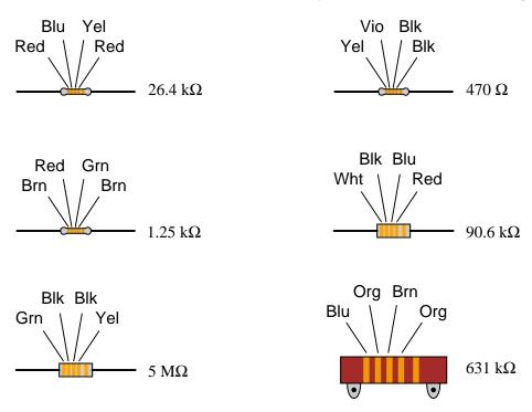
What patterns do you notice between the color codes (given as three-letter abbreviations, so as to avoid interpretational errors resulting from variations in print quality) and the resistance values of each resistor? Why do precision resistors use a "5-band" color code instead of a "4-band" color code? <u>file 00265</u>
