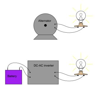
However, when measured by an analog voltmeter, the inverter's output voltage is slightly greater than the alternator's output voltage. Explain this discrepancy in measurements.
