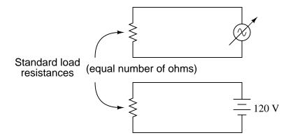
In this condition of equal power dissipation, how much voltage is the AC power supply outputting? Be as specific as you can in your answer.
