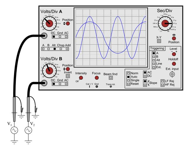
While this feature is extremely useful, one must be careful in connecting two sources of AC voltage to an oscilloscope. Since the "reference" or "ground" clips of *each* probe are electrically common with the oscilloscope's metal chassis, they are electrically common with each other as well.
