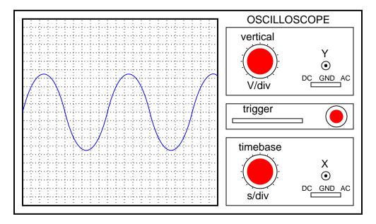
The core of an analog oscilloscope is a special type of vacuum tube known as a *Cathode Ray Tube*, or *CRT*. While similar in function to the CRT used in televisions, oscilloscope display tubes are specially built for the purpose of serving an a measuring instrument.
