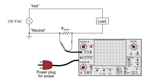
Most oscilloscopes have at least two vertical inputs, used to display more than one waveform simultaneously:
