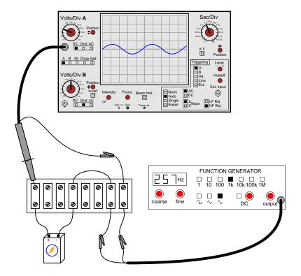
Something is wrong with this circuit. Based on the oscilloscope's display, determine whether the battery or the function generator is faulty:
