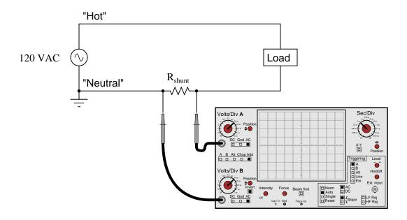
Failing to consider that the "ground" leads on all probes are common to each other (as well as common to the safety ground conductor of the line power system) is a *very* common mistake among students first learning how to use oscilloscopes. Hopefully, discussing scenarios such as this will help students avoid this problem in their labwork.
