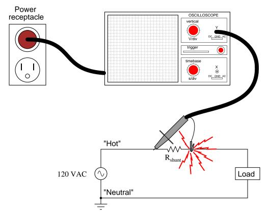
Here, the reference lead of the oscilloscope (the small alligator clip, not the sharp-tipped probe) creates a short-circuit in the power system. Explain why this happens.  $\underline{\text{file }01820}$
