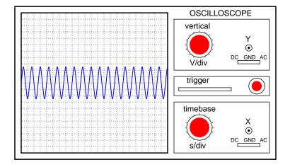
What display control(s) need to be adjusted on the oscilloscope in order to show fewer cycles of this signal on the screen, with a greater height (amplitude)?  $\frac{\text{file }00532}{\text{file }00532}$
