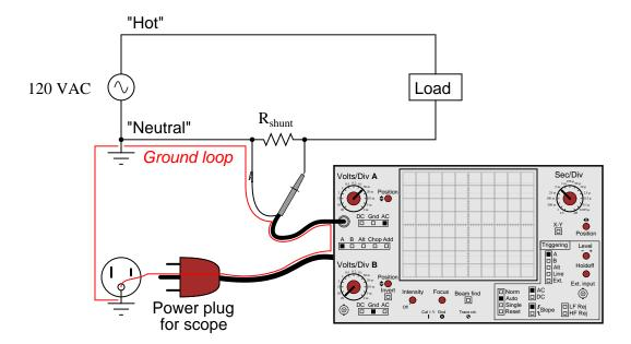
Ground loops are to be avoided in measurement circuits because they may be the source of some very strange effects, including the coupling of noise voltage from entirely unrelated circuits to the one being measured. To avoid this problem, the best solution for measuring the voltage dropped across the shunt resistor is to use two scope probes and set the scope up for differential voltage measurement:
