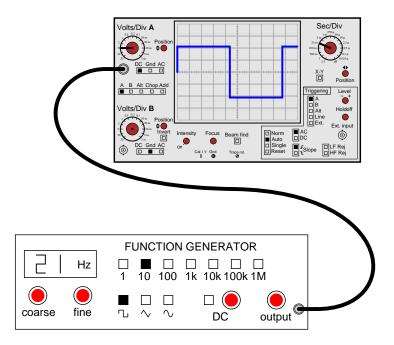
It is then that the student realizes the first oscilloscope has its "coupling" control set to AC, while the second oscilloscope was set to DC. Now the student is really confused! The signal is obviously AC, as it
