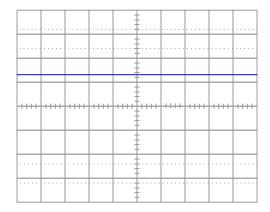
Assuming the oscilloscope display has been properly "zeroed" and the vertical sensitivity is set to 5 volts per division, determine the voltage of the battery.
