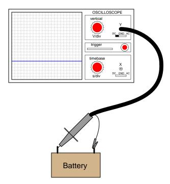
An oscilloscope is connected to a battery of unknown voltage. The result is a straight line on the display:
