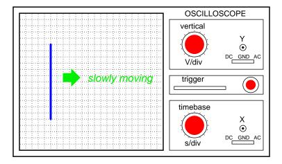
What appears on the oscilloscope screen is a vertical line that moves slowly from left to right. What display control(s) need to be adjusted on the oscilloscope in order to show a normal-looking wave on the screen?
