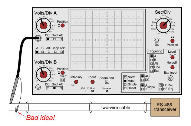
One solution to this problem is to use both probes of a dual-trace oscilloscope, and set it up for differential measurement. In this mode, only one waveform will be shown on the screen, even though two probes are being used. No ground clips need be connected to the circuit under test, and the waveform shown will be indicative of the voltage between the two probe tips.
