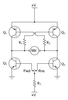
At any given moment, how many transistors are turned on and how many are turned off? Also, explain what would happen to the function of the circuit if resistor R1 failed open.  $\frac{\text{file }00449}{\text{circuit}}$
