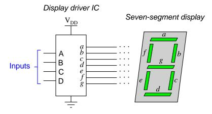
The behavior of the display driver IC may be represented by a truth table with seven outputs: one for each segment of the seven-segment display (a through g). In the following table, a "1" output represents an active display segment, while a "0" output represents an inactive segment:
