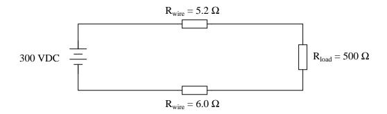
Also, calculate the amount of power that would be delivered to the load resistor if the wires were superconducting  $(R_{wire} = 0.0 \,\Omega)$ .
