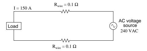
Calculate the load voltage, load power dissipation, the power dissipated by the wire resistance  $(R_{wire})$ , and the overall power efficiency, indicated by the Greek letter "eta"  $(\eta = \frac{P_{load}}{P_{source}})$ .
