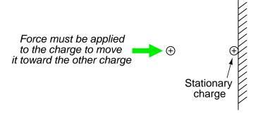
This mechanical work becomes "stored" in the electric field between the charges, and is a form of *potential energy*. This, again, is similar to a mechanical spring, where the work done in compressing a spring is "stored" as potential energy in its compressed state.
