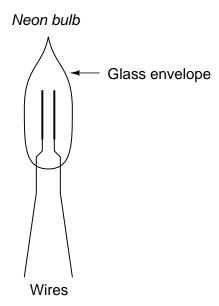
When a large enough static electric charge is applied between the two wires of the neon bulb, the neon gas inside will "ionize" and produce a colored flash of light. Experiment with generating your own static electricity and then making the bulb flash. Hint: it may be easier to see the bulb's flash if the room is dark.
