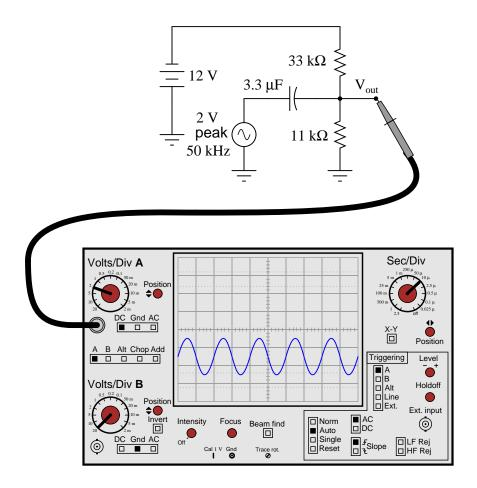
Follow-up question: explain why it is acceptable to use a polarized (polarity-sensitive) capacitor in this circuit when it is clearly connected to a source of AC. Why is it not damaged by the AC voltage when used like this?
