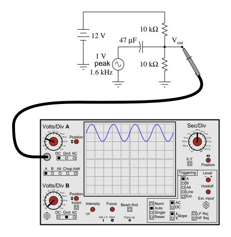
Follow-up question: what would the oscilloscope display look like if the coupling switch for channel A had been set to "AC" instead of "DC"?
