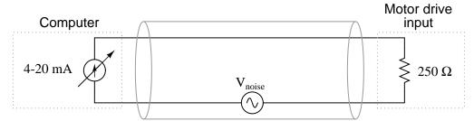
Use the superposition theorem to qualitatively determine which signal standard drops the greatest amount of noise voltage across the motor drive input's resistance, thereby most affecting the motor speed control.
