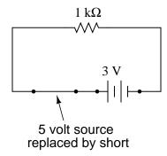
Now, suppose we were to remove the other voltage source from the circuit, replacing it with its internal resistance (0  $\Omega$ ). Re-calculate the resistor's voltage drop and current in the resulting circuit:
