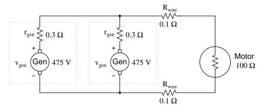
Use the Superposition Theorem to re-calculate the motor current and motor terminal voltage, commenting on how these figures compare with the first calculation (using only one generator).
