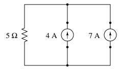
Calculate the resistor's voltage drop and current in this circuit.
