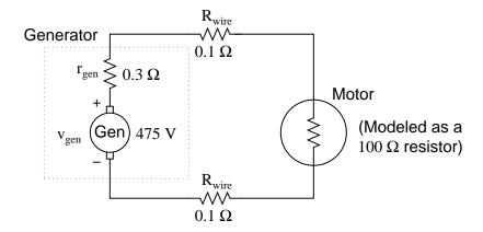
Calculate the amount of current this generator will supply to the motor and the voltage measured across the motor's terminals, taking into account all the resistances shown (generator internal resistance  $r_{gen}$ , wiring resistances  $R_{wire}$ , and the motor's equivalent resistance).
