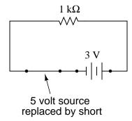
Now, suppose we were to remove the other voltage source from the circuit, replacing it with its internal resistance (0  $\Omega$ ). Re-calculate the resistor's voltage drop and current in the resulting circuit:
