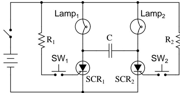
When the power is first turned on, neither lamp will energize. If either pushbutton switch is then momentarily actuated, the lamp controlled by that SCR will energize. If, after one of the lamps has been energized, the *other* pushbutton switch is then actuated, its lamp will energize *and the other lamp will de-energize*.
