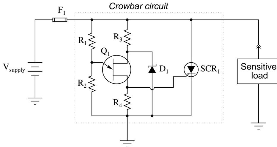
Measuring the supply voltage with a voltmeter, everything checks out well. There does not appear to be an overvoltage condition causing a legitimate "crowbar" event in the circuit. Disconnecting the load from the crowbar circuit and powering it up with a standard bench-top laboratory power supply reveals the load to be in perfect condition. Thus, both the source and the load have been eliminated as possibilities that may have blown the fuse(s).
