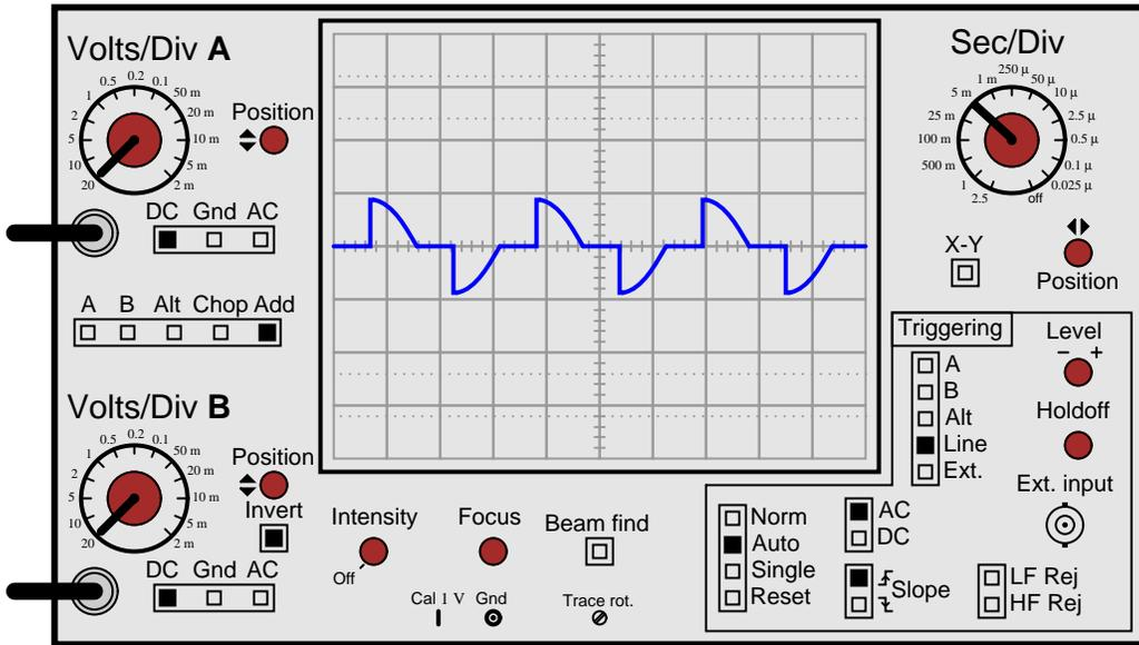
Explain why this circuit cannot provide continuous adjustment of light bulb brightness below this level.
