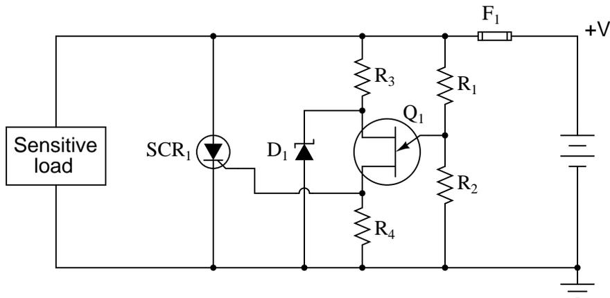
Here, the UJT serves as an overvoltage detection device, triggering the SCR when necessary. Explain how this circuit works, and what the function of each of its components is.
