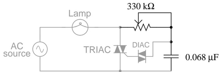
Calculate how many degrees of phase shift the capacitor's voltage is, compared to the total voltage across the series RC network, assuming a frequency of 60 Hz, and a 50% potentiometer setting.
