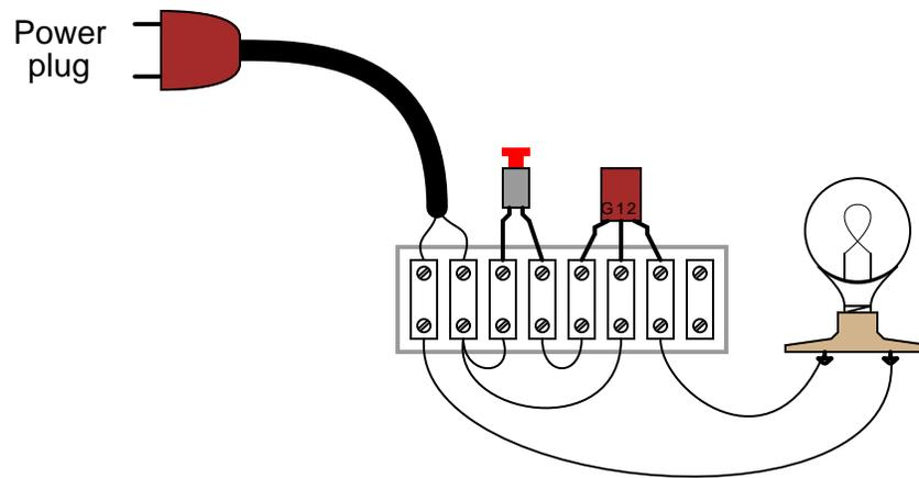
When the pushbutton switch is actuated, nothing happens. What is wrong with this circuit? Hint: the problem in this circuit is very subtle, and may be very difficult to discern.
