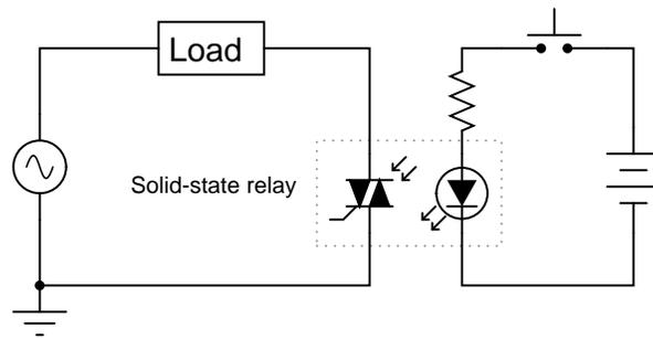
Describe some of the advantages of using a solid-state relay for switching AC power instead of using an electromechanical relay as shown here:
