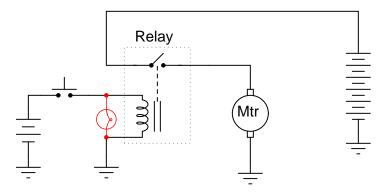
Instead of that stored energy manifesting itself as a high-voltage arc at the switch, it powers the light bulb for a brief time after the switch opens, dissipating in a non-destructive manner.
