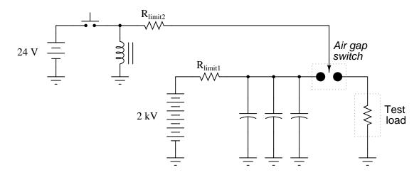
Suppose this surge power supply circuit failed to work after several months of good service. Nothing happens any more when the pushbutton switch is pressed and released. No spark is heard or seen in the air gap, and the test load receives no surge of current.
