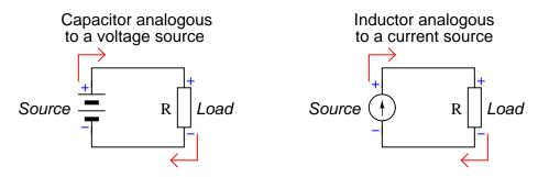
Large R values slow down RC circuits and speed up LR circuits, while small R values speed up RC circuits and slow down LR circuits.
