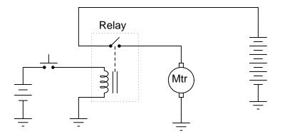
The problem here is every time the pushbutton switch is released, the contacts arc significantly. This happens because the inductor releases all of its stored energy as a high-voltage spark across the opening contacts. *Inductive kickback* is the phrase commonly used to describe this effect, and over time it will prematurely destroy the switch.
