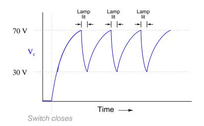
Follow-up question: assuming a source voltage of 100 volts, a resistor value of 27 k $\Omega$ , and a capacitor value of 22  $\mu$ F, calculate the amount of time it takes for the capacitor to charge from 30 volts to 70 volts (assuming the neon bulb draws negligible current during the charging phase).
