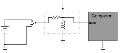
This circuit would certainly work to create brief pulses of voltage to the computer input, but it would also likely *destroy* the computer's input circuitry after a few switch actuations! Explain why.
