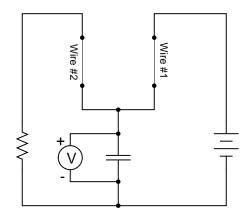
In order for this circuit to function properly as an intervalometer, which wire does the projectile need to break first? Explain why. Also, the voltmeter used in this instrument must be one with as high an input resistance as possible for best accuracy. Explain why this is necessary as well.
