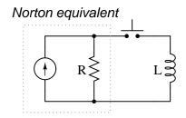
Re-analyze the circuit in this form, and try to explain why more resistance makes the inductor charging time faster and less resistance makes the inductor charging time slower. file 03533
