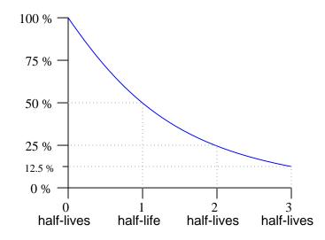
In RC and LR circuits, decay time is expressed in a slightly different way. Instead of measuring decay rate in units of *half-lives*, we measure decay rate in units of *time constants*, symbolized by the Greek letter "tau" ( $\tau$ ).
