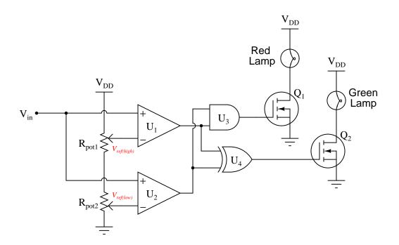
A technician decides to replace the red lamp, thinking it is burned out. This, unfortunately, does not fix the problem. Identify two possible component faults that could account for this problem, and describe what further diagnostic steps you would take to determine the precise nature of the fault. file 03839
