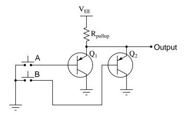
Be sure to explain why the proposed faults would cause the output to fail low.  $\underline{file}\ 03830$
