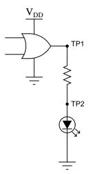
Now, obviously the output of the gate is "high" when the LED is on, otherwise it would not receive enough voltage to illuminate. Why then does a logic probe fail to indicate a high logic state at TP2? file 02866
