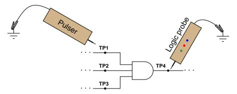
No matter which input test point (TP1, TP2, or TP3) she pulses, though, the output test point (TP4) always reads low. Does this prove the AND gate to be defective? Explain why or why not. file 03840
