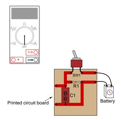
How would the multimeter be used to measure the voltage across the component labeled "R1" when energized? Include these important points in your answer:
