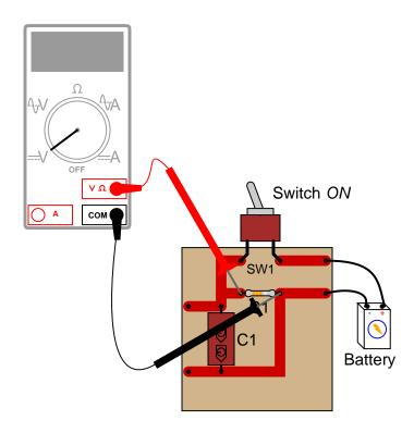
The test lead connections (to the circuit) shown are not the only correct answer. It is possible to touch the test leads to different points on the PCB and still measure the voltage across the resistor (component labeled R1). What are some alternative points on the PCB where the voltage across R1 could be measured?
