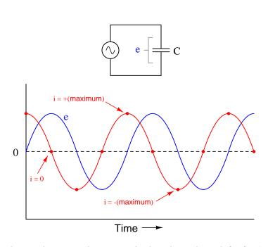
For a capacitor, voltage is lagging and current is leading, by a phase shift of  $90^{\circ}$ .
