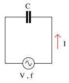
Write a single formula solving for capacitance given these three values (V, I, and f). file 02113
