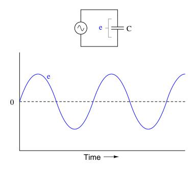
How much phase shift (in degrees) is there between the voltage and current waveforms? Which waveform is leading and which waveform is lagging?
