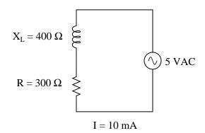
How many ohms of opposition does the series combination of resistor and inductor offer? What name do we give to this quantity, and how do we symbolize it, being that it is composed of both resistance (R) and reactance (X)?
