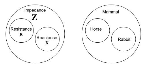
Resistance is a type of impedance, and so is reactance. The difference between the two has to do with *energy exchange*.
