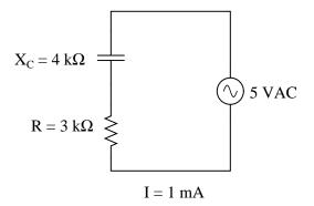
How many ohms of opposition does the series combination of resistor and capacitor offer? What name do we give to this quantity, and how do we symbolize it, being that it is composed of both resistance (R) and reactance (X)?
