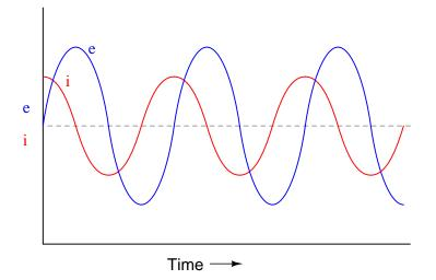
Given that power is the product of voltage and current (p = ie), plot the waveform for power in this circuit. Also, explain how the mnemonic phrase "*ELI the ICE man*" applies to these waveforms. file 00633
