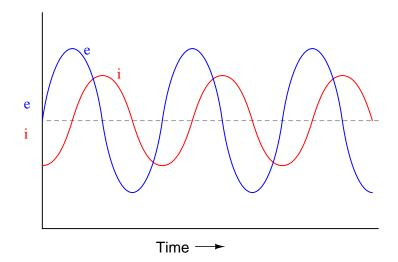
Given that power is the product of voltage and current (p = ie), plot the waveform for power in this circuit. Also, explain how the mnemonic phrase "ELI the ICE man" applies to these waveforms. file 00632
