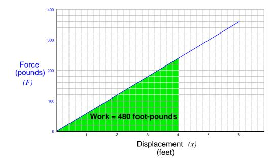
Note how the geometric interpretation of the shaded area on the graph exactly equals the result predicted by the equation  $E_p = \frac{1}{2}kx^2$ : the area of a triangle is one-half times the base times the height. One-half times 4 feet times 240 pounds is 480 foot-pounds.
