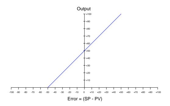
In this graph the bias value is 50% and the gain of the controller is 1.
