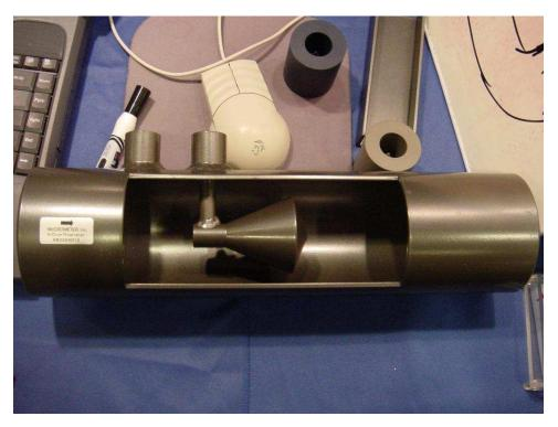
Segmental wedge elements are special pipe sections with wedge-shaped restrictions built in. These devices, albeit crude, are useful for measuring the flow rates of *slurries*, especially when pressure is sensed by the transmitter through remote-seal diaphragms (to eliminate the possibility of impulse tube plugging):
