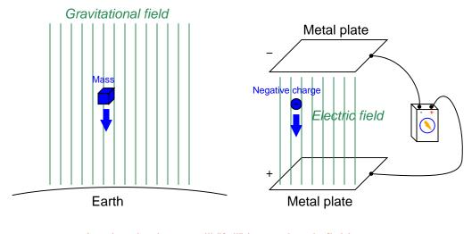
An electric charge will "fall" in an electric field just as a mass will fall in a gravitational field.
