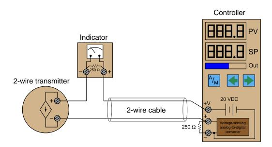
The indicator contains its own 250 ohm resistor to provide a 1-5 volt signal for the meter mechanism to sense. This means the total loop resistance is now 500 ohms (plus any wire resistance). At full current (20 mA), this total resistance will drop (at least) 10 volts, leaving 10 volts or less
