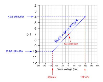
Most modern pH instruments will display the calculated slope value after calibration. This value should (ideally) be 59.17 millivolts per pH unit at 25 degrees Celsius, but it will likely be a bit less than this. The voltage-generating ability of a glass electrode decays with age, so a low slope value may indicate a probe in need of replacement.
