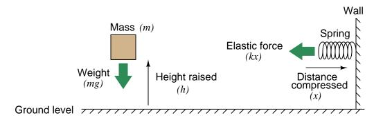
In either case, potential energy is calculated by the work done in exerting a force over a parallel distance. In the case of the weight, potential energy  $(E_p)$  is the simple product of weight (gravity g acting on the mass m) and height (h):
