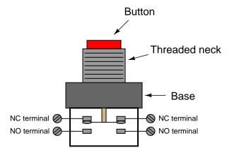
The threaded neck inserts through a hole cut into a metal or plastic panel, with a matching nut to hold it in place. Thus, the button faces the human operator(s) while the switch contacts reside on the other side of the panel.
