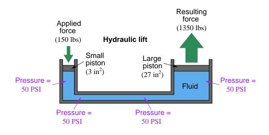
The key assumption we make here is that the only force we need to consider on the fluid is the force exerted on the small piston (150 pounds). If this is truly the only force acting on the fluid, then it will likewise be the only source of fluid pressure, and pressure will simply be equal to force divided by area (150 pounds  $\div$  3 square inches = 50 PSI).
