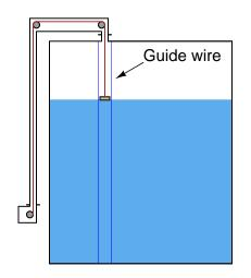
The guide wires are anchored to the floor and roof of the vessel, passing through ring lugs on the float to keep it from straying laterally.
