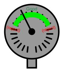
This is another example of the *analogue* nature of pneumatic pressure signals: the pressure registered by this gauge *represents* a completely different variable, in this case the mechanical fit of the shaft to the test jig.
