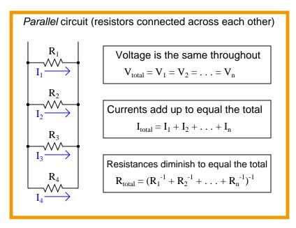
The rule for calculating total resistance in a parallel circuit perplexes many students with its weird compound reciprocal notation. There is a more intuitive way to understand this rule, and it involves a different quantity called *conductance*, symbolized by the letter G.
