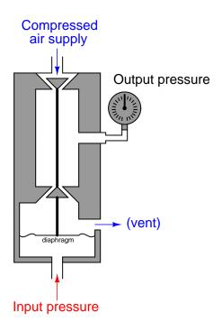
The diaphragm is nothing more than a thin disk of sheet metal, upon which an incoming air pressure signal presses. Force on the diaphragm is a simple function of signal pressure (P) and diaphragm area (A), as described by the standard force-pressure-area equation:
