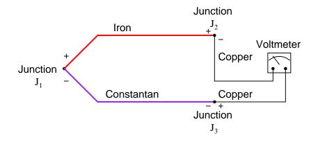
Here we have three voltage-generating junctions:  $J_1$  of iron and constantan,  $J_2$  of iron and copper, and  $J_3$  of copper and constantan which just happens to be the metallic combination for a type T thermocouple. Upon first inspection it would seem we have a much more complex situation than we did with just two metals (iron and copper), but in actuality the situation is as simple as before.
