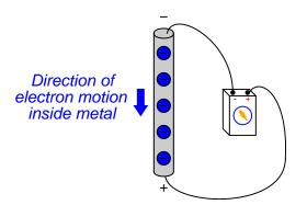
If the source of this voltage is continually replenished by chemical energy, mechanical energy, or some other form of energy, the free electrons will continually loop around this circular path. We call this unbroken path an *electric circuit*.
