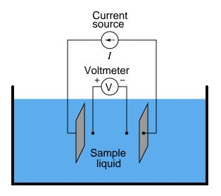
In the 4-wire conductivity cell, any electrode plating will merely burden the current source by causing it to output a greater voltage, but it will *not* affect the amount of voltage detected by the two inner electrodes as that electric current passes through the liquid. Some conductivity instruments employ a second voltmeter to measure the voltage dropped between the "excitation" electrodes, to indicate electrode fouling:
