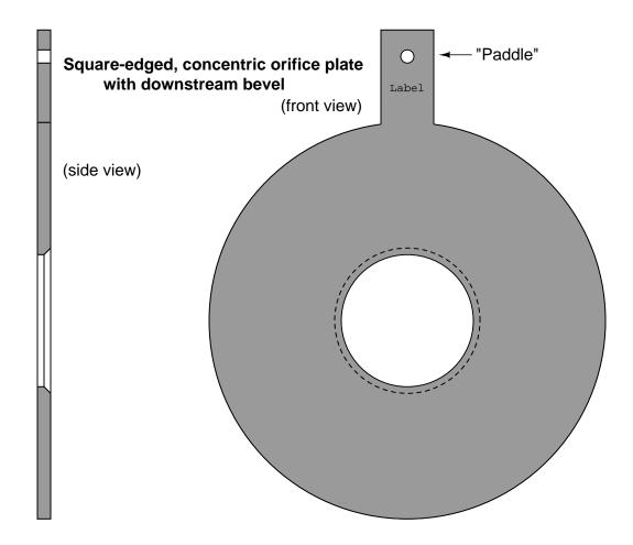
Looking at the side-view of this orifice plate, the intended direction of flow is left-to-right, with the sharp edge facing the incoming fluid stream and the bevel providing a non-contact outlet for the fluid. Beveled orifice plates are obviously uni-directional, and *must* be installed with the paddle text facing upstream.
