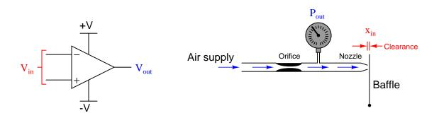
For each system there is an input and an output. For the opamp, input and output are both electrical (voltage) signals:  $V_{in}$  is the differential voltage between the two input terminals, and  $V_{out}$  is the single-ended voltage measured between the output terminal and ground. For the baffle/nozzle, the input is the physical gap between the baffle and nozzle  $(x_{in})$  while the output is the backpressure indicated by the pressure gauge  $(P_{out})$ .
