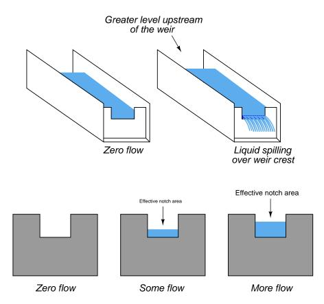
This dependence of notch area on flow rate creates a very different relationship between flow rate and liquid height (measured above the crest) than the relationship between flow rate and differential pressure in an orifice plate:
