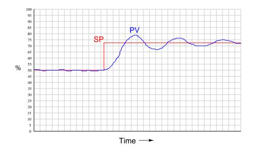
If the gain is set too low, the process response will be stable under steady-state conditions, but "sluggish" to changes in setpoint because the controller does not take aggressive enough action to cause quick changes in the process:
