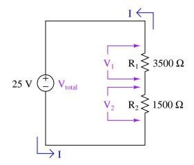
Note: arrows point in the direction of electron motion
