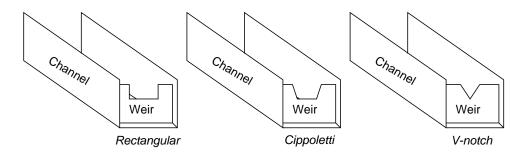
A rectangular weir has a notch of simple rectangular shape, as the name implies. A Cippoletti weir is much like a rectangular weir, except that the vertical sides of the notch have a 4:1 slope (rise of 4, run of 1; approximately a 14 degree angle from vertical). A V-notch weir has a triangular notch, customarily measuring either 60 or 90 degrees.
