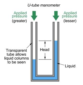
Liquid column height in a manometer should always be interpreted at the centerline of the liquid column, regardless of the shape of the liquid's meniscus (the curved air/liquid interface):
