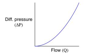
To obtain a linear flow measurement signal from the differential pressure instrument's output signal, we must "square root" that signal, either with a computer inside the transmitter, with a computer inside the receiving instrument, or a separate computing instrument (a "square root extractor"). We may see mathematically how this yields a value for flow rate (Q), following from our original equation:
