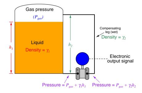
$$(P_{gas} + \gamma_1 h_1) - (P_{gas} + \gamma_2 h_2) = \gamma_1 h_1 - \gamma_2 h_2$$
