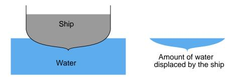
If we could somehow measure the weight of that water displaced, we would find it exactly equals the dry weight of the ship:
