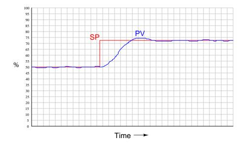
As with on/off control, instances of overshoot (the process variable rising above setpoint) and undershoot (drifting below setpoint) are generally undesirable, and for the same reasons. Ideally, the controller will be able to respond in such a way that the process variable is made equal to setpoint as quickly as the process dynamics will allow, yet with no substantial overshoot or undershoot. With plain proportional control, however, this ideal goal is nearly impossible.
