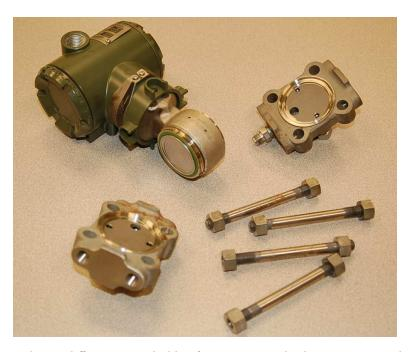
The important design differences are hidden from view, inside the sensing capsule. Functionally, though, this transmitter is much the same as its differential-capacitance cousin.
