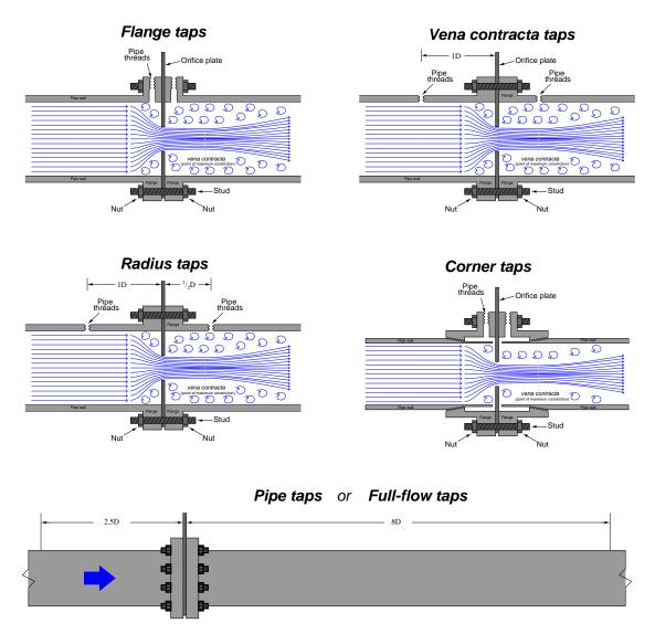
Flange taps are the most popular tap location in the United States. Flanges may be manufactured with tap holes pre-drilled and finished before the flange is even welded to the pipe, making this a very convenient pressure tap configuration. Most of the other tap configurations require drilling into the pipe after installation, which is not only labor-intensive, but may possibly weaken the pipe at the locations of the tap holes.
