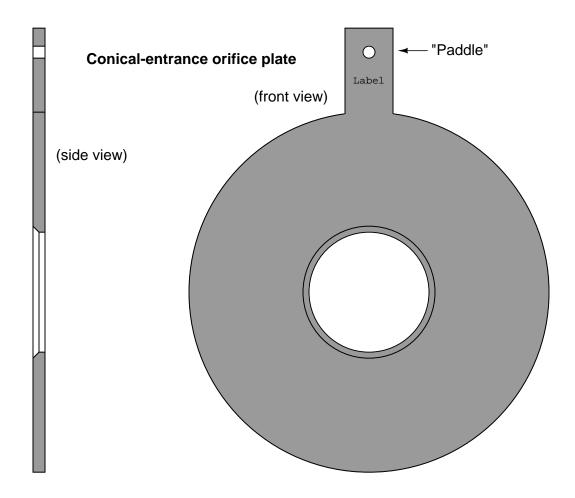
Here, is it vitally important to pay attention to the paddle's text label. This is the only sure indication of which direction an orifice plate needs to be installed. One can easily imagine an instrument technician mistaking a conical-entrance orifice plate for a square-edged, beveled orifice plate and installing it backward!
