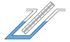
This way, a greater motion of liquid is required to generate the same hydrostatic pressure (vertical liquid displacement) than in an upright manometer, making the inclined manometer more sensitive.
