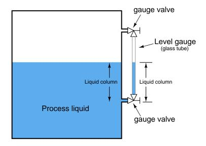
Level gauge values exist to allow replacement of the glass tube without emptying or depressurizing the process vessel. These values are usually equipped with flow-limiting devices in the event of a tube rupture, so that too much process fluid does not escape even when the values are fully open.
