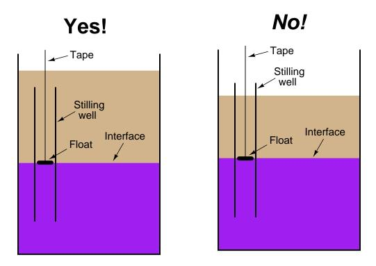
In the left-hand installation where the stilling well is completely submerged, the interface levels will always match. In the right-hand installation where the top of the stilling well extends above the total liquid level, however, the two levels may not always match:
