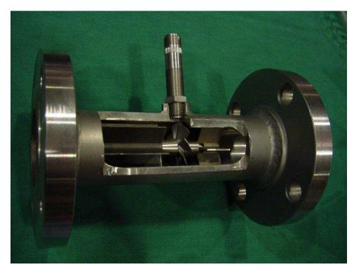
Note the sets of "flow conditioner" vanes immediately before and after the turbine wheel in the photograph. As one might expect, turbine flowmeters are very sensitive to *swirl* in the process fluid flowstream. In order to achieve high accuracy, the flow profile must not be swirling in the vicinity of the turbine, lest the turbine wheel spin faster or slower than it should to represent the velocity of a straight-flowing fluid.
