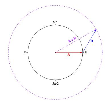
The length of the dashed-line vector  $\mathbf{A} + \mathbf{B}$  (radius of the dashed-line circle) represents the amplitude of the resultant sum waveform, while the phase shift is represented by the angles between
