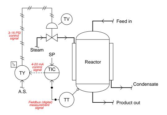
The purpose of this control system is to ensure the chemical solution inside the reactor vessel is maintained at a constant temperature. A steam-heated "jacket" envelops the reactor vessel, transferring heat from the steam into the chemical solution inside. The control system maintains a constant temperature by measuring the temperature of the reactor vessel, and throttling steam from a boiler to the steam jacket to add more or less heat as needed.
