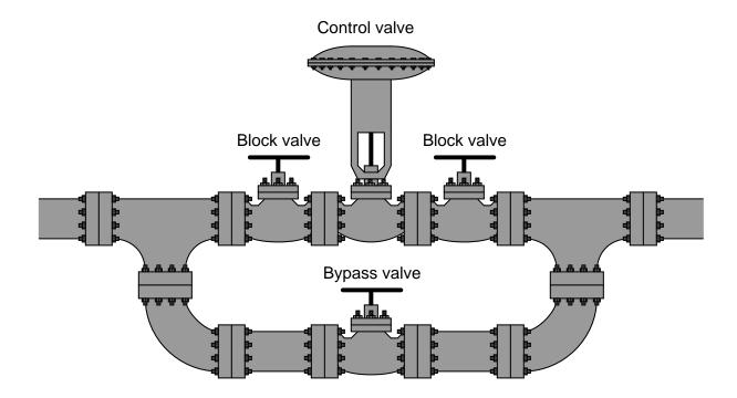
Since the manually-operated bypass valve now performs the job that the automatic control valve used to, a human operator must remain posted at the bypass valve to carefully throttle it and maintain control of the process.
