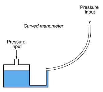
The scale positioned alongside the curved viewing tube will be linear, with equal spacings between division marks along its entire length. The vertical height of the liquid column translates pressure into varying degrees of movement along the axis of the tube by the tube's curvature. Literally, any inverse function desired may be "encoded" into this manometer by fashioning the viewing tube into the desired (custom) shape without any need to print a nonlinear scale.
