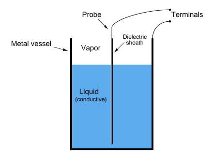
In this style of capacitive level probe, the variable is distance (d), since the conductive liquid essentially acts to bring the vessel wall electrically closer to the probe. This means total capacitance
