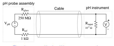
Equivalent electrical circuit of a pH probe and instrument
