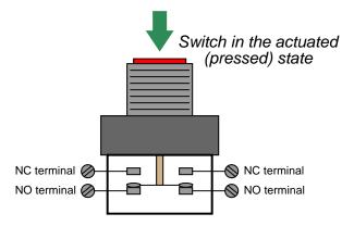
The schematic diagram symbol for this type of switch looks much like the real thing, with the normally-closed contact set on top and the normally-open contact set below:
