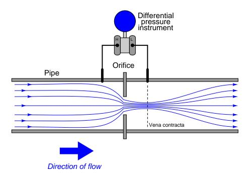
Now, the really weird thing about measuring flow this way is that the resulting  $\Delta P$  signal does not linearly correspond to flow rate. Double the flow rate, and the  $\Delta P$  quadruples. Triple the flow rate and the  $\Delta P$  increases by a factor of nine. To express this relationship mathematically:
