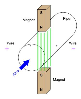
The direction of liquid flow cuts perpendicularly through the lines of magnetic flux, generating a voltage along an axis perpendicular to both. Metal electrodes opposite each other in the pipe wall intercept this voltage, making it readable to an electronic circuit.
