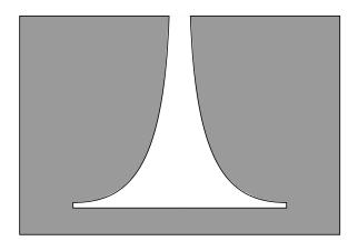
This weir design is not used very often, due to its inherently weak structure and tendency to clog with debris.
