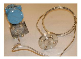
A close-up view of the sealing diaphragm shows its corrugated design, allowing the metal to easily flex and transfer pressure to the fill fluid within the capillary tubing:
