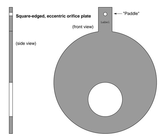
For gas flows, the hole should be offset downward, so that any liquid droplets or solid particles may easily pass through. For liquid flows, the hole should be offset upward to allow gas bubbles to pass through and offset downward to allow heavy solids to pass through.
