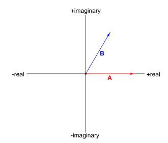
If we do this, we may symbolically represent each vector as a complex number. For example, vector **B** in the above diagram could be represented as the complex number x + jy (using j as the symbol for an imaginary quantity instead of i so as to not confuse it with *current*):
