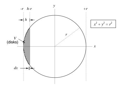
If  $x^2 + y^2 = r^2$  (the mathematical definition of a circle), then the volume of each circular disk comprising the accumulated volume between -r and h - r is equal to  $\pi y^2 dx$ . In other words, the total accumulated area between -r and h - r is:
