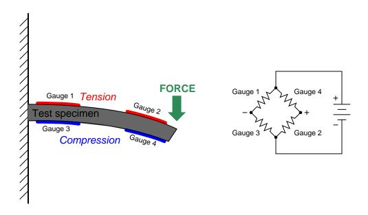
Not only does a full-active bridge circuit provide greater sensitivity and linearity than a quarteractive bridge, but it also *naturally* provides temperature compensation without the need for "dummy" strain gauges, since the resistances of all four strain gauges will change by the same proportion if the specimen temperature changes.
