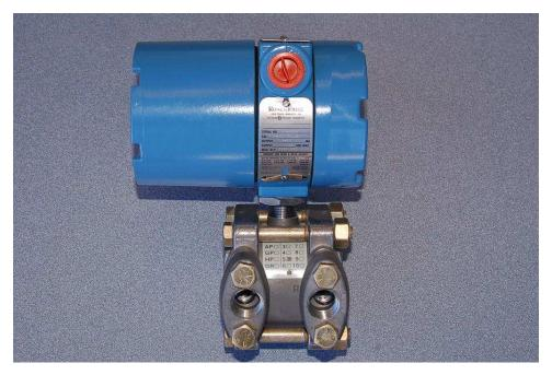
By removing four bolts from the transmitter, we are able to remove two flanges from the pressure capsule, exposing the isolating diaphragms to plain view:
