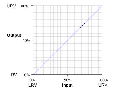
This graph shows how any given percentage of input should correspond to the same percentage of output, all the way from 0% to 100%.
