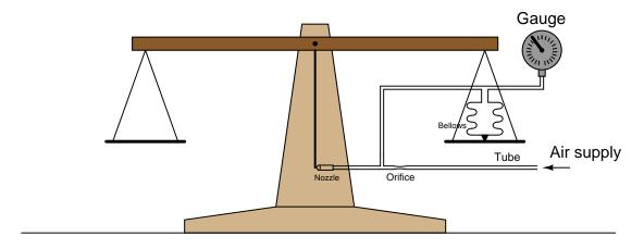
Although it may seem as though we are done with the task of fully automating the laboratory scale, we can go a step further. Building this pneumatic negative-feedback balancing system provides us with a capability the old manually-operated scale never had: *remote indication*. There is no reason why the indicating gauge must be located near the scale. Nothing prevents us from locating the receiver gauge some distance from the scale, and using long lengths of tubing to connect the two:
