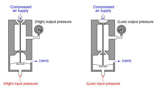
Since there is a direct relationship between input pressure and output pressure in this pneumatic relay, we classify it as a *direct-acting relay*. If we were to add an actuating diaphragm to the first pilot valve design, we would have a *reverse-acting relay* as shown here:
