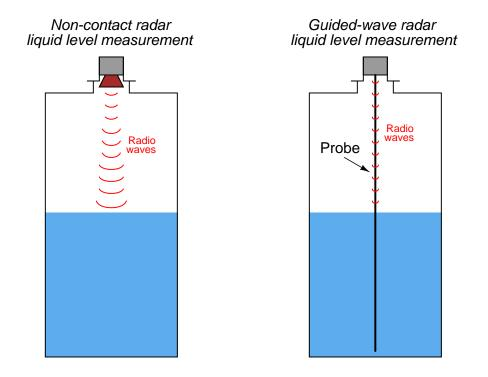
Non-contact radar transmitters are always mounted on the top side of a storage vessel. Modern radar transmitters are quite compact, as this photograph shows:
