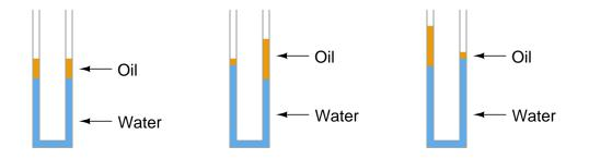
The only way to ensure proper two-part liquid interface level indication in a sightglass is to keep both ports (nozzles) submerged:
