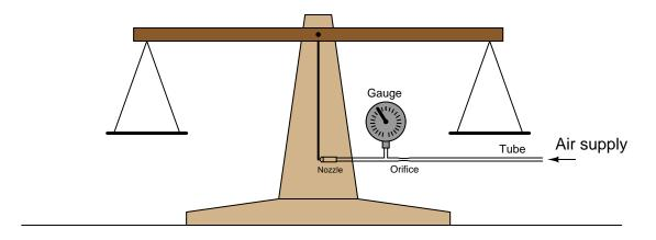
Now we have a highly sensitive means of indicating when the scale is balanced, but we still have not yet achieved full automation. The scale cannot balance itself, at least not yet.
