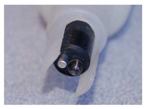
It is extremely important to always keep the glass electrode wet. Its proper operation depends on complete *hydration* of the glass, which allows hydrogen ions to penetrate the glass and develop the Nernst potential. The probes shown in these photographs are shown in a dry state only because they have already exhausted their useful lives and cannot be damaged any further by dehydration.
