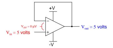
If we simply assume there will be no difference of voltage between the two input terminals of the opamp with negative feedback in effect, we may conclude that the output voltage is exactly equal to the input voltage, since that is what *must* happen in order for the two input terminals to see equal potentials.
