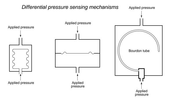
The challenge in doing this, of course, is how to extract the mechanical motion of the pressuresensing element to an external mechanism (such as a pointer) while maintaining a good pressure seal. In gauge pressure mechanisms, this is no problem because one side of the pressure-sensing element must be exposed to atmospheric pressure anyway, and so that side is always available for mechanical connection.
