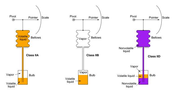
Given that the liquid and vapor are in direct contact with each other, the pressure in the system will be precisely equal to the *saturated vapor pressure* at the vapor/liquid interface. This makes the Class II system sensitive to temperature only at the bulb and nowhere else along the system's volume. Because of this phenomenon, a Class II filled-bulb system requires no compensation for temperature changes at the indicator.
