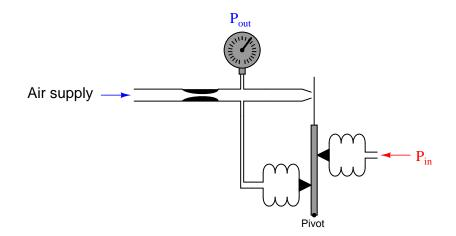
This arrangement effectively reduces the feedback force by placing the feedback bellows at a mechanical disadvantage to the input bellows. If the distance between the feedback bellows tip and the force beam pivot is exactly half the distance between the input bellows tip and the force beam pivot, the effective force ratio will be one-half.
