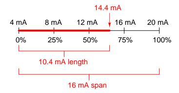
As a percentage, this thick line is 10.4 mA long (the distance between 14.4 mA and 4 mA) over a total (possible) length of 16 mA (the total span between 20 mA and 4 mA). Thus:
