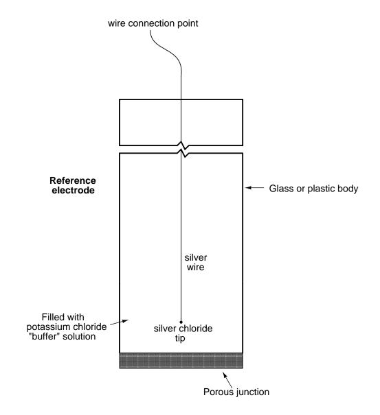
Together, the measurement and reference electrodes provide a voltage-generating element sensitive to the pH value of whatever solution they are submerged in:
