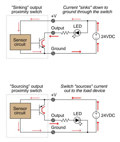
These terms simply make no sense when viewed from the perspective of electron flow notation. If you were to actually trace the directions of the electrons, you would find that a device "sourcing" current has electrons flowing *into* its connection terminal, while a device "sinking" current sends electrons *out* to another device where they travel (up) to a point of more positive potential.
