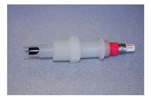
A close-up photograph of the probe tip reveals the glass measurement bulb, a weep hole for process liquid to enter the reference electrode assembly (internal to the white plastic probe body), and a metal *solution ground* electrode:
