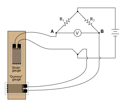
The "dummy" gauge is attached to the specimen in such a way that it maintains the same temperature as the active strain gauge, yet experiences no strain. Thus, any *difference* in gauge resistances must be due solely to specimen strain. The differential nature of the bridge circuit naturally translates the differential resistance of the two gauges into one voltage signal representing strain.
