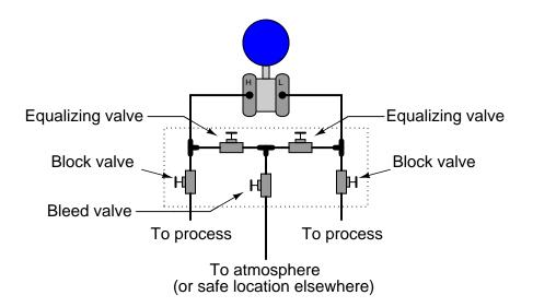
Manifold valve positions for normal operation and maintenance are as follows:
