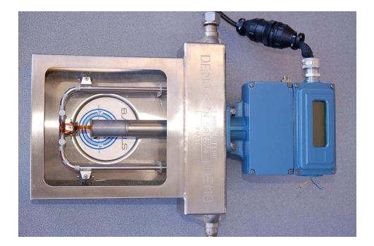
A closer inspection of this flowmeter shows that there are actually two U-tubes, one positioned directly above the other, shaken in complementary directions by a common electromagnetic force coil:
