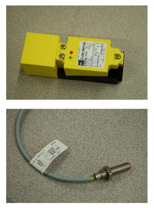
This switch detects the passing of teeth on the chain sprocket, generating a slow square-wave electrical signal as the sprocket rotates. Such a switch may be used as a rotational speed sensor
