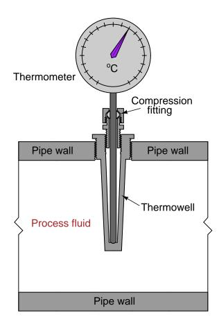
If the temperature gauge is removed for service or replacement, the thermowell maintains pressure integrity of the pipe (no process fluid leaking out, and no air leaking in):
