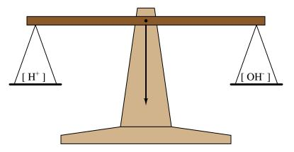
When the solution is pure water, this imaginary scale is balanced (neutral), with  $[H^+] = [OH^-]$ . Adding an acid to the solution tips the scale one way, while adding a caustic to the solution tips it the other way<sup>3</sup>.
