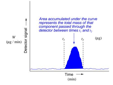
Since process chromatographs have the ability to independently analyze the quantities of multiple components in a chemical sample, these instruments are inherently *multi-variable*. A single analog
