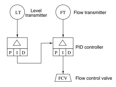
In this case, the primary controller senses the level in a vessel, commanding the secondary (flow) controller to maintain the necessary amount of flow either in or out of the vessel as needed to maintain level at some setpoint.
