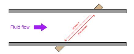
In this flowmeter design, a clean fluid with no solid impurities is essential for good signal transmission.
