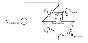
Fixed resistors  $R_1$  and  $R_2$  are of precisely known value and high precision. Variable resistor  $R_{adjust}$  has a labeled knob allowing for a person to adjust and read its value to a high degree of precision. When the ratio of the variable resistance to the specimen resistance equals the ratio of the two fixed resistors, the sensitive galvanometer will register exactly zero volts regardless of the excitation source's value. This is called a *balanced* condition for the bridge circuit:
