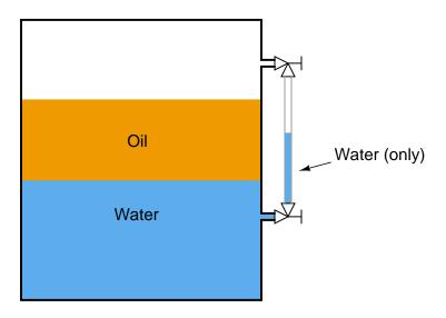
Here we see how a column of water in the sightglass shows less (total) level than the combination of water and oil inside the process vessel. Since the oil lies between the two level gauge ports into the vessel (sometimes called *nozzles*), it cannot enter the sightglass tube, and therefore the level gauge will continue to show just water.
