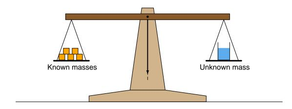
Here, the unknown mass is the sensed quantity, and the known masses are the adjustable quantity. A human lab technician applies as many masses to the left-hand side of the scale as needed to achieve balance, then counts up the sum total of those masses to determine the quantity of the unknown mass.
