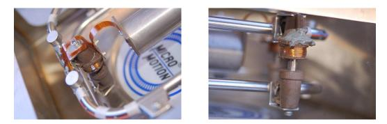
Advances in sensor technology and signal processing have allowed the construction of Coriolis flowmeters employing straighter tubes than the U-tube unit previously illustrated and photographed. Straighter tubes are advantageous for reasons of reduced plugging potential and the ability to easily drain all liquids out of the flowmeter when needed.
