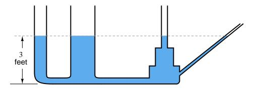
Since the force of fluid weight is generated only along the axis of gravitational attraction (straight down), that is the only axis of measurement important in determining "hydrostatic" fluid pressure.
