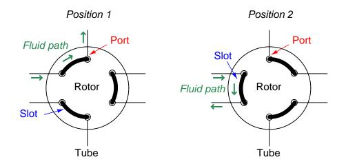
Three slots connect three pairs of ports together. When the rotary valve actuates, the port connections switch, redirecting gas flows.
