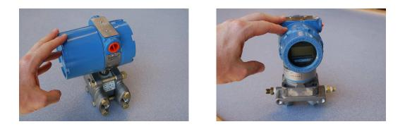
Two more models of electronic differential pressure transmitter are shown in the next photograph, the Yokogawa EJA110 (left) and the Foxboro IDP10 (right):
