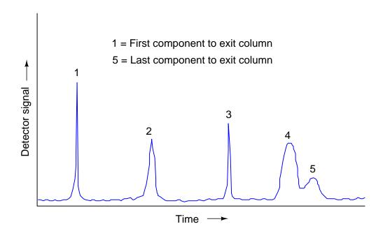
Narrow peaks represent compact bunches of molecules all exiting the column at nearly the same time. Wide peaks represent more diffuse groupings of similar (or identical) molecules. In this chromatogram, you can see that components 4 and 5 are not clearly differentiated over time. Better separation may be achieved by altering the sample volume, carrier gas flow rate, type of carrier gas, column packing material, and/or column temperature.
