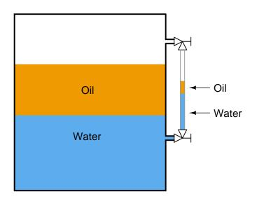
In effect, the level gauge and vessel together form a U-tube manometer. So long as the pressures from each liquid column are the same, the columns balance each other. The problem is, many different liquid-liquid interface columns can have the same hydrostatic pressure without being identical to one another:
