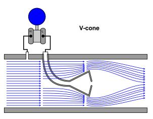
This cone is hollow, with a pressure-sensing port on the downstream side allowing for easy detection of fluid pressure near the vena contracta. Upstream pressure is sensed by another port in
