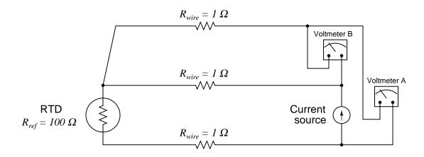
In a three-wire RTD circuit, voltmeter "A" measures the voltage dropped across the RTD (plus the voltage dropped across the bottom current-carrying wire). Voltmeter "B" measures just the voltage dropped across the top current-carrying wire. Assuming both current-carrying wires will have (very nearly) the same resistance, subtracting the indication of voltmeter "B" from the indication given by voltmeter "A" yields the voltage dropped across the RTD.
