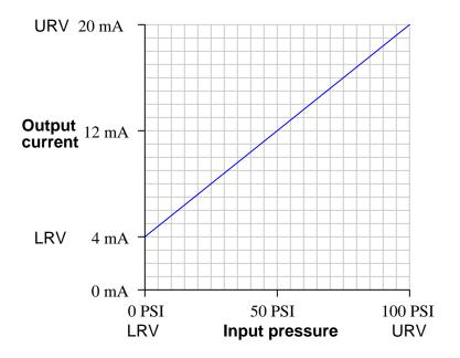
Although the graph is still linear, zero pressure does not equate to zero current. This is called a *live zero*, because the 0% point of measurement (0 PSI fluid pressure) corresponds to a non-zero ("live") electronic signal. 0 PSI pressure may be the LRV (Lower Range Value) of the transmitter's input, but the LRV of the transmitter's output is 4 mA, not 0 mA.
