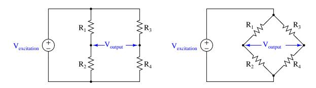
The voltage source powering the bridge circuit is called the *excitation* source. This source may be DC or AC depending on the application of the bridge circuit. The components comprising the bridge need not be resistors, either: capacitors, inductors, lengths of wire, sensing elements, and other component forms are possible, depending on the application.
