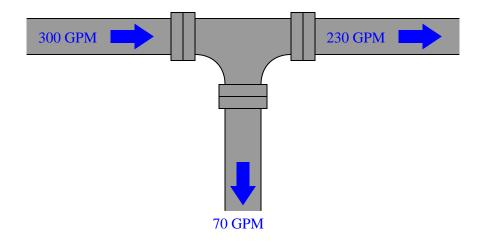
So long as there are no leaks in this piping system, every drop of water entering the tee must be balanced by a drop exiting the tee. For there to be a continuous mis-match between flow rates would imply a violation of the Law of Mass Conservation.
