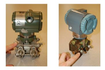
Regardless of make or model, every differential pressure ("DP", "d/p", or  $\Delta P$ )<sup>8</sup> transmitter has *two* pressure ports to sense different process fluid pressures. One of these ports is labeled "high" and the other is labeled "low". This labeling does not necessarily mean that the "high" port must always be at a greater pressure than the "low" port. What these labels represent is the effect that a pressure at that point will have on the output signal.
