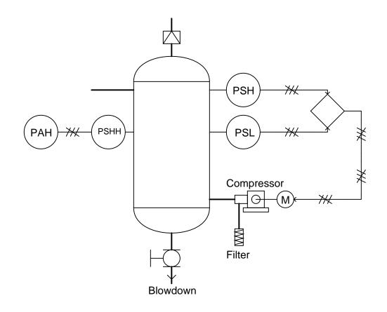
The "PSH" (*pressure switch, high*) activates when the air pressure inside the vessel reaches its high control point. The "PSL" (*pressure switch, low*) activates when the air pressure inside the vessel drops down to its low control point. Both switches feed discrete (on/off) electrical signals to a logic control device (signified by the diamond) which then controls the starting and stopping of the electric motor-driven air compressor.
