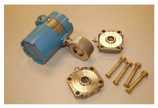
A close-up photograph shows the construction of one of the isolating diaphragms, which unlike
