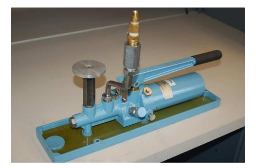
There is also such a thing as a *pneumatic* deadweight tester. In these devices, a constant flow of gas such as compressed air or bottled nitrogen vents through a bleed port operated by the primary piston. The piston moves as necessary to maintain just enough gas pressure inside the unit to suspend the mass(es) against gravity. This gas pressure passes on to the instrument under test, just as liquid pressure in a hydraulic deadweight tester passes to the test instrument for comparison:
