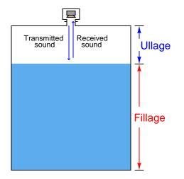
Ullage is the "natural" mode of measurement for this sort of level instrument, because the sound wave's time-of-flight is a direct function of how much empty space exists between the liquid surface and the top of the vessel. Total tank height will always be the sum of fillage and ullage, though. If the ultrasonic level transmitter is programmed with the vessel's total height, it may calculate fillage via simple subtraction:
