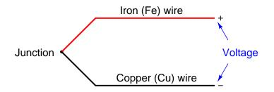
This phenomenon provides us with a simple and direct way to electrically infer temperature: simply measure the voltage produced by the junction, and you can tell the temperature of that junction. And it would be that simple, if it were not for an unavoidable consequence of electric circuits: when we connect any kind of electrical instrument the iron and copper wires, we inevitably produce another junction of dissimilar metals. The following schematic shows this fact.
