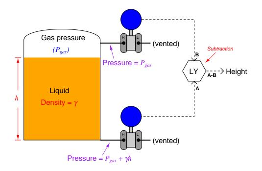
This approach enjoys the distinct advantage of avoiding a potentially wet compensating leg, but suffers the disadvantages of extra cost and greater error due to the potential calibration drift of two transmitters rather than just one. Such a system is also impractical in applications where the gas pressure is substantial compared to the hydrostatic (elevation head) pressure<sup>7</sup>.
