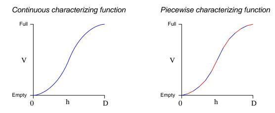
The computer correlates the input signal (height measurement, h) to a point on this piecewise function, linearly interpolating between the nearest pair of programmed coordinate points. The number of points available for multi-point characterizers varies between ten and one hundred<sup>2</sup> depending on the desired accuracy and the available computing power.
