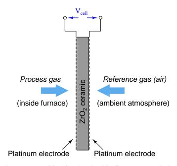
The electrical voltage generated by this "sandwich" of zirconium and platinum is sent to an electronic amplifier circuit, and then to a microcomputer which applies an inverse function to the measured voltage in order to arrive at an inferred measurement for oxygen concentration. This type of chemical analysis is called *potentiometric*, since it measures ("metric") based on an electrical voltage ("potential").
