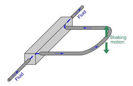
The two parallel tubes will experience opposite Coriolis forces as the U-tube assembly shakes up and down, causing the U-bend to twist. As mass flow rate through the tube increases, so does the degree of twisting. By monitoring the amplitude of this twisting motion, we may infer the mass flow rate of the fluid passing through the tube:
