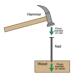
The impact of the hammer's blow is directed straight through the solid nail into the wood below. Nothing surprising here. But now consider what a fluid would do when subjected to the same hammer blow:
