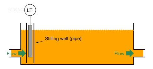
Stilling wells may be used in conjunction with many types of level instruments: floats, displacers, ultrasonic, radar, and laser to name a few. If the process application necessitates liquid-liquid interface measurement, however, the stilling well must be properly installed to ensure the interface level inside the well match the interface levels in the rest of the vessel. Consider this example of using a stilling well in conjunction with a tape-and-float system for interface measurement:
