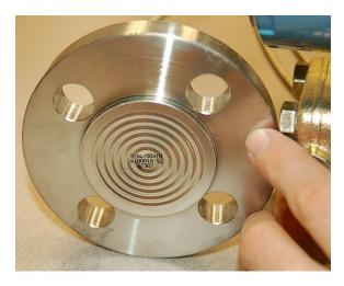
Just like the isolating diaphragms of the pressure-sensing capsule, these remote diaphragms need only transfer process fluid pressure to the fill fluid and (ultimately) to the taut sensing diaphragm inside the instrument. Therefore, these diaphragms perform their function best if they are designed to easily flex. This allows the taut sensing diaphragm to provide the vast majority of the opposing force to the fluid pressure, as though it were the only spring element in the fluid system.
