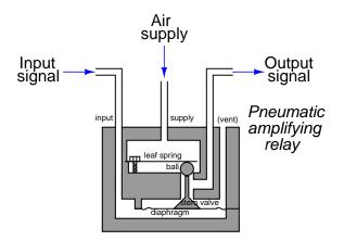
The motion of the diaphragm actuated a pair of valves: one with a cone-shaped plug and the other with a metal ball for a plug. The ball-plug allowed supply air to go to the output port, while the cone-shaped "stem valve" plug vented excess air pressure to the vent port.
