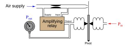
Thus, adding a relay to a self-balancing pneumatic system is analogous to increasing the openloop voltage gain of an opamp  $(A_{OL})$  by several-fold: it makes the overall gain *closer to ideal*. The overall gain of the system, though, is dictated by the ratio of bellows leverage on the force beam, just like the overall gain of a negative-feedback opamp circuit is dictated by the feedback network and *not* by the opamp's internal (open-loop) voltage gain.
