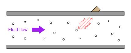
If the reflected wave returns from a bubble that is advancing toward the flowmeter sensor, the reflected frequency will be greater than the incident frequency. If the flow reverses direction and the reflected wave returns from a bubble that is traveling away from the sensor, the reflected frequency will be less than the incident frequency.
