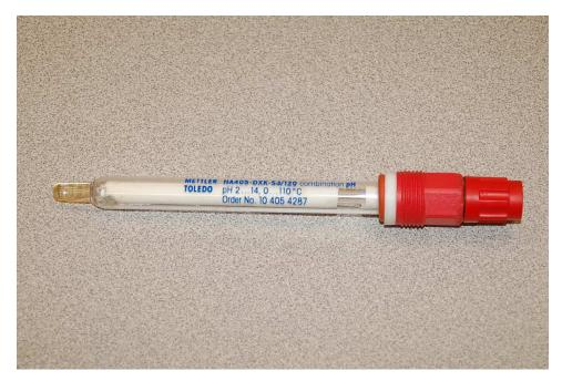
The red-colored plastic cap on the right-hand end of this combination electrode covers and protects a gold-plated coaxial electrical connector, to which the voltage-sensitive pH indicator (or transmitter) attaches.
