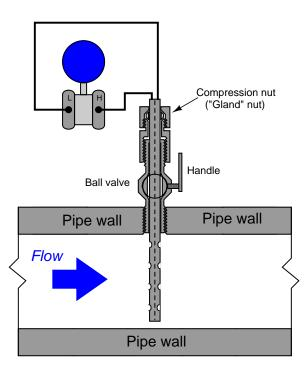
The Annubar element may be extracted from the pipe by loosening a "gland nut" and pulling the assembly out until the end passes through a hand ball valve. Once the element has been extracted this far, the ball valve may be shut and the Annubar completely removed from the pipe:
