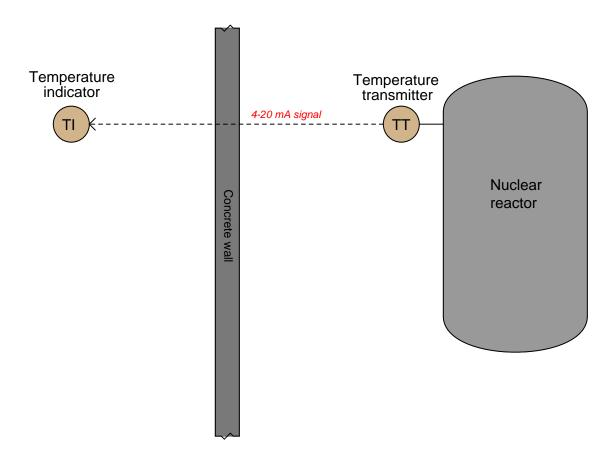
No human can survive inside the concrete-walled containment vessel when the nuclear reactor is operating, due to the strong radiation flux around the reactor. The temperature transmitter is built to withstand the radiation, though, and it transmits a 4 to 20 milliamp electronic signal to an
