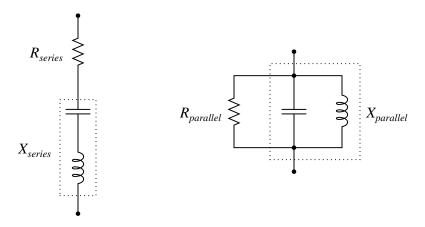
If the total impedance of one circuit (either series or parallel) is known, the component values of the equivalent circuit may be found by algebraically manipulating these equations and solving for the desired R and X values:
