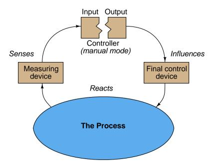
By making carefully measured changes in the controller's output and examining the consequent changes in transmitter signal, one may determine the existence of many different problems including transmitter and process noise, improper transmitter ranges, final control element hysteresis, variations in process gain, lag times, dead times, and other impediments to optimum control. Only after examining the process and its response to changes in valve position should controller tuning be attempted.
