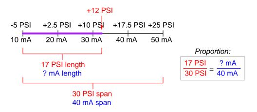
Finding the "length" of this line segment in units of milliamps is as simple as setting up a proportion between the length of the line in units of PSI over the total (span) in PSI, to the length of the line in units of mA over the total (span) in mA:
