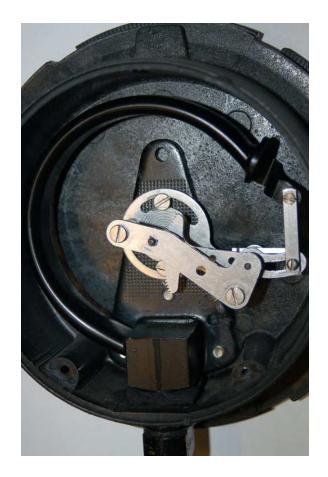
It should be noted that bellows, diaphragms, and bourdon tubes alike may all be used to measure differential and/or absolute pressure in addition to gauge pressure. All that is needed for these other functionalities is to subject the *other* side of each pressure-sensing element to either another applied pressure (in the case of differential measurement) or to a vacuum chamber (in the case of absolute pressure measurement):
