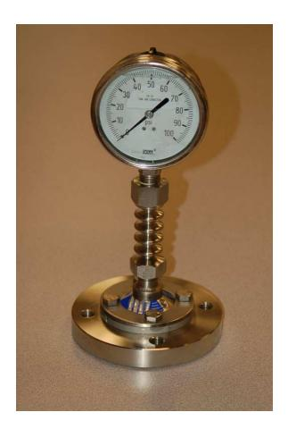
A view facing the bottom of the flange reveals the thin metal isolating diaphragm which keeps process fluid from entering the gauge mechanism. Only inert fill fluid occupies the space between this diaphragm and the gauge's bourdon tube:
