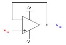
We call this "negative" or "degenerative" feedback because its effect is counteractive in nature. If the output voltage rises too high, the effect of feeding this signal to the inverting input will be to bring the output voltage back down again. Likewise, if the output voltage is too low, the inverting input will sense this and act to bring it back up again. *Self-correction* typifies the very nature of negative feedback.
