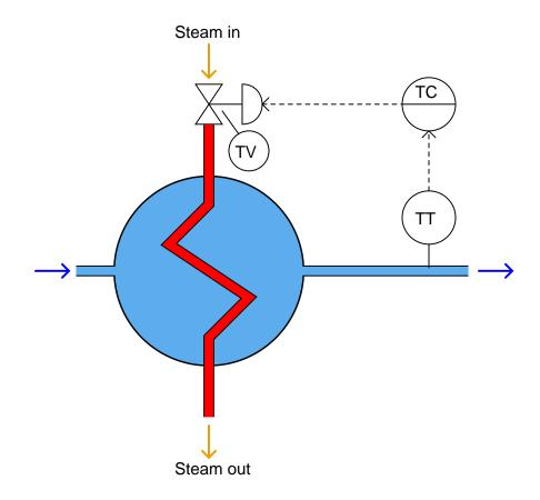
Here, the circle with the letters "TC" in the center represents the controller. Those letters stand for Temperature Controller, since the process variable being controlled is the process fluid's *temperature*. Usually, the controller consists of a computer making automatic decisions to open and close the valve as necessary to stabilize the process variable at some predetermined *setpoint*.
