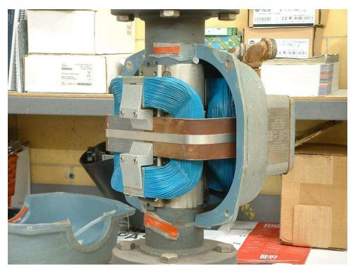
Perhaps the simplest form of coil excitation is when the coil is energized by 60 Hz AC power taken from the line power source. Since motional EMF is proportional to fluid velocity and to the flux density of the magnetic field, the induced voltage for such a coil will be a sine wave whose amplitude varies with volumetric flow rate.
