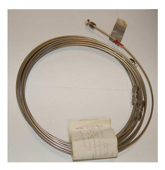
This particular GC column is 28 feet long, with an *outside* diameter of only 1/8 inch (the tube's inside diameter is even less than that). Column geometry and packing material vary greatly with application. The many choices intrinsic to column design are best left to specialists in the field of chromatography, not the average technician or even the average process engineer.
