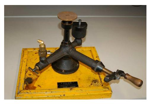
When sufficient pressure has been accumulated inside the tester to overcome the weight on the piston, the piston rises off its rest and "floats" on the pressurized oil, as shown in this close-up photograph:
