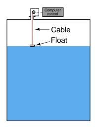
A simpler version of this technique uses a spring-reel to constantly tension the cable holding the float, so that the float continuously rides on the surface of the liquid in the vessel<sup>1</sup>:
