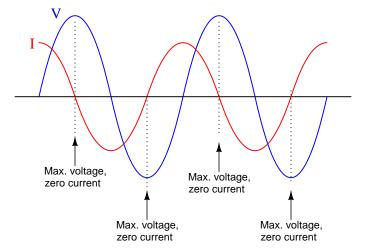
At these instantaneous points in time, it truly does appear as if the "resistance" of the capacitor is undefined (infinite), with multiple incidents of maximum voltage and zero current. However, this does not capture the essence of what we are trying to do: relate the *peak amplitude* of the voltage with the *peak amplitude* of the current, to see what the ratio of these two peaks are. The ratio calculated here utterly fails because those peaks never happen at the same time.
