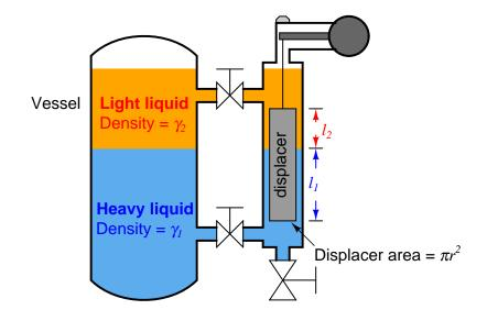
$$F_{buoyant} = \gamma_1 \pi r^2 l_1 + \gamma_2 \pi r^2 l_2$$
