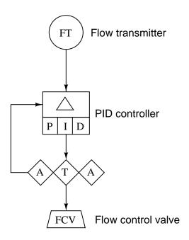
Rectangular blocks such as the  $\Delta$ , P, I, and D shown in this diagram represent automatic functions. Diamond-shaped blocks such as the A and T blocks are manual functions which must be set by a human operator. Showing even more detail, the following SAMA diagram indicates the presence of *setpoint tracking* in the controller algorithm, a feature that forces the setpoint value to equal the process variable value any time the controller is in manual mode:
