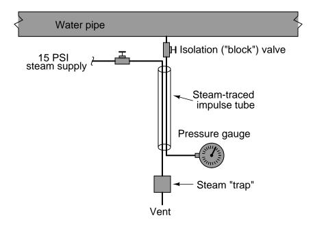
Steam flows through the shutoff valve, through the tube in the insulated bundle, transferring heat to the impulse tube as it flows past. Cooled steam condenses into water and collects in the *steam trap* device located at the lowest elevation on the steam trace line. When the water level builds up to a certain level inside the trap, a float-operated valve opens to vent the water. This allows more steam to flow into the tracing tube, keeping the impulse line continually heated.
