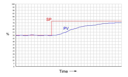
With proportional-only control, the only way to obtain fast-acting response to setpoint changes or "upsets" in the process is to set the gain constant high enough that some "overshoot" results:
