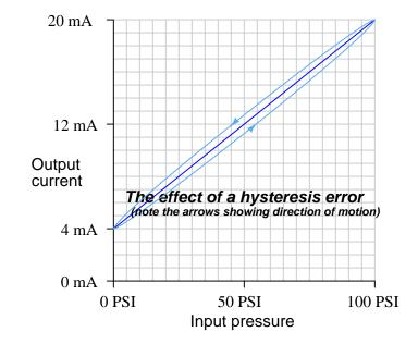
Hysteresis errors are almost always caused by mechanical friction on some moving element (and/or a loose coupling between mechanical elements) such as bourdon tubes, bellows, diaphragms, pivots, levers, or gear sets. Flexible metal strips called *flexures* – which are designed to serve as frictionless pivot points in mechanical instruments – may also cause hysteresis errors if cracked or bent.
