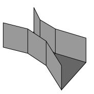
Like weirs, flumes generate upstream liquid level height changes indicative of flow rate. One of the most common flume design is the *Parshall flume*, named after its inventor R.L. Parshall when it was developed in the year 1920.
