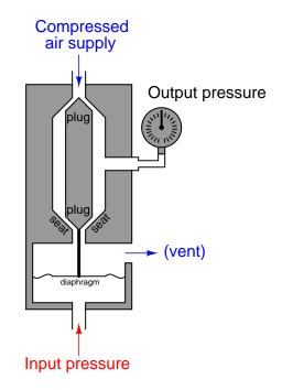
The gain (A) of any pneumatic relay is defined just the same as the gain of any electronic amplifier circuit, the ratio of output change to input change:
