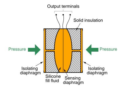
Any difference of pressure across the cell will cause the diaphragm to flex in the direction of least pressure. Since capacitance between conductors is inversely proportional to the distance separating them, this causes capacitance on the low-pressure side to increase and capacitance on the highpressure side to decrease:
