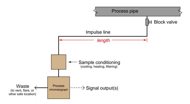
gas to make its way through the long impulse tube to the analyzer to be sampled!
