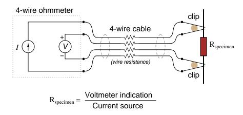
Only the outer two conductors carry substantial current. The inner two conductors connecting the voltmeter to the test specimen carry negligible current (due to the voltmeter's extremely high input impedance) and therefore drop negligible voltage along their lengths. Voltage dropped across the current-carrying (outer) wires is irrelevant, since that voltage drop is never detected by the voltmeter.
