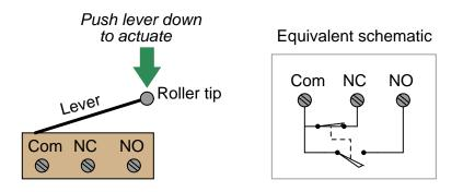
This switch contact arrangement is sometimes referred to as a *form-C* contact set, since it incorporates both a form-A contact (normally-open) as well as a form-B contact (normally-closed).
