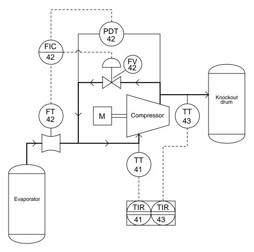
Now we see there is more instrumentation associated with the compressor than just a flow transmitter. There is also a differential pressure transmitter (PDT), a flow indicating controller (FIC), and a "recycle" control valve that allows some of the vapor coming out of the compressor's discharge line to go back around into the compressor's suction line. Additionally, we have a pair of temperature transmitters that report suction and discharge line temperatures to an indicating recorder.
