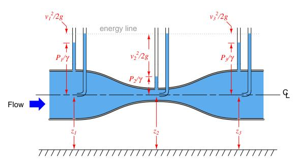
A more realistic scenario would show the influence of energy lost in the system due to friction. Here, the total energy is seen to decrease as a result of friction:
