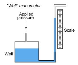
Due to the well's much larger cross-sectional area, liquid motion inside of it is negligible compared to the motion of liquid inside the clear viewing tube. For all practical purposes, the only liquid motion is inside the smaller tube. Thus, the well manometer provides an easier means of reading pressure: no longer does one have to measure the difference of height between two liquid columns, only the height of a single column.
