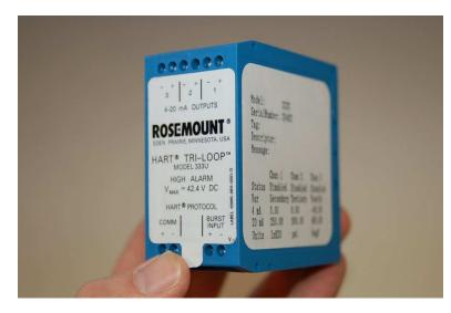
This device polls the multi-variable transmitter and converts up to three HART variables into independent 4-20 mA analog output signals, which any suitable analog indicator or controller device may receive.
