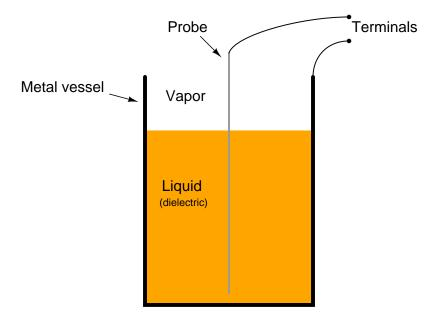
In this style of capacitive level probe, the variable is permittivity ( $\epsilon$ ), provided the liquid has a substantially greater permittivity than the vapor space above the liquid. This means total capacitance will be greatest when the vessel is full (average permittivity  $\epsilon$  is at a maximum), and least when the vessel is empty.
