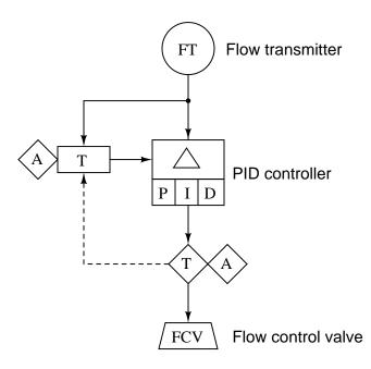
Here we see a new type of line: dashed instead of solid. This too has meaning in the world of SAMA diagrams. Solid lines represent analog (continuously variable) signals such as process variable, setpoint, and manipulated variable. Dashed lines represent discrete (on/off) signal paths, in this case the auto/manual state of the controller commanding the PID algorithm to get its setpoint either from the operator's input (A) or from the process variable input (the flow transmitter: FT).
