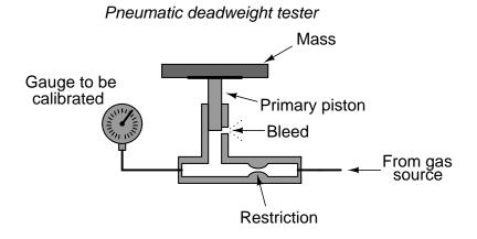
In fact, the construction and operation of a pneumatic deadweight tester is quite similar to a self-balancing (force-balance) pneumatic instrument mechanism with a baffle/nozzle assembly. A moving element opens or closes a variable restriction downstream of a fixed restriction to generate a varying pressure. In this case, that pressure directly operates the bleed vent to self-regulate gas pressure at whatever value is necessary to suspend the mass against gravity.
