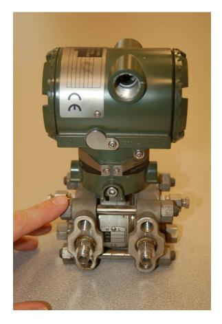
Even when disassembled, the transmitter does not look much different from the more common differential capacitance sensor design. Process pressure enters through ports in two flanges, presses against a pair of isolating diaphragms, transferring motion to the sensing diaphragm where the resonant elements change frequency with diaphragm strain:
