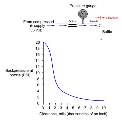
The physical distance between the baffle and the nozzle alters the resistance of air flow through the nozzle. This in turn affects the air pressure built up inside the nozzle (called the nozzle *backpressure*). Like a voltage divider circuit formed by one fixed resistor and one variable resistor, the baffle/nozzle mechanism "divides" the pneumatic source pressure to a lower value based on the ratio of restrictiveness between the nozzle and the fixed orifice.
