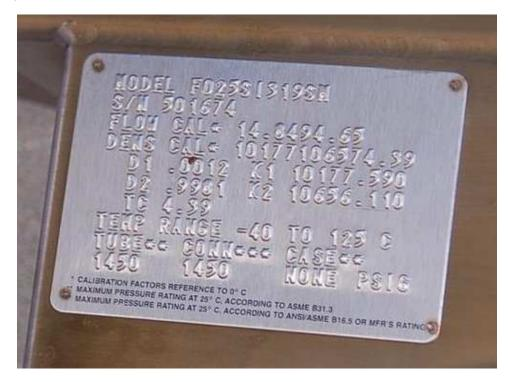
Coriolis flowmeters are equipped with RTD temperature sensors to continuously monitor the process fluid temperature. Fluid temperature is important to know because it affects certain properties of the tubes (e.g. spring constant, diameter, and length). The temperature indication is usually accessible as an auxiliary output, which means a Coriolis flowmeter may double as a (very expensive!) temperature transmitter.
