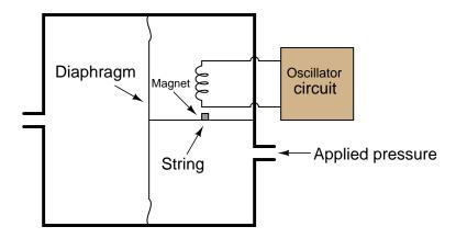
The Foxboro company pioneered this concept in an early *resonant wire* design of pressure transmitter. Later, the Yokogawa corporation of Japan applied the concept to a pair of micro-machined<sup>4</sup> silicon resonator structures, which became the basis for their successful line of "DPharp" pressure transmitters. A photograph of a Yokogawa model EJA110 pressure transmitter with this technology is seen here:
