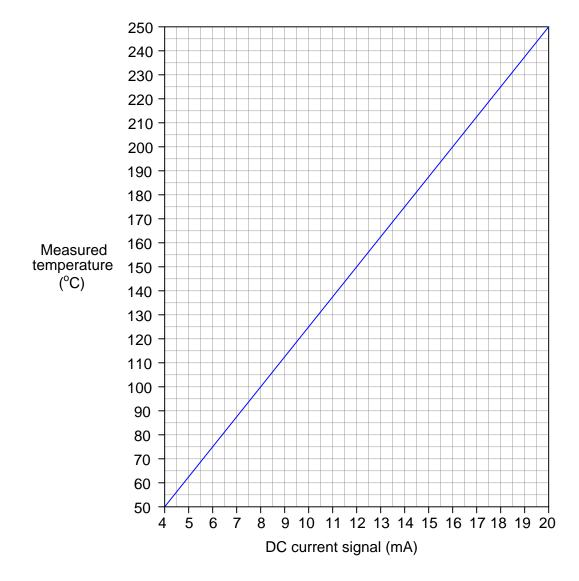
This is not unlike the pneumatic instrument signal standard or 3 to 15 pounds per square inch (PSI), where a varying air pressure signal represents some process measurement in an analog (proportional) fashion.
