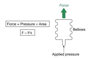
If the bellows' expansion is externally restrained so it does not stretch appreciably – and therefore the metal never gets the opportunity to act as a restraining spring – the force exerted by the bellows on that restraining object will *exactly* equal the pneumatic pressure multiplied by the cross-sectional area of the bellows' end.
