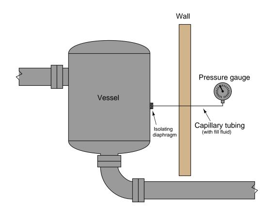
Such systems are often referred to as *remote seals*, and they are available on a number of different pressure instruments including gauges, transmitters, and switches. If the purpose of an isolating diaphragm and fill fluid is to protect the sensitive instrument from corrosive or otherwise harsh chemicals, it is often referred to as a *chemical seal*.
