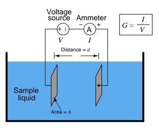
The conductance measured by this instrument is a function of plate geometry (surface area and distance of separation) as well as the ionic activity of the solution. A simple increase in separation distance between the probe electrodes will result in a decreased conductance measurement (increased resistance R) even if the liquid solution's ionic properties do not change. Therefore, conductance (G) is not particularly useful as an expression of liquid conductivity.
