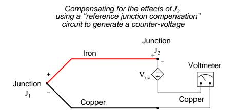
This technique is known as *hardware* compensation. A stand-alone circuit designed to do this is sometimes called an *ice point*, because it electrically accomplishes the same thing as physically placing the reference junction(s) in a bath of ice-water.
