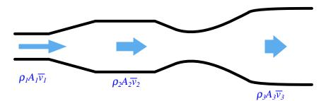
Fluid continuity is an expression of a more fundamental law of physics: the *Conservation of Mass.* If we assign appropriate units of measurement to the variables in the continuity equation, we see that the units cancel in such a way that only units of mass per unit time remain:
