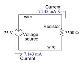
Note: arrows point in the direction of electron motion
