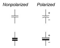
A capacitor's capacitance is related to the electric permittivity of the dielectric material (symbolized by the Greek letter "epsilon,"  $\epsilon$ ), the cross-sectional area of the overlapping plates (A), and the distance separating the plates (d):
