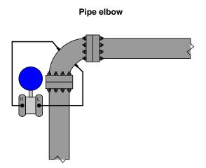
Pipe elbows should be considered for flow measurement only as a last resort. Their inaccuracies tend to be extreme, owing to the non-precise construction of most pipe elbows and the relatively weak differential pressures generated<sup>8</sup>.
