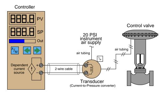
This particular controller has two digital displays, one for process variable (PV) and one for setpoint (SP), with a bargraph for displaying the output value (Out). One pushbutton provides the operator with a way to switch between Automatic and Manual modes (A/M), while two other pushbuttons provide means to decrement and increment either the setpoint value (in Automatic mode) or the Output value (in Manual mode).
