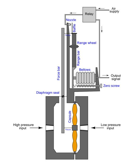
Part of the reason for this instrument's popularity is the extreme utility of differential pressure transmitters in general. A "DP cell" may be used to measure pressure, vacuum, pressure differential, liquid level, liquid or gas flow, and even liquid density. A reason for this *particular* differential
