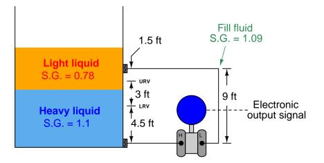
As the first step in our "thought experiment," we imagine what the process would look like with the interface at the LRV level, calculating hydrostatic pressures seen at each side of the transmitter:
