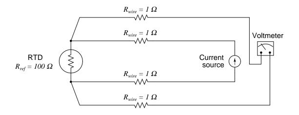
Current is supplied to the RTD from a current source, whose job it is to precisely regulate current regardless of circuit resistance. A voltmeter measures the voltage dropped across the RTD, and Ohm's Law is used to calculate the resistance of the RTD  $(R = \frac{V}{I})$ .
