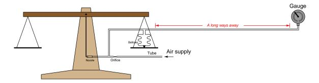
By equipping the scale with a pneumatic self-balancing apparatus, we have turned it into a *pneumatic mass transmitter*, capable of relaying the mass measurement in pneumatic, analog form to an indicating gauge far away. This is the basic *force-balance* principle used in most pneumatic industrial transmitters to convert some process measurement into a 3-15 PSI pneumatic signal.
