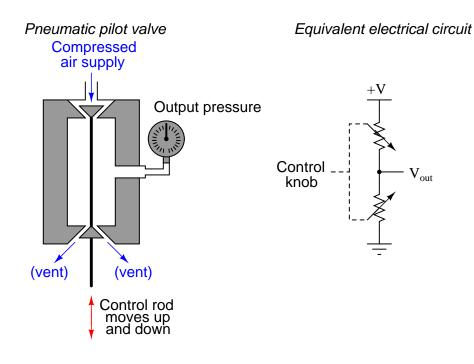
At this point, all we've managed to accomplish is build a better baffle/nozzle mechanism. We still do not yet have a pneumatic equivalent of an electronic transistor. To accomplish that, we must have some way of allowing an air pressure signal to control the motion of a pilot valve's control rod. This is possible with the addition of a *diaphragm*, as shown in this illustration:
