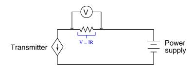
If neither component (diode nor resistor) is pre-installed in the circuit, and if a Hall-effect (clampon) precision milliammeter is unavailable, a technician may still perform useful troubleshooting measurements using nothing but a DC voltmeter. Here, however, one must be careful of how to interpret these voltage measurements, for they may not directly correspond to the loop current as was the case with measurements taken in parallel with the precision resistor.
