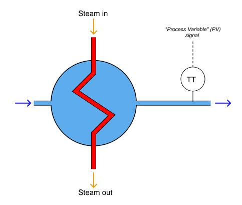
The signal coming from the transmitter (shown in the illustration by the dashed line), representing the heated fluid's exiting temperature, is called the *process variable*. Like a variable in a mathematical equation that represents some story-problem quantity, this signal represents the measured quantity we wish to control in the process.
