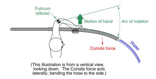
We cannot build a Coriolis flowmeter exactly like the water hose illustration shown above unless we are willing to let the process fluid exit the tubing, so a common Coriolis flowmeter design uses a U-shaped tube that redirects the fluid flow back to the center of rotation. The curved end of the flexible U-tube is forced to shake back and forth while the tube ends anchor to a stationary manifold:
