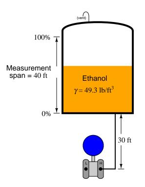
This means the transmitter's impulse line contains a 30-foot elevation head of ethanol, so that the transmitter "sees" 30 feet of ethanol when the tank is empty and 70 feet of ethanol when the tank is full. A 3-point calibration table for this instrument would look like this, assuming a 4 to 20 mA DC output signal range:
