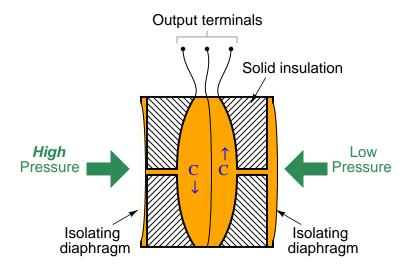
A capacitance detector circuit connected to this cell uses a high-frequency AC excitation signal to measure the different in capacitance between the two halves, translating that into a DC signal which ultimately becomes the signal output by the instrument representing pressure.
