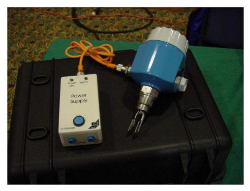
An electronic circuit continuously excites the tuning fork, causing it to mechanically vibrate. When the prongs of the fork contact anything with substantial mass, the resonant frequency of the structure dramatically decreases. The circuit detects this change and indicates the presence of material contacting the fork.
