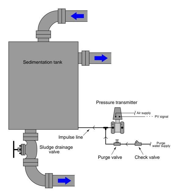
A continuous flow of clean water enters through a "purge valve" and flows through the impulse line, keeping it clear of sediment while still allowing the pressure instrument to sense pressure at
