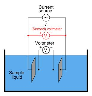
Any form of electrode fouling will cause this secondary voltage measurement to rise, thus providing an indicator that instrument technicians may use for predictive maintenance (telling them when the probes need cleaning or replacement). Meanwhile, the primary voltmeter will do its job of accurately measuring liquid conductivity so long as the current source is still able to output its normal amount of current.
