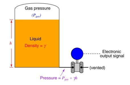
A pressure transmitter has no way of "knowing" how much of the sensed pressure is due to liquid elevation and how much of it is due to pressure existing in the vapor space above the liquid. Unless a way can be found to compensate for any non-hydrostatic pressure in the vessel, this extra pressure will be interpreted by the transmitter as additional liquid level.
