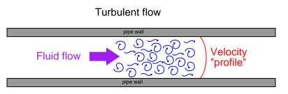
A generally accepted rule-of-thumb is that Reynolds number values less than 10,000 will probably be laminar, while values in excess of 10,000 will probably be turbulent. There is no definite threshold value for all fluids and piping configurations, though.
