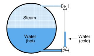
Looking at the sightglass as a U-tube manometer again, we see that unequal-height liquid columns may indeed balance each other's hydrostatic pressures if the two columns are comprised of liquids with different densities. The weight density of water is  $62.4 \text{ lb/ft}^3$  at standard temperature, but may be as low as only  $36 \text{ lb/ft}^3$  at temperatures common for power generation boilers.
