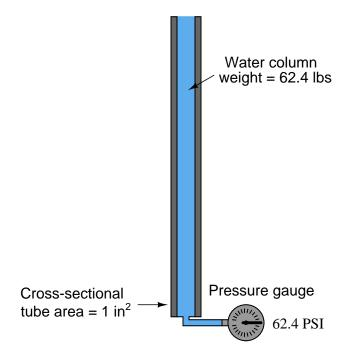
Naturally, we would expect the pressure measured at the bottom of this tall tube to be 62.4 pounds per square inch, since the entire column of water (weighing 62.4 pounds) has its weight supported by one square inch of area.
