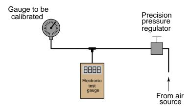
When the electronic test gauge is designed for very low pressures (inches of water column), they are sometimes referred to as *electronic manometers*.
