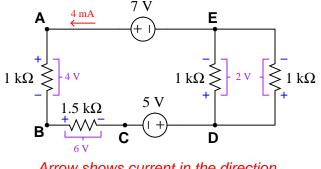
Arrow shows current in the direction of conventional flow notation
