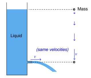
This was discovered by Evangelista Torricelli almost 100 years prior to Bernoulli's more comprehensive formulation. The velocity may be determined by solving for v after setting the potential and kinetic energy formulae equal to each other (since all potential energy at the upper height must translate into kinetic energy at the bottom, assuming no frictional losses):
