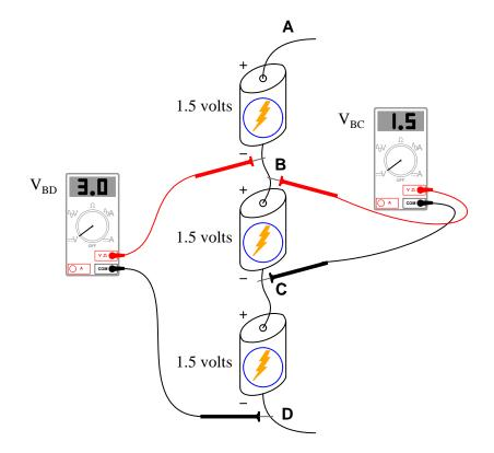
The voltage as measured between any two points directly across a single battery will be 1.5 volts:
