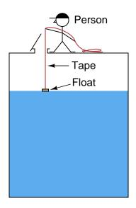
A person lowers a float down into a storage vessel using a flexible measuring tape, until the tape goes slack due to the float coming to rest on the material surface. At that point, the person notes the length indicated on the tape (reading off the lip of the vessel access hole).
