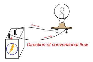
This relationship between voltage polarity marks and conventional flow current makes more intuitive sense than electron flow notation, because it is reminiscent of fluid pressure and flow direction:
