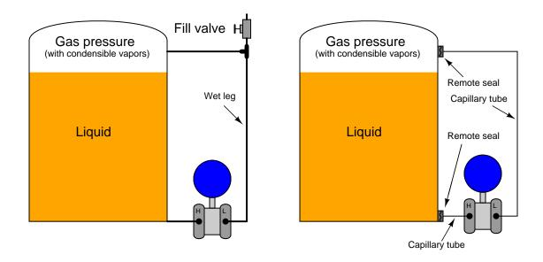
The following example shows the calibration table for a compensated-leg (wet) hydrostatic level measurement system, for a gasoline storage vessel and water as the wet leg fill fluid. Here, I am assuming a density of  $41.0 \text{ lb/ft}^3$  for gasoline and  $62.4 \text{ lb/ft}^3$  for water, with a 0 to 10 foot measurement range and an 11 foot wet leg height:
