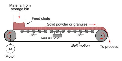
The load cell measures the weight of a fixed-length belt section, yielding a figure of material weight per linear distance on the belt. A tachometer (speed sensor) measures the speed of the belt. The product of these two variables is the mass flow rate of solid material "through" the weighteeder:
