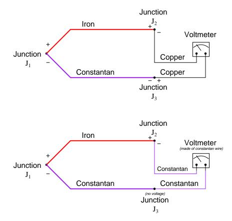
The practical import of all this is we can always treat the reference junction(s) as a single junction made from the same two metal types as the measurement junction, so long as all dissimilar metal
