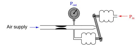
We call this a *motion* balance system instead of a *force* balance system because we see two motions canceling each other out to maintain a constant nozzle gap instead of two forces canceling each other out to maintain a constant nozzle gap.
