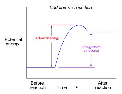
A *catalyst* is a substance that works to minimize activation energy in a chemical reaction without being altered by the reaction itself. Catalysts are popularly used in industry to accelerate both exothermic and endothermic reactions, reducing the gross amount of energy that must be initially input to a process to make a reaction occur. A common example of a catalyst is the *catalytic*
