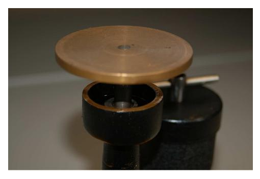
A common operating practice for any deadweight tester is to gently spin the mass during testing so that the primary piston continually rotates within its cylinder. Any motion will prevent static friction from taking hold, helping to ensure the only force on the primary piston is the force of the fluid within the deadweight tester.
