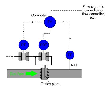
Note the location of the RTD (thermowell), positioned downstream of the orifice plate so that the turbulence it generates will have negligible impact on the fluid dynamics at the orifice plate. The American Gas Association (AGA) allows for upstream placement of the thermowell, but only if located at least three feet upstream of a flow conditioner<sup>12</sup>.
