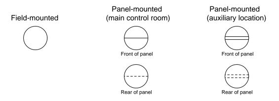
The type of "bubble" used for each instrument tells us something about its location. This, obviously, is quite important when working in a facility with many thousands of instruments scattered over acres of facility area, structures, and buildings.
