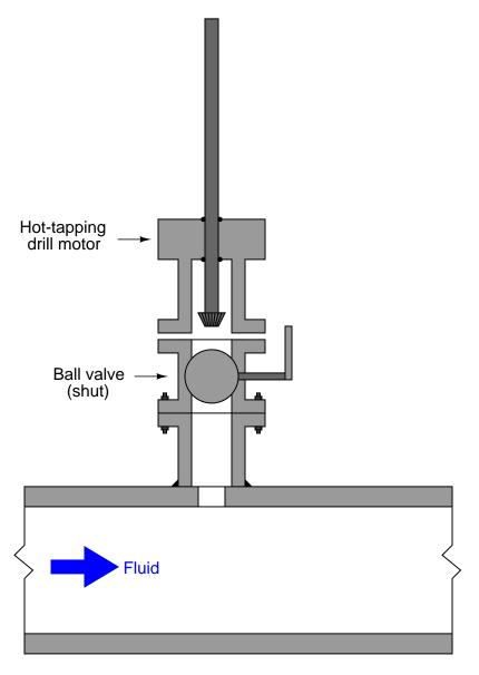
Now there is a flanged and isolated connection into the "hot" pipe, through which an insertion flowmeter (or other instrument/device) may be installed.
