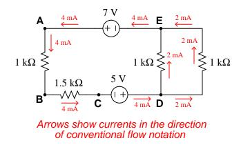
At nodes where just two wires connect (such as points A, B, and C), the amount of current going in to the node exactly equals the amount of current going out (4 mA, in each case). At nodes where three wires join (such as points D and E), we see one large current and two smaller currents (one 4 mA current versus two 2 mA currents), with the directions such that the sum of the two smaller currents form the larger current.
