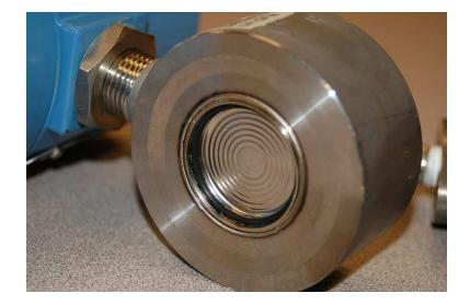
The differential capacitance sensor inherently measures *differences* in pressure applied between its two sides. In keeping with this functionality, this pressure instrument has two threaded ports into which fluid pressure may be applied. A later section in this chapter will elaborate on the utility of differential pressure transmitters (section 12.5 beginning on page 316).
