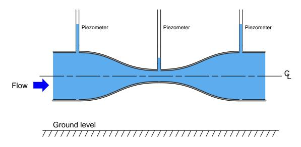
If we add three more piezometers to the venturi tube assembly, each one equipped with its own *Pitot tube* facing upstream to "catch" the velocity of the fluid, we see that total energy is indeed conserved at every point in the system. Here, each of the "heads" represented in Bernoulli's equation are shown in relation to the different piezometer heights:
