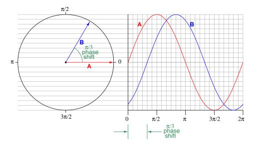
Graphically computing the sum of these two waves would be quite difficult in the standard graph (right-hand side), but it is as easy as stacking vectors tip-to-tail in the crank diagram:
