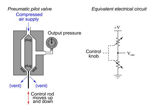
As the control rod is moved up and down, *both* variable restrictions change in complementary fashion. As one restriction opens up, the other pinches shut. The combination of two restrictions changing in opposite direction results in a much more aggressive change in output pressure as registered by the gauge.
