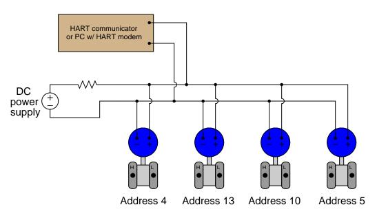
Setting an instrument's HART address to a non-zero value is all that is necessary to engage multidrop mode. The address numbers themselves are irrelevant, as long as they fall within the range of 1 to 15 and are unique to that network.
