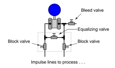
While this illustration shows the three values as separate devices, connected together and to the transmitter by tubing, three-value manifolds are more commonly manufactured as monolithic devices: the three values cast together into one block of metal, attaching to the pressure transmitter by way of a flanged face with O-ring seals. Bleed values are most commonly found as separate devices threaded into one or more of the ports on the transmitter's diaphragm chambers.
