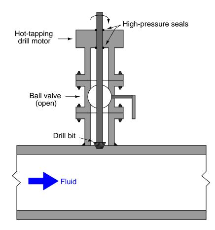
Once the hole has been completely drilled, the bit is extracted and the ball valve shut to allow removal of the hot-tapping drill:
