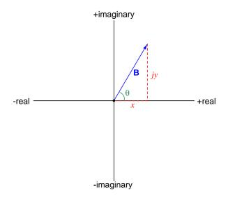
Alternatively, we could express this complex quantity in polar form as an amplitude (B) and an angle  $(\Theta)$ , using the cosine and sine functions to translate this amplitude and angle into rectangular
