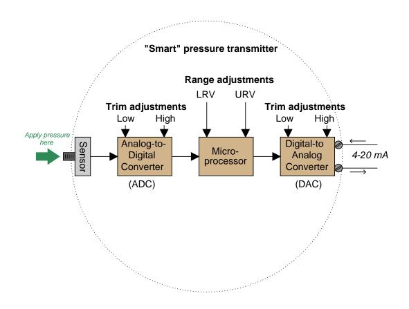
It is important to note all the adjustments within this device, and how this compares to the relative simplicity of an all-analog pressure transmitter:
