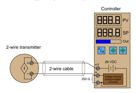
It is very common to find controllers with their own built-in loop power supplies, due to the popularity of loop-powered (2-wire) 4-20 mA transmitters. If we know the transmitter requires a DC voltage source somewhere in the circuit to power it up, it makes sense to include one in the controller, right?
