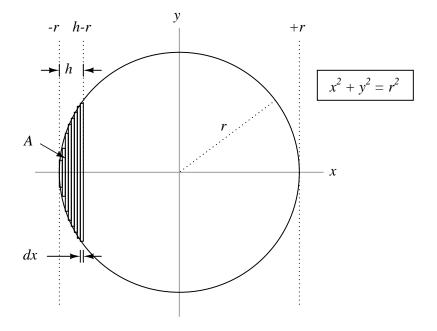
In this sketch, I show the circle "filling" from left to right rather than from bottom to top. I have done this strictly out of mathematical convention, where the x (horizontal) axis is the independent variable. No matter how the circle gets filled, the relationship of area (A) to fill distance (h) will be the same.
