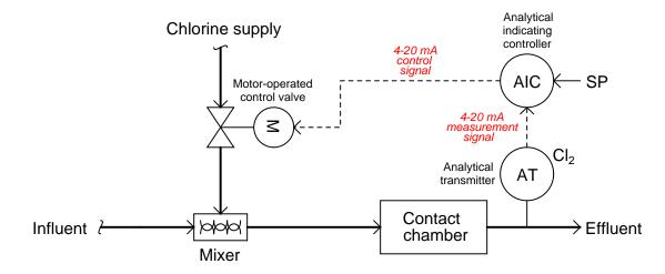
Chlorine gas coming through the control valve mixes with the incoming water (influent), then has time to disinfect in the contact chamber before exiting out to the environment.
