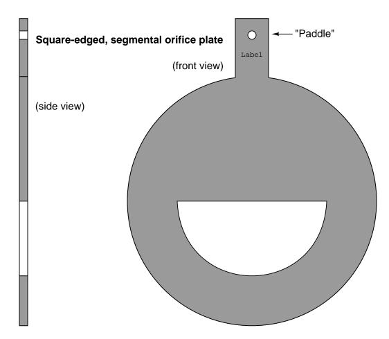
As with the eccentric orifice plate design, the segmental hole should be offset downward in gas flow applications and either upward or downward in liquid flow applications depending on the type of undesired material(s) in the flowstream.
