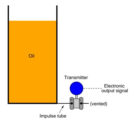
Connected as such, the differential pressure transmitter functions as a gauge pressure transmitter, responding to hydrostatic pressure exceeding ambient (atmospheric) pressure. As liquid level increases, the hydrostatic pressure applied to the "high" side of the differential pressure transmitter also increases, driving the transmitter's output signal higher.
