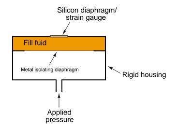
The isolating diaphragm is designed to be much more flexible (less rigid) than the silicon diaphragm, because its purpose is to seamlessly transfer fluid pressure from the process fluid to
