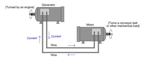
Given the proper metal alloys, the friction that electrons experience within the metal wires may be made very small, allowing nearly all the energy to be expended at the load (motor), with very little wasted along the path (wires). This makes electricity the most efficient means of energy transport known.
