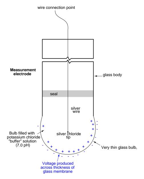
Any concentration of hydrogen ions in the process solution differing from the hydrogen ion concentration in the buffer solution  $([H^+] = 1 \times 10^{-7} M)$  will cause a voltage to develop across the thickness of the glass. Thus, a standard pH measurement electrode produces no potential when the process solution's pH value is exactly 7.0 pH (equal in hydrogen ion activity to the buffer solution trapped within the bulb).
