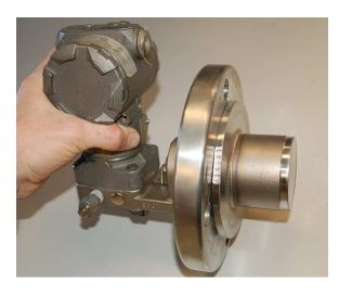
The calibration table for a transmitter close-coupled to the bottom of an oil storage tank would be as follows, assuming a zero to twelve foot measurement range for oil height, an oil density of 40 pounds per cubic foot, and a 4-20 mA transmitter output signal range:
