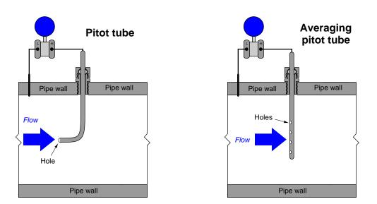
A variation on the latter theme is the *Annubar* flow element, a trade name of the Dieterich Standard corporation. An "Annubar" is an averaging pitot tube consolidating high and low pressuresensing ports in a single probe assembly:
