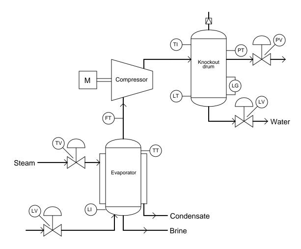
One might guess the instrument interconnections based on the instruments' labels. For instance, a good guess would be that the level transmitter (LT) on the bottom of the knockout drum might send the signal that eventually controls the level valve (LV) on the bottom of that same vessel. One might also guess that the temperature transmitter (TT) on the top of the evaporator might be part of the temperature control system that lets steam into the heating jacket of that vessel.
