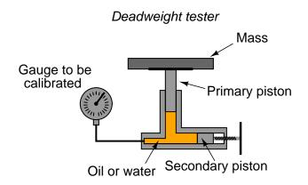
After connecting the gauge (or other pressure instrument) to be calibrated, the technician adjusts the secondary piston to cause the primary piston to lift off its resting position and be suspended by oil pressure alone. So long as the mass placed on the primary piston is precisely known, Earth's gravitational field is constant, and the piston is perfectly vertical, the fluid pressure applied to the instrument under test *must* be equal to the value described by the following equation:
