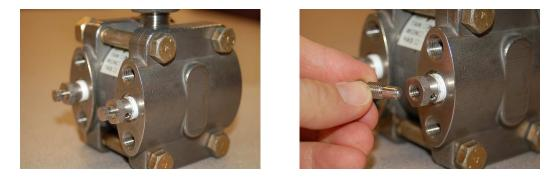
When installed directly on the flanges of a pressure instrument, these bleed valves may be used to bleed unwanted fluids from the pressure chambers, for example bleeding air bubbles from an instrument intended to sense water pressure, or bleeding condensed water out of an instrument intended to sense compressed air pressure.
