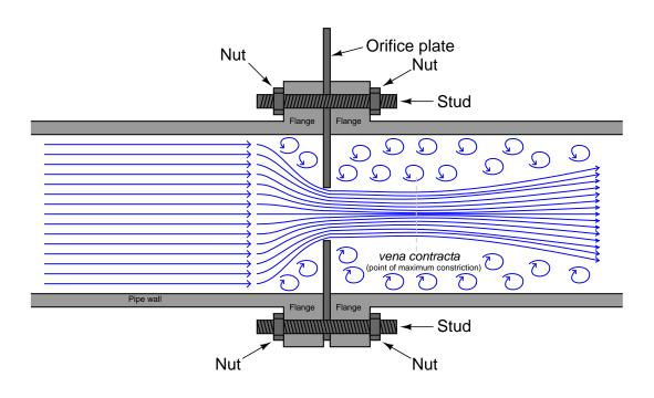
The point where the fluid flow profile constricts to a minimum cross-sectional area after flowing through the orifice is called the *vena contracta*, and it is the area of minimum fluid pressure. The vena contracta corresponds to the narrow throat of a venturi tube.
