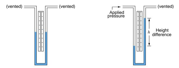
Pressure is read on the scale as the difference in height (h) between the two liquid columns. One nice feature of a manometer is that it really cannot become "uncalibrated" so long as the fluid is pure and the assembly is maintained in an upright position. If the fluid used is water, the manometer may be filled and emptied at will, and even rolled up for storage if the tubes are made of flexible plastic.
