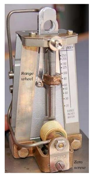
As in all instruments, the zero adjustment works by *adding or subtracting* a quantity, while the span adjustment works by *multiplying or dividing* a quantity. In the Foxboro model 13 pneumatic transmitter, the quantity in question is force. The zero screw adds or subtracts force to the mechanical system by tensioning a spring, while the range wheel multiplies or divides force in the
