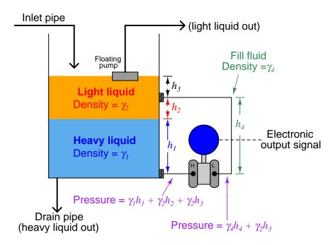
Since both sides of the differential pressure transmitter "see" the hydrostatic pressure generated by the liquid column above the top connection point  $(\gamma_2 h_3)$ , this term is naturally canceled:
