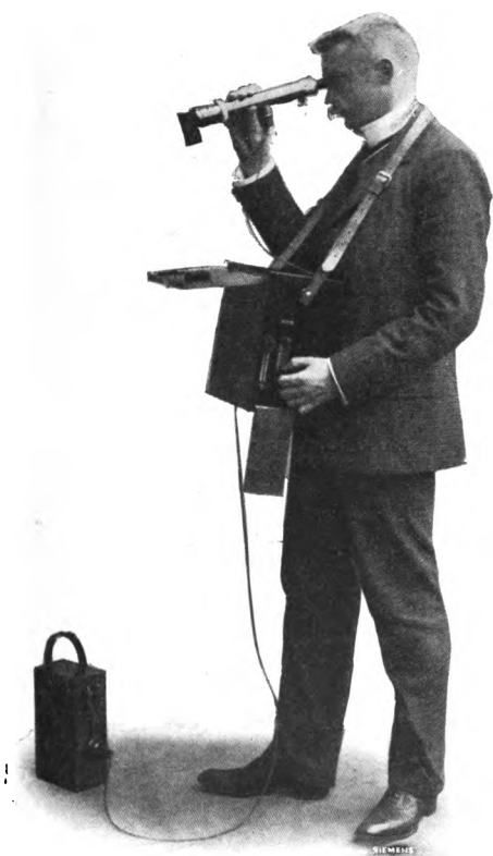
FIG. 54.—SIEMENS' OPTICAL PYROMETER, PORTABLE FORM.
