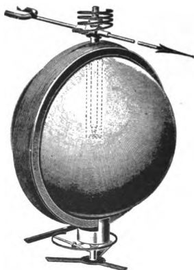
FIG. 12.—PRINCIPLE OF SINGLE-PIVOT GALVANOMETER.
