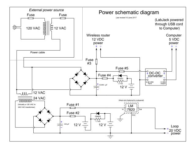
Power is sent to each RTU box at 12 volts AC, from a transformer located near a 120 VAC power source. This keeps the field power cable at a safe, low voltage (similar to outside sprinkler control systems and walkway lighting).
