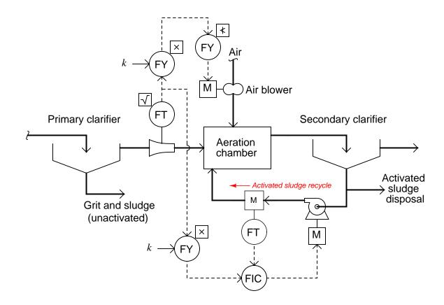
Suppose the magnetic flowmeter used to measure sludge recycle flow imparts a magnetic flux density of 0.2 Tesla across a flowtube 4 inches in diameter (10.16 centimeters, or 0.1016 meters). Calculate the amount of voltage this flowtube will generate at a sludge flow rate of 0.67 cubic meters per minute. Also, convert this sludge flow rate into units of gallons per minute.
