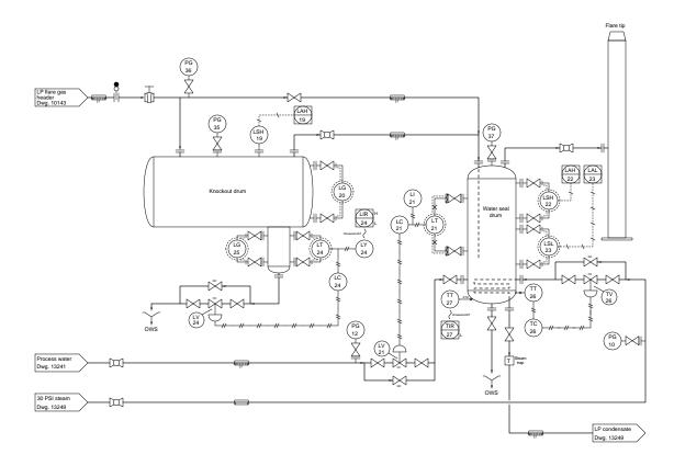
As with most flare systems, the exact composition of material sent to the flare to be burned is both highly variable and unknown from moment to moment. In a typical refinery, anything from hydrogen gas to diesel fuel might get sent to the flare during a "depressurization" event.
