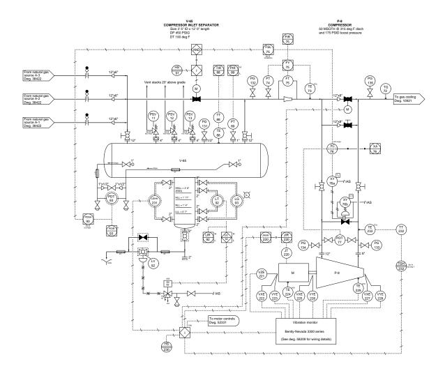
Flowmeter FT-75 has been in service for many years, but unfortunately does not provide good enough turndown for operations' needs when the compressor is operated at a fraction of its rated capacity. Engineers are debating what type(s) of flowmeter might be used to replace FT-75.
