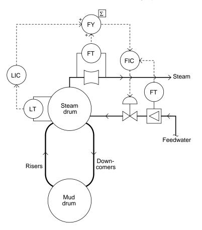
Supposing this venturi tube normally develops a differential pressure of 100 inches water column at a flow rate of 970 pounds per minute with a steam density of  $\rho = 1.33$  lbm/ft<sup>3</sup>, calculate the following:
