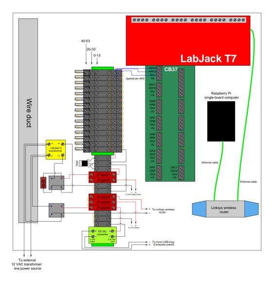
Each RTU enclosure is weatherproof, and equipped with a set of batteries to maintain DC power to all the system components in the event of an external AC power failure.
