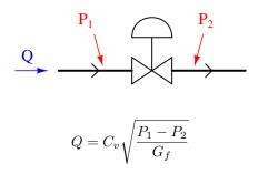
The variable  $C_v$  is called the *flow coefficient* of the control valve, and it varies from zero at full-closed to a certain maximum value (depending on valve size and type) at wide-open.
