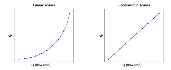
Flow elements such as orifice plates, venturi tubes, Pitot tubes, and flow nozzles should exhibit a simple quadratic characteristic, represented by the formula  $Q = k\sqrt{\Delta P}$ . Logarithmic scales are very helpful when graphing inherently nonlinear functions such as this. Note what happens to this quadratic function when the logarithm is taken of both sides:
