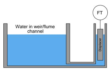
This level-sensing instrument usually provides the characterization necessary to linearize the weir or flume's nonlinear flow/height response. If the level-sensing instrument is ultrasonic, the flow characterization may be done in the same digital computer that calculates liquid level by timing the sound echoes.
