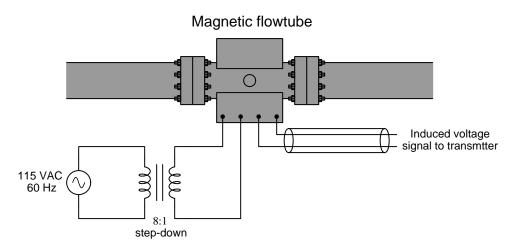
The magnitude of the induced voltage signal is a function of the field coil's magnetic flux density (B), the velocity of the fluid moving through the flowtube (v), and the diameter of the flowtube (d). The phase angle of the induced voltage signal will be the same as the phase angle of the current through the field coil, relative to the source voltage.
