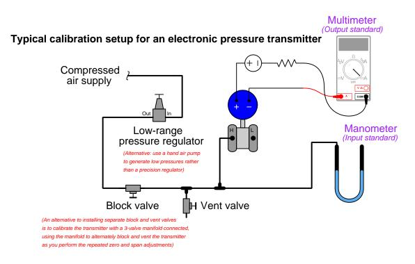
If the low-range pressure regulator does not reliably generate low enough pressures, you may throttle both the block and vent valves, using them as a sort of "pressure divider" (analogous to two resistors throttling current to make a voltage divider) to apply a lower pressure to the manometer and DP transmitter than the regulator outputs:
