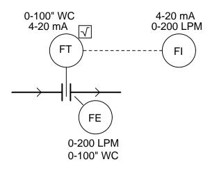
Note that the transmitter is equipped with internal square root characterization, so that no external square root computer is required.
