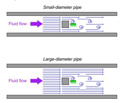
If the bluff bodies in both pipes have the same physical dimensions, and the vortex shedding frequencies are the same in both scenarios, which pipe carries a greater volumetric flow rate of water? Or, do they carry the same amount of flow? Why or why not??
