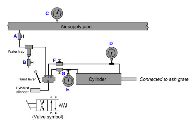
Moving the hand lever back and forth to test the system for yourself, you see that the cylinder indeed remains in its "retracted" position all the time. You see that pressure gauge  $\mathbf{C}$  registers a full 85 PSI of air pressure (as you expect it to), but neither gauges  $\mathbf{D}$  nor  $\mathbf{E}$  move from their resting indications of 0 PSI each.
