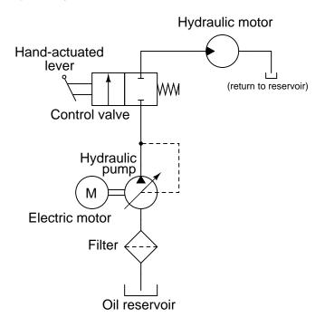
As hydraulic pressure increases, the pump mechanism automatically adjusts to give less volume displacement per rotation. Explain how this works to regulate pressure, and also why it saves energy compared to the more traditional design of a constant-displacement pump combined with a pressure-relief valve.
