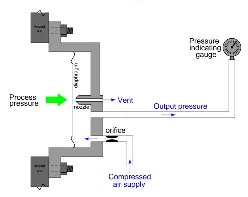
Describe the response of this device, step by step, to an increase in process pressure. Hint: the diaphragm in this device is "slack," meaning it has negligible spring effect. This means even very small pressure differences are sufficient to move the diaphragm significantly.
