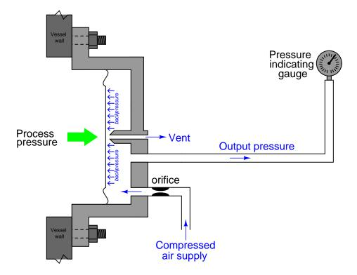
Because both pressures (process fluid, and air backpressure) act against the same amount of surface area on the diaphragm, the point of force balance between them will be when the two pressures are equal to each other. Thus, the output air pressure (sensed by some remote pressure-measuring instrument) mirrors, or "repeats," the process pressure.
