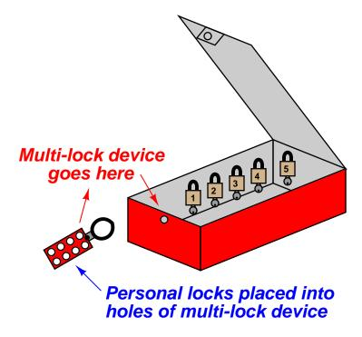
Explain how having numbered padlocks stored inside this lock-box prior to a job, and by having workers apply their personal padlocks to secure the lid of this lock-box, help to ensure the equipment will be safe for everyone to work on.
