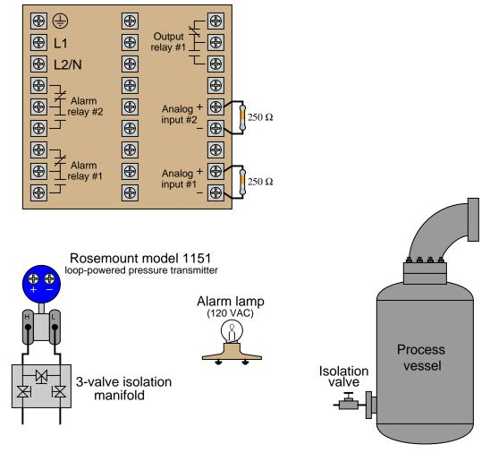
Sketch all necessary connecting wires and tubes to make this a working system. Note: you will need to add electrical power sources to the diagram! Also, identify the proper open/closed state for each hand valve contained in the pressure transmitter's three-valve isolation manifold.
