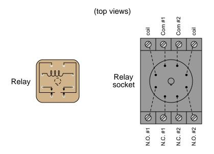
Draw the necessary connecting wires between terminals in this circuit, so that actuating the normallyopen pushbutton switch sends power from the battery to the coil to energize the relay:
