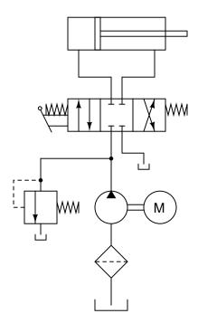
When the lever is pulled, the cylinder's piston moves in one direction. When the lever is pushed, it moves in the other direction. When the lever is released, it spring-returns to a center position, and the piston remains where it is.
