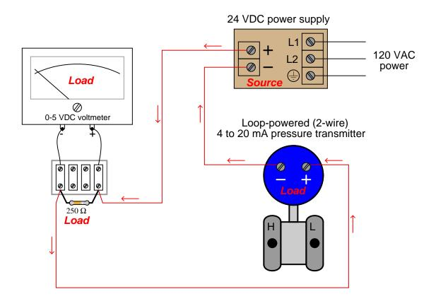
Note how current (shown in the direction of conventional flow) always exits the positive terminal of a source, and always enters the positive terminal of a load.
