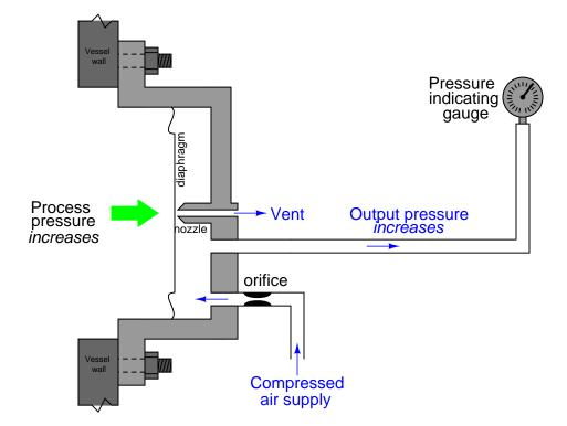
As air flow through the nozzle reduces, the "backpressure" built up by supply air through coming through the orifice increases. This increased backpressure forces the diaphragm to the left, against the process pressure, until the diaphragm begins to back away from the nozzle and a new point of balance (equilibrium) is reached:
