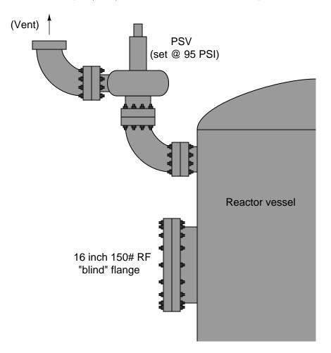
Calculate the total force exerted on a 16 inch blind flange located on the side of the reactor at the PSV lift pressure, as well as the stress imposed by this force among each of the 20 bolts holding the flange in place, both answers expressed in the unit of *pounds*. Use  $15\frac{1}{4}$  inches as the effective diameter of the blind flange.
