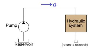
But what kind of electrical source best mimics a positive-displacement hydraulic pump turned at a constant speed, a *voltage* source or a *current* source?
