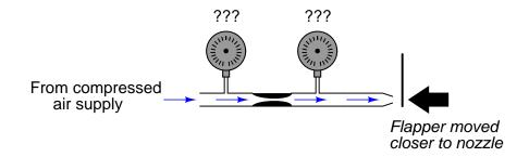
If the flapper travels further away from the nozzle, what effect will it have on the two pressure gauges' indications?
