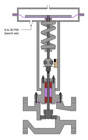
Calculate the *seat load* force applied to the seat by the plug when there is no air pressure applied to the actuator. Note: the "seat load" is a critical engineering parameter to ensure tight shut-off of the valve, especially under emergency conditions.
