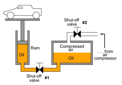
Which shut-off valve would be the safer one to close for halting the platform's upward motion when lifting an automobile off the ground? Why?
