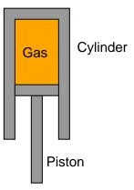
In particular, sketch how the gas pressure inside the cylinder relates to changes in cylinder volume caused by piston movement, assuming no change in gas temperature or leakage of gas molecules from the cylinder:
