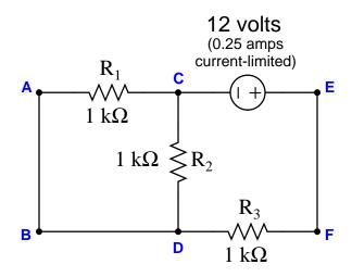
Identify the likelihood of each specified fault for this circuit. Consider each fault one at a time (i.e. no coincidental faults), determining whether or not each fault could independently account for *all* measurements and symptoms in this circuit.
