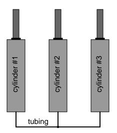
Assuming that all three pistons are the same size, calculate the force generated by the pistons of cylinders #2 and #3 if the piston of cylinder #1 is pushed with 500 pounds of force. file i00152
