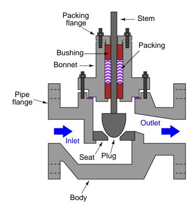
If we were to use this valve "backwards," the pressure drop across the plug would tend to "slam" it closed whenever it approached the closed position. In other words, the process fluid's differential pressure drop would make it very difficult to maintain any plug position near full-closed.
