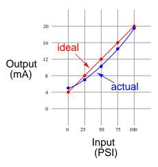
A zero error is usually correctable by simply adjusting the "zero" screw on an analog instrument, without making any other adjustments. Span errors, by contrast, usually require multiple adjustments of the "zero" and "span" screws while alternately applying 0% and 100% input range values to check for correspondence at both ends of the linear function.
