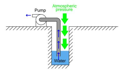
Based on this description of pump operation, what is the theoretical maximum height that any pump can lift water out of a well, assuming the well is located at sea level?
