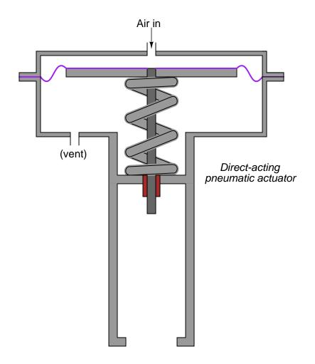
For an "air-to-open" valve, either of these two combinations will work:
