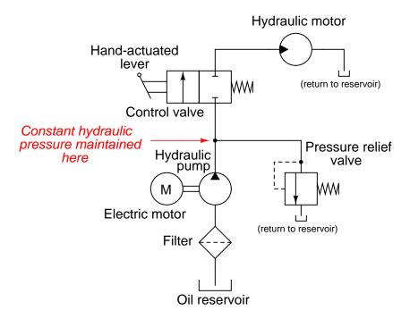
If not for the pressure-relief valve, the hydraulic pump would "lock up" and refuse to turn whenever the control valve was placed in the "stop" position (as shown in the diagram). With the pressure-relief valve in place, the pump will continue to spin and hydraulic pressure will be maintained.
