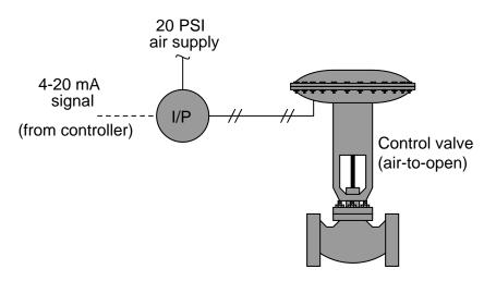
An instrument technician removes the cover from the I/P transducer and momentarily presses the baffle against the nozzle. The control valve immediately responds by opening fully.
