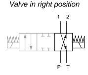
Pressure source to port 2 Port 1 return to tank (reservoir)
