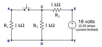
Identify the likelihood of each specified fault for this circuit. Consider each fault one at a time (i.e. no coincidental faults), determining whether or not each fault could independently account for *all* measurements and symptoms in this circuit.
