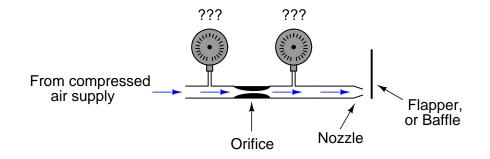
Qualitatively speaking, what would these two pressure gauges indicate? Assume that the air supply is regulated by a pressure regulator, and so remains at a constant pressure. Would the two pressure gauges indicate the same amount of pressure? Would one of them indicate a higher pressure than the other? Explain your answer.
