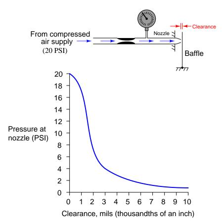
As you can see, this is a very sensitive mechanism. A nearly full swing of pressure (0 PSI to supply) is obtained with just several thousandths of an inch of baffle movement. It is this extreme sensitivity that allows us to assume there is negligible motion in a pneumatic force-balance mechanism operating within its calibrated range.
