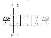
Pressure source to port 1 Port 2 return to tank (reservoir)
