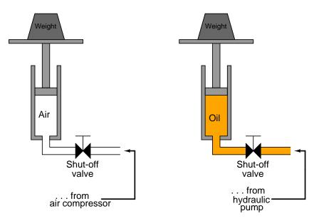
What will happen if the weight were to fall off the lift platform after it had been raised up from ground level, in each case? Assume that the shut-off valve is closed (no fluid flow from pump or compressor into the cylinder) when this happens.
