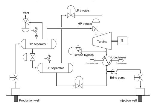
One day an operator notices something strange on the trend graph for the HP separator: the brine level in that separator seems to oscillate in a square-wave manner around the usual setpoint value, but stabilizes at any other setpoint value:
