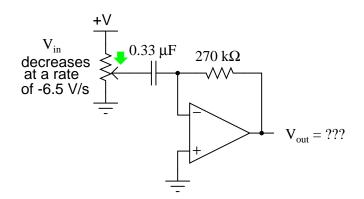
Then, calculate the "time constant" of this differentiator circuit (i.e. the factor relating output voltage to input rate-of-change).
