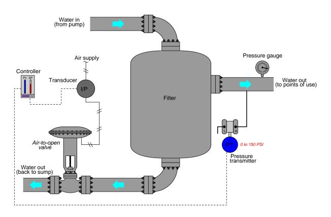
An operator tells you there is a problem with this system, though: the controller faceplate registers 146 PSI of water pressure, with a setpoint at 100 PSI. You happen to notice that the bargraph on the controller faceplate showing output is at 100%. Another operator in the field (near the exchanger) reports via radio that the control valve stem is at the "closed" position, and that the pressure gauge mounted on the filter's discharge line registers 143 PSI.
