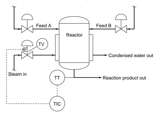
First, identify the proper *action* of the temperature controller (either direct or reverse) assuming the temperature transmitter is direct-acting, the control valve is fail-open (air-to-close), and the positioner is configured for signal-to-close.
