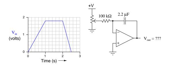
Also, calculate the "time constant" of this integrator circuit (i.e. the factor relating output voltage rate-of-change to input voltage).
