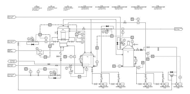
Suppose the last instrument technician to calibrate flow control valve FV-36 made a mistake, such that the valve stem position is 5% further open than it should be at all signal values. For example, if the controller sends a 25% (8 mA) signal to the control valve, it actually opens up to a stem position of 30%.
