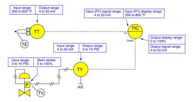
Analog (non-"smart") transmitters, I/P transducers, and valve positioners are ranged using "zero" and "span" adjustments, typically screws or nuts. The ranging of analog instruments is discussed in the "Instrument Calibration" chapter of the *Lessons In Industrial Instrumentation* textbook.
