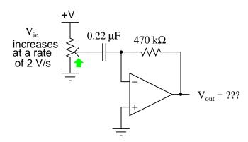
Then, calculate the "time constant" of this differentiator circuit (i.e. the factor relating output voltage to input rate-of-change).
