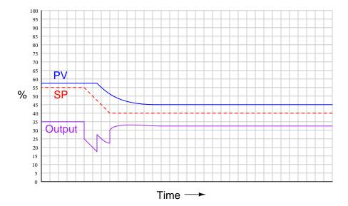
Identify which of the following algorithms is being used in this P+D controller, and how you can tell:
