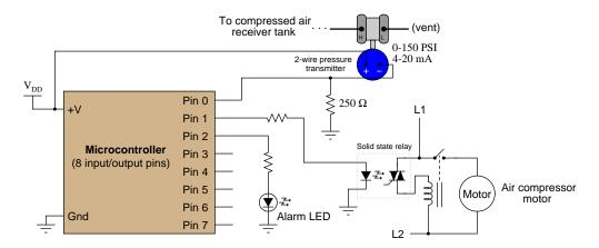
Examine the following program (written in an informal programming language called "pseudocode") and explain how the microcontroller decides when to turn the motor on and off. Also determine the pressures at which the microcontroller turns on and shuts off the compressor:
