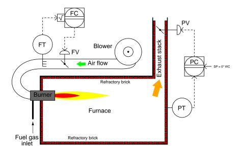
Suppose one day you are informed of a problem with this furnace: flames are seen escaping around the edges of the doors leading into the furnace while it is in operation.
