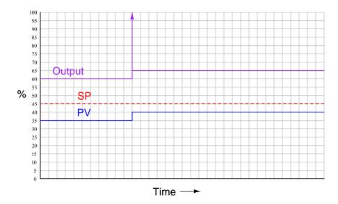
The controller output graph shown here is *qualitative* only. Although drawn to scale (i.e. all changes in the output are properly scaled relative to each other), the scale itself is arbitrary and therefore may not match the scale of your sketch:
