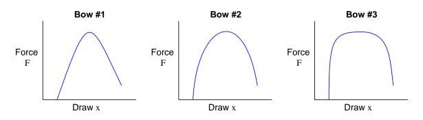
Each bow exhibits the exact same peak force, holding force, and draw length. The difference is in the shape of the cam mechanisms used to characterize each bow's draw. Examine the three force-draw curves shown here, then answer the following questions:
