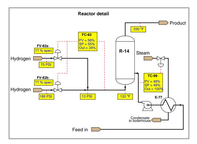
This graphic display, however, is not complete. The engineer forgot to program it to display the individual positions of valves FV-82a and FV-82b. The way it stands right now, the operator can see the controller's output signal (shown here at 34%), but cannot tell what the individual stem positions are for each of the two split-ranged valves. This task has been left to you!
