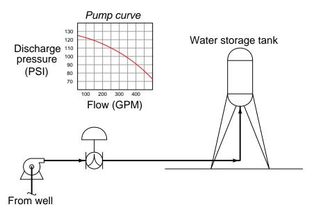
Assume a vertical distance of 195 feet from the pump discharge to the average water level in the storage tank.
