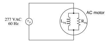
Calculate the equivalent inductance  $(L_{eq})$  if the measured source current is 27.5 amps and the motor's equivalent resistance  $(R_{eq})$  is 11.2  $\Omega$ .
