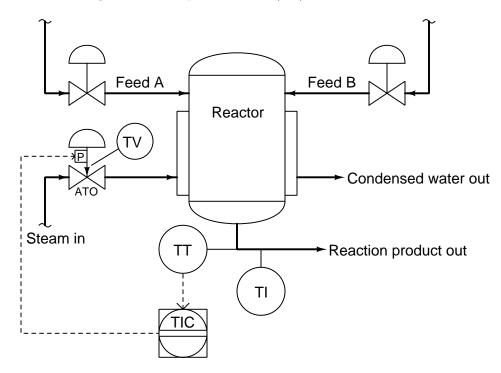
Suppose the last instrument technician to calibrate the temperature transmitter made a mistake, and the transmitter consistently reads  $15^{\circ}$  too hot. For example, if the reaction product temperature is actually  $275^{\circ}$  F, the transmitter outputs a current signal corresponding to  $290^{\circ}$  F.
