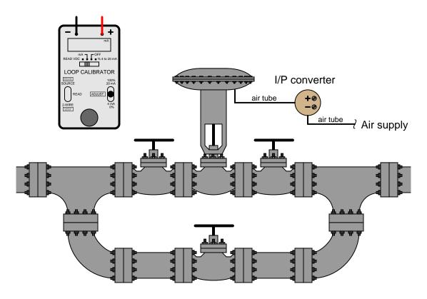
Show how you could still (creatively) use the loop calibrator to stroke the valve despite its lacking functionality – feel free to add any other electronic component(s) as necessary to make it work. Then, calculate the necessary current to send to the valve to make it open to 75%, assuming a split-range calibration of 12 mA (closed) to 20 mA (open).
