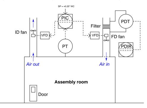
Suppose you are called to troubleshoot a problem in this system: the room air pressure is holding steady at +0.17 inches WC (according to the display on the DDC control system) with the FD fan running at 100% speed and the ID fan running at 0% speed. Based on this data, identify the most likely cause of the problem, and also how you would confirm your diagnosis *before* making any repairs.
