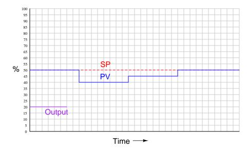
Qualitatively graph the response of a proportional-plus-derivative controller over time to the following changes in process variable:
