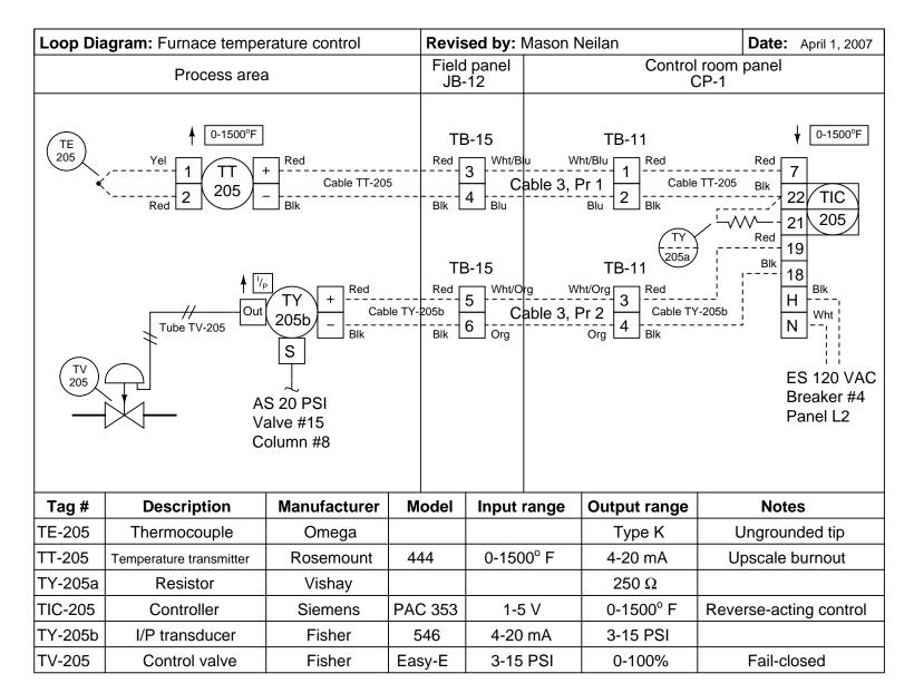
Question 92 Sample Loop Diagram (using a single-loop controller)
