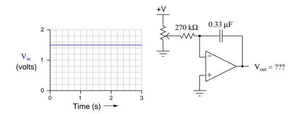
Also, calculate the "time constant" of this integrator circuit (i.e. the factor relating output voltage rate-of-change to input voltage). <u>file i01026</u>
