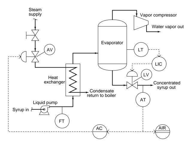
Suppose the level control valve (LV) fails completely open. Determine the effect this failure will have on the sugar concentration of the outgoing syrup.
