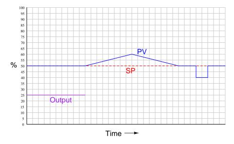
Then, draw a final graph of the controller's output, showing how the P, I, and D terms would combine to form a composite waveform:
