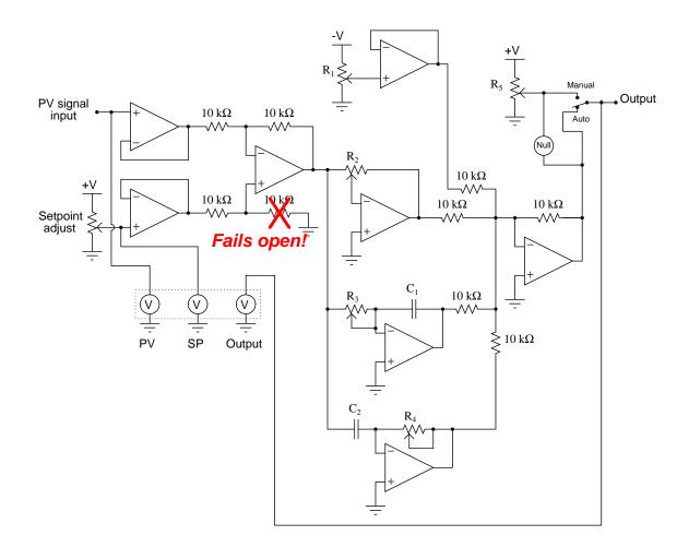
Then suddenly the resistor shown below the subtracting opamp fails open, due to a bad solder joint. Determine how the controller will drive the output signal as a result of this fault. Specifically, determine:
