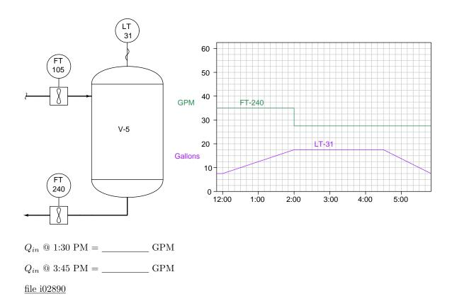
Calculate the volume of liquid discharged from this vessel between 1:00 PM and 4:00 PM based on the information shown here:
