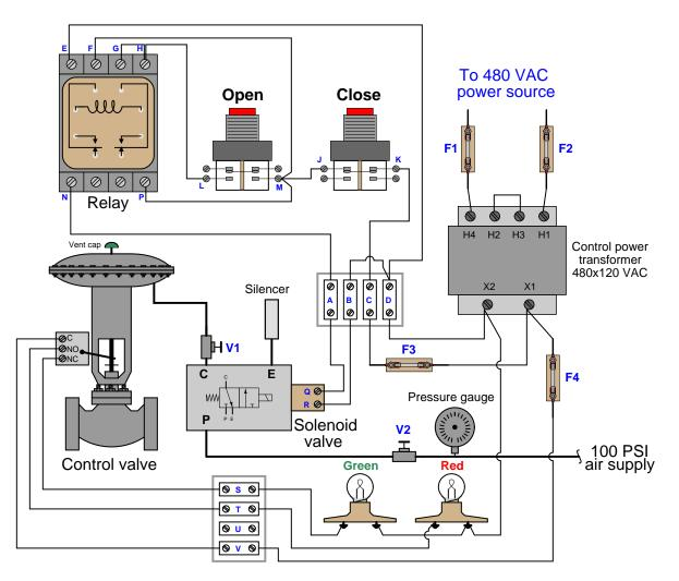
Determine the diagnostic value of each of the following tests. Assume only one fault in the system, including any single component or any single wire/cable/tube connecting components together. If a proposed test could provide new information to help you identify the location and/or nature of the one fault, mark "yes." Otherwise, if a proposed test would not reveal anything relevant to identifying the fault (already discernible from the measurements and symptoms given so far), mark "no."
