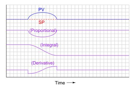
The controller output graph shown here is *qualitative* only. Although drawn to scale (i.e. all changes in the output are properly scaled relative to each other), the scale itself is arbitrary and therefore may not match the scale of your sketch:
