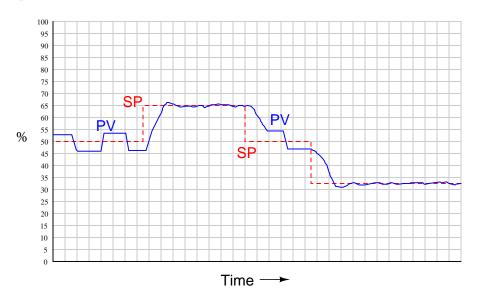
Identify a realistic cause for this strange level-control behavior, and then identify the next step you would take to diagnose and rectify the problem.
