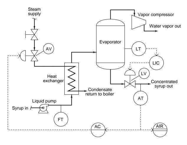
Suppose the analytical control loop has been optimally tuned, with the sugar concentration of the evaporated syrup holding precisely at setpoint. Now suppose the steam supplied to this process by the boiler suddenly increases in temperature. Explain what will happen to the syrup's sugar concentration over time, assuming two different control algorithms, all other factors being equal:
