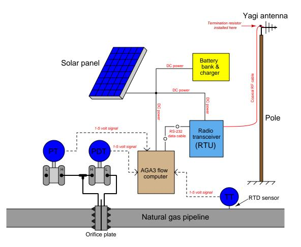
In this installation, the transmission line is a 20 foot length of 50  $\Omega$  coaxial cable. Knowing that reflected signals are bad in any transmission line system, the technician who installed this system also installed a 50  $\Omega$  termination resistor at the antenna-end of the cable, in parallel with the antenna.
