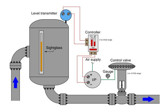
A field operator informs you that a sight glass on this vessel reads 3 feet 9 inches, and the control valve stem position is approximately 40% open.
