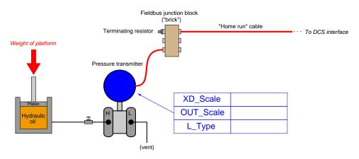
Assuming the circular piston has a diameter of 4 inches, determine the proper XD\_Scale, OUT\_Scale, and L\_Type parameter values to make the transmitter functional over a platform weight range of 0 to 25,000 pounds.
