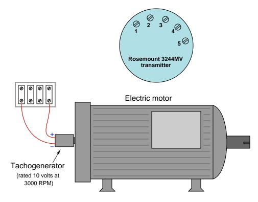
The tachogenerator is nothing more than a small, permanent-magnet DC generator whose output voltage is directly proportional to shaft speed (this one rated 10 volts output at 3000 RPM).
