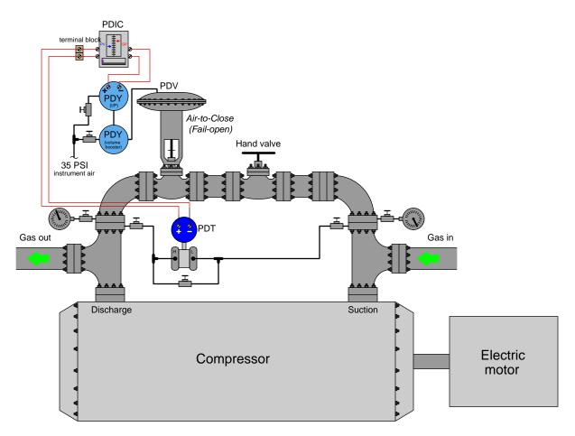
Unfortunately, this system has a problem. The pressure differential indicating controller (PDIC) shows the process variable (PV) being about 50% of range, while the setpoint (SP) is adjusted to 70%. The controller's output indication shows 0%.
