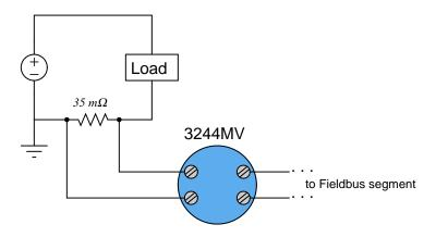
Determine the proper XD\_Scale, OUT\_Scale, and L\_Type parameter values to make the transmitter functional over a DC load current range of 0 to 2.5 amps. <u>file i03642</u>
