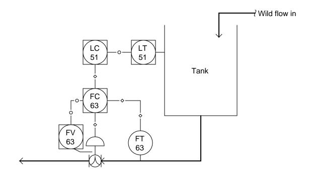
A function block diagram shows how the signals interconnect in this Fieldbus control system:
