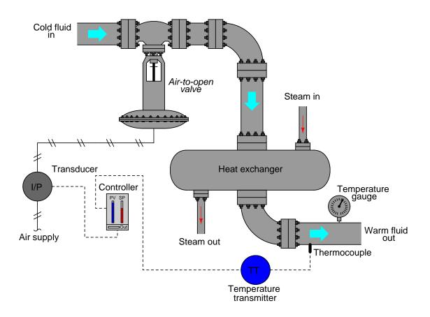
An operator tells you there is a problem with this system, though: the controller faceplate shows the temperature well above setpoint. You happen to notice that the bargraph on the controller faceplate showing output is at 0%. Another operator in the field (near the exchanger) reports via radio that the control valve stem is at the "closed" position.
