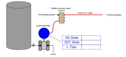
Determine the proper XD\_Scale,  $OUT_Scale$ , and L\_Type parameter values to make the transmitter functional over the entire height of the tank.
