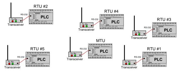
Unfortunately, there is a problem with this system. None of the RTUs are communicating with the MTU. Upon inspection, you see that the "Tx" indicator is blinking on the MTU's transceiver unit but not the "Rx" indicator.
