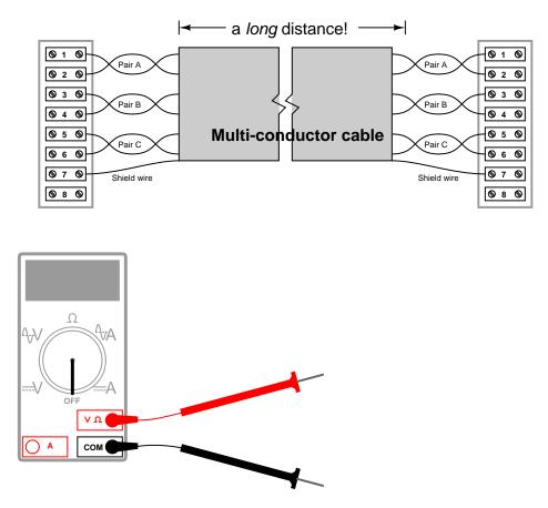
Devise a series of measurements that a technician could take using a multimeter located at one end of the cable, to test for each of the following cable faults. Be sure to specify which setting the multimeter should be configured for, and which terminals the test leads should touch. Also, be sure to specify what range of measurements would indicate "good" versus "bad" for each test:
