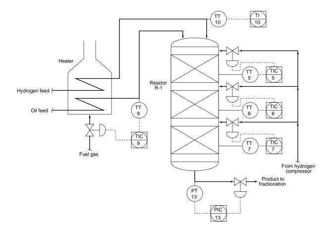
The hydrocracking reaction is exothermic, which means it produces (rather than absorbs) heat. In order to control the reaction temperature and prevent it from "running away," cool hydrogen gas is added to each catalyst bed inside the reactor to *quench* the reaction and regulate its temperature.
