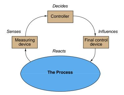
You can check each element of your feedback control loop by comparing its input with its output to see if each element is doing what it should:
