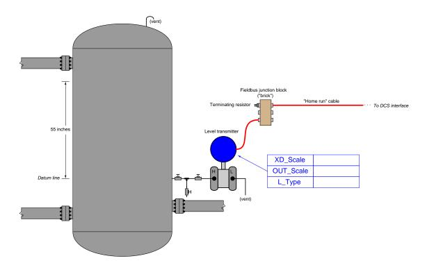
Complete the configuration table in the above illustration, showing the proper XD\_Scale, OUT\_Scale, and L\_Type parameter values to make the transmitter function as it should in this application.
