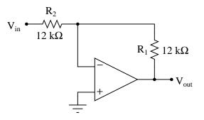
Calculate all voltage drops and currents in this circuit, complete with arrows for current direction and polarity markings for voltage polarity. Then, calculate the overall voltage gain of this amplifier circuit  $(A_V)$ , both as a ratio and as a figure in units of decibels (dB):
