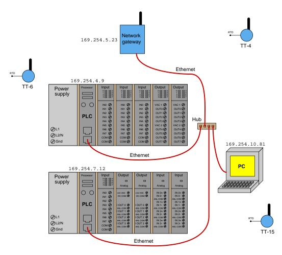
Unfortunately, there is a problem in this system. One PLC (IP = 169.254.4.9) cannot seem to read the temperature sensed by transmitter TT-15. We happen to know that the other PLC (IP = 169.254.7.12) can read the temperatures of the other two *WirelessHART* transmitters (TT-4 and TT-6) just fine, but we don't know if this other PLC can read TT-15's data.
