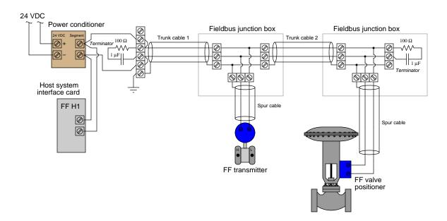
The first step you take in diagnosing this problem is to measure DC voltage with your voltmeter at the terminals of the valve positioner. There, you measure a steady 23.1 volts DC.
