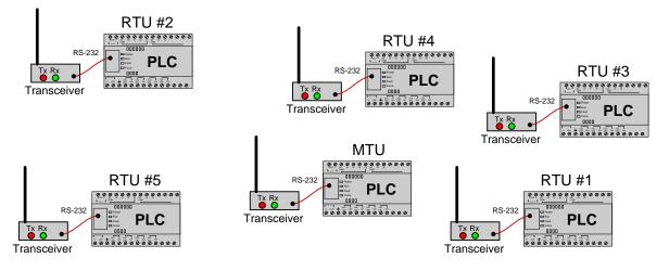
Unfortunately, there is a problem with this system. RTU number 4 does not communicate with the MTU. Upon inspection, you see that the "Tx" and "Rx" LED indicators are blinking on all the RTU radio transceivers except for RTU #4: there, only the "Rx" LED blinks.
