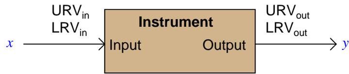
$$\frac{x - LRV_{in}}{URV_{in} - LRV_{in}} = \frac{y - LRV_{out}}{URV_{out} - LRV_{out}}$$
