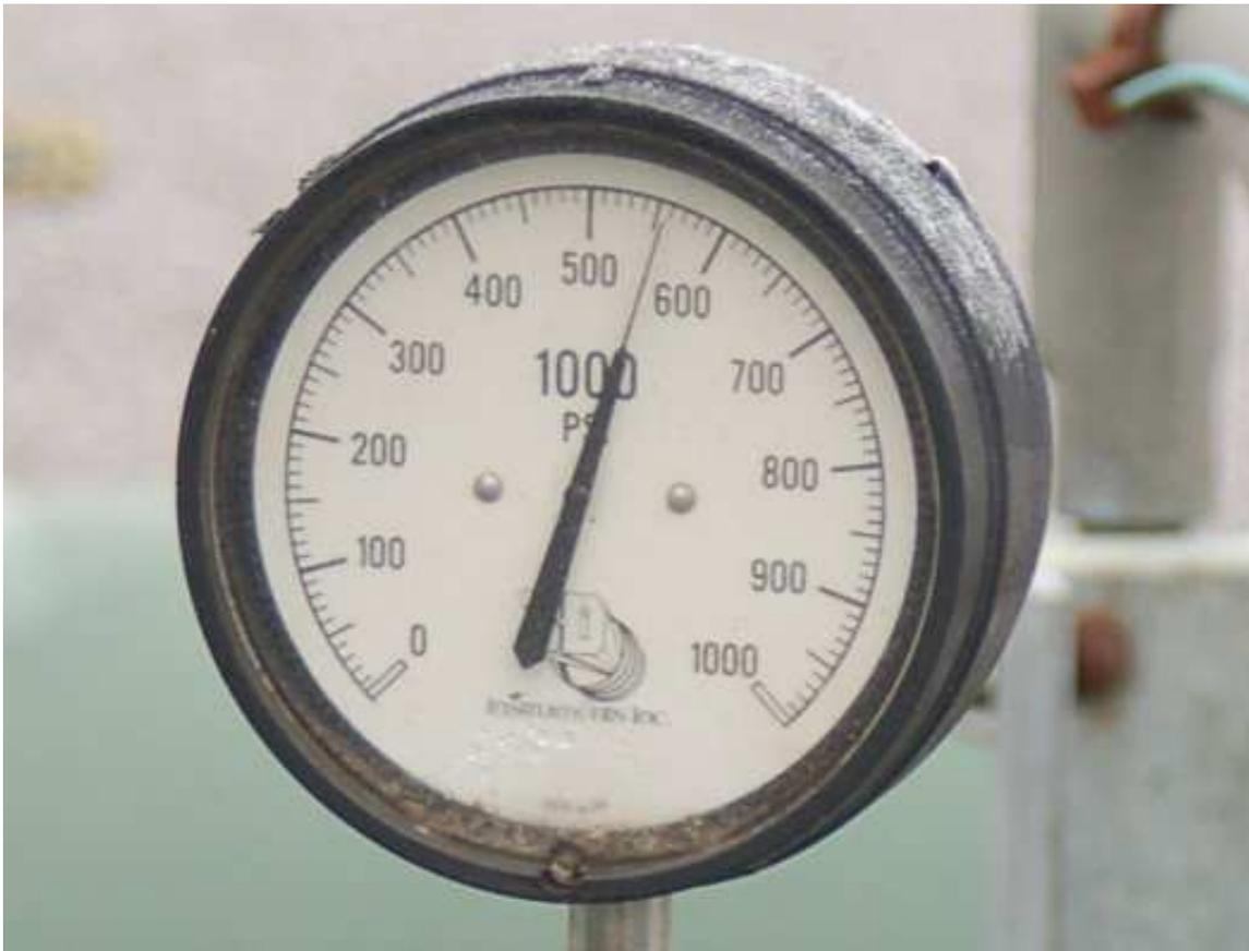
How low and how high could this pressure actually be, given the stated accuracy of this gauge?
