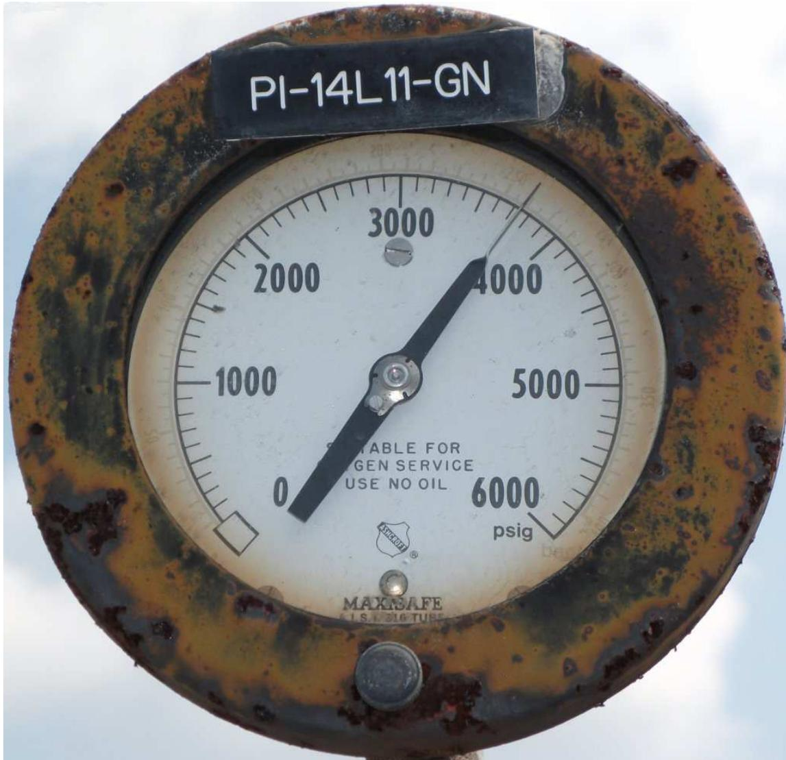
How low and how high could this pressure actually be, given the stated accuracy of this gauge?
