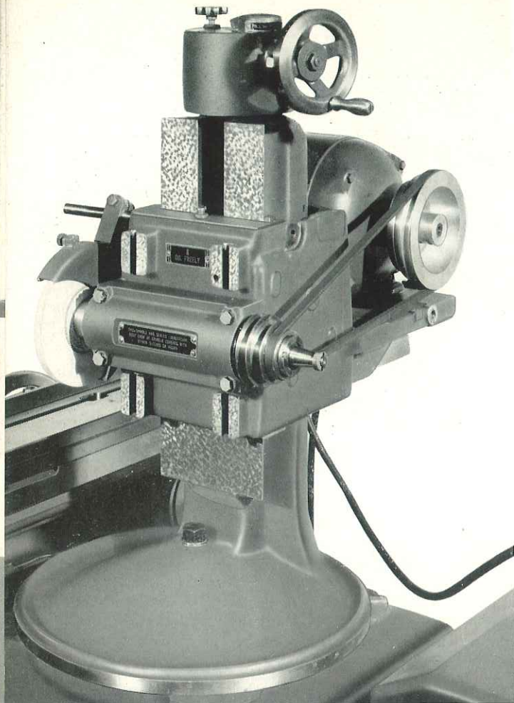
Above —Reliably accurate vertical, transverse and angular settings of the spindle are easily obtained, facilitating a wide variety of set-ups. The elevating screw handwheel may be swiveled to the most convenient operating position, regardless of the angular position of the upright. Note —Belt guard and spindle guard have been removed in above illustration.
