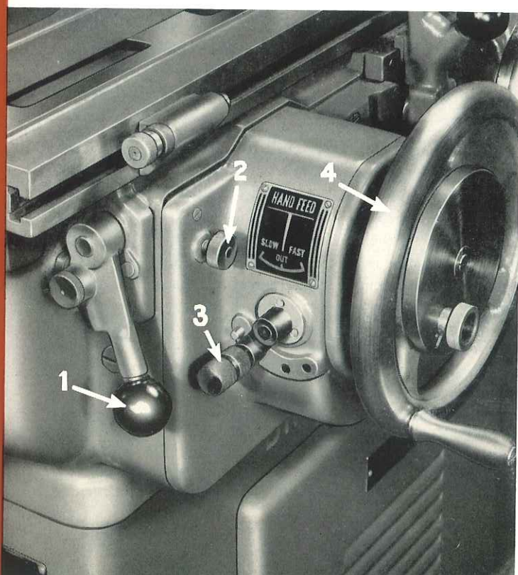
Left —Close-up showing location of controls at left side of the table handwheel.
