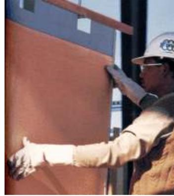
**Figure 11: Sheets of copper cathode produced in electro winning cells**
