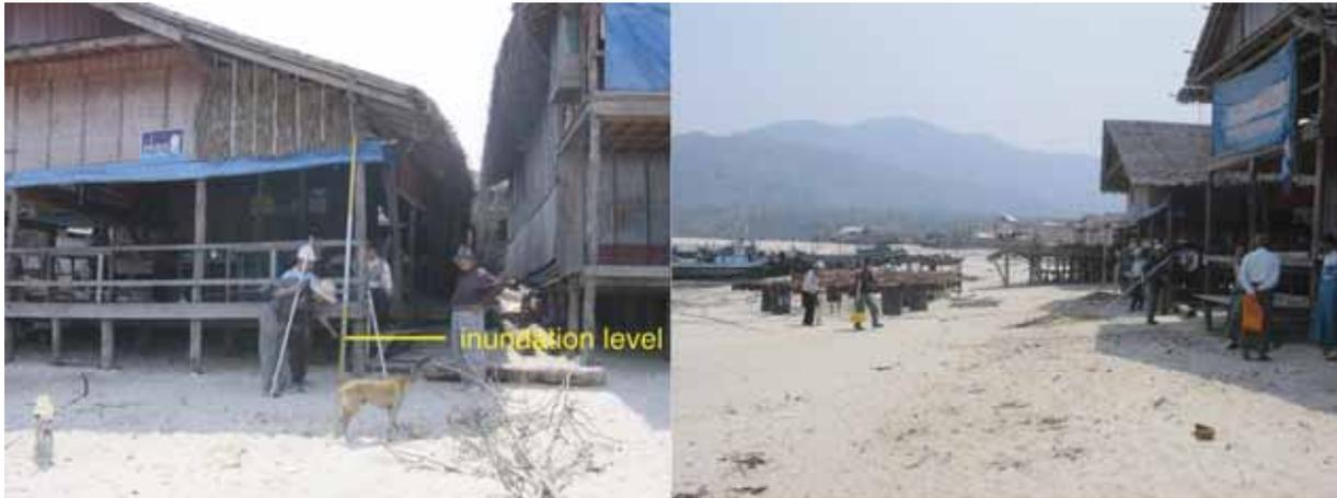
Photo 3. Photographs show survey measurement at Thabawseik-Kyauksent Village. Arrow indicates the height of tsunami (pointed by Interviewee).
