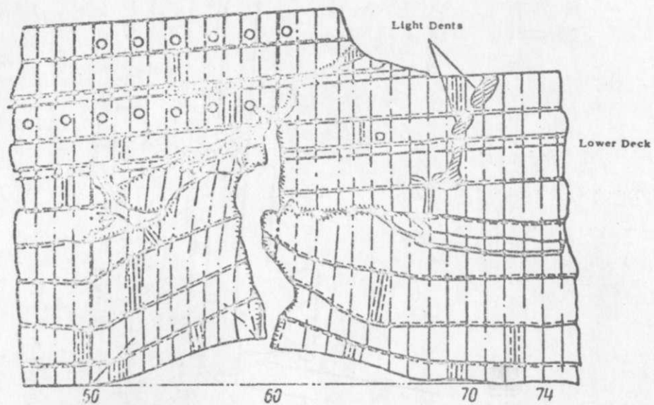
Figure 150 - HUNTER. Damage to Port Side
