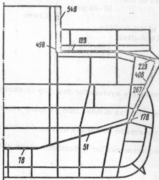
Figure 86 - MUSASHI. Cross-Section in the Vicinity of Main Battery Turret
