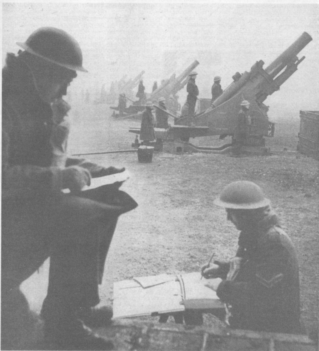
A most impressive suggestion of power is afforded by these 9.2-in. howitzers lined up "somewhere in England." As a result of the strange changes that the mechanization of the Army has brought about, they are now manned by Yeomanry. Their great weight makes it impossible to move them as a whole, so for transport they can be divided into three parts, the barrel, the bed and breech, and the recoil apparatus.
