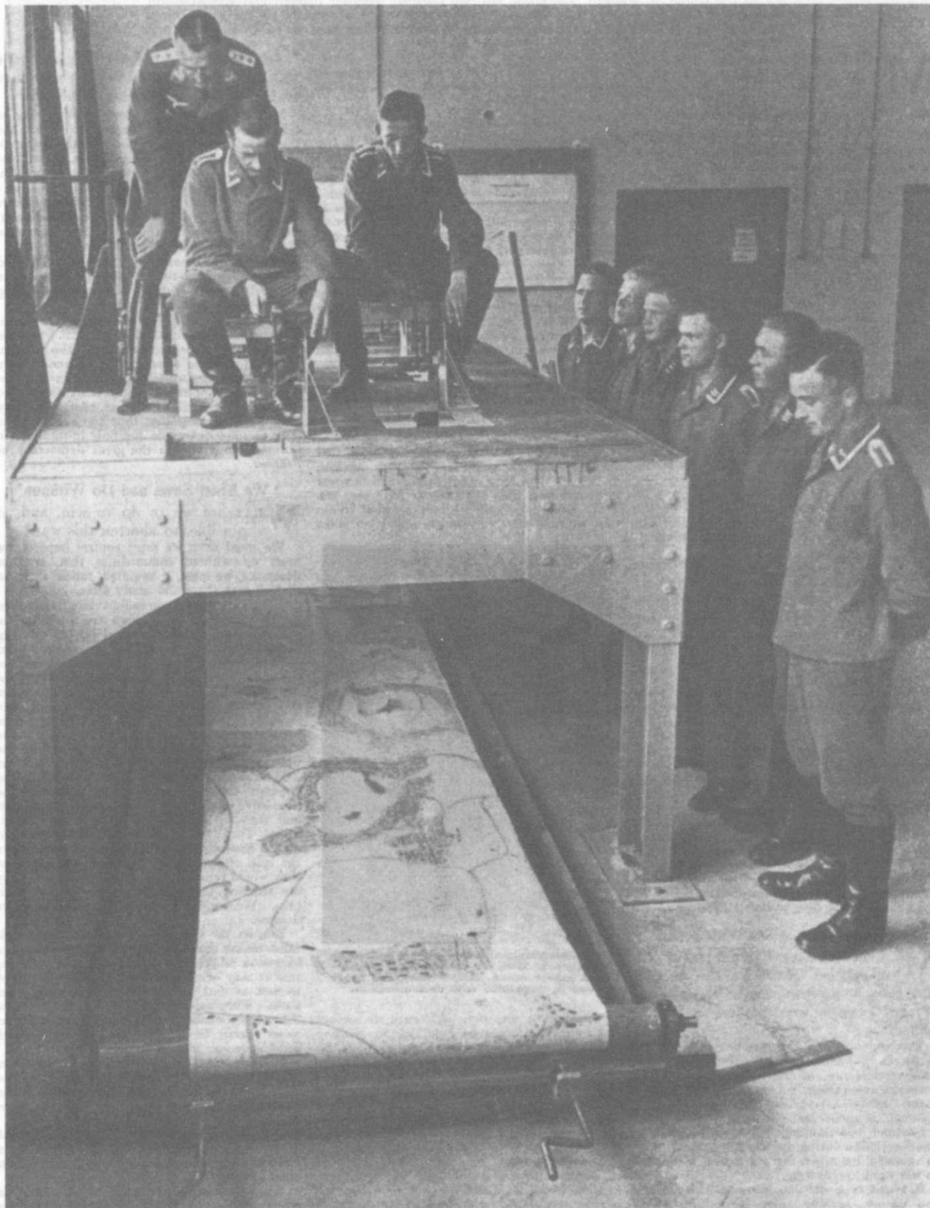
Young Nazi airmen are put through an intensive course of training. They are here learning the far from gentle art of bombing. In this ingenious apparatus a map on rollers passes beneath the pupil showing a stretch of country as nearly as possible as it would appear seen from an aeroplane flying at a great height and speed. When the lever releasing the bomb is pulled the aim is automatically registered on the map.
