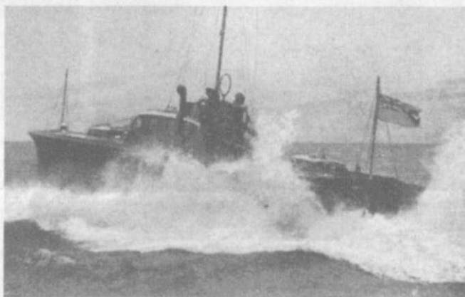
A recent addition to the fleet of motor boats of the R.A.F. is the fast launch seen above. She is designed as a rescue ship, and in her small hull has sick berth accommodation for twenty injured persons.
