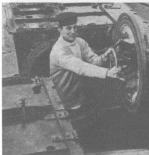
Once alongside the parent ship the men below are soon on deck. The one left, coming on deck, has his hands on the wheel by which the hatch is screwed down to make it watertight. On board the depot ship the first call is for letters from home, and then most of the bearded men enjoy a shave, like the one right.
