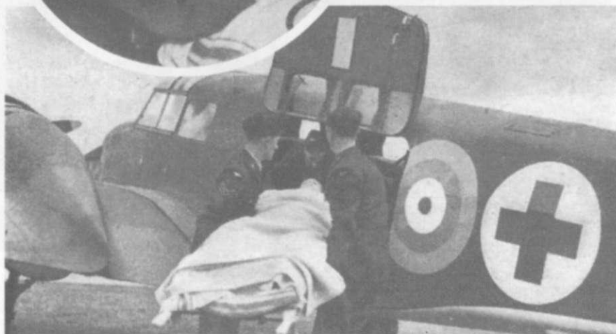
The ambulance 'planes might almost be called flying hospitals, for among other equipment they carry oxygen cylinders. In the circle, oxygen is being administered. Above, a stretcher case is being put on board. As can be seen in the photograph, top right, the undercarriages of the ambulance 'planes are exceptionally low, so that access to the interior is easy.
