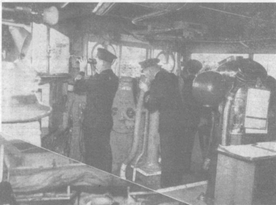
The control of a battleship is a very complicated matter compared with what it was thirty or forty years ago—as the photograph above, taken on the compass platform of a battleship at sea, shows. The navigating officer, centre, is giving instructions; on his left is the officer of the watch, while one of innumerable "gadgets" is the magnetic compass, right.
