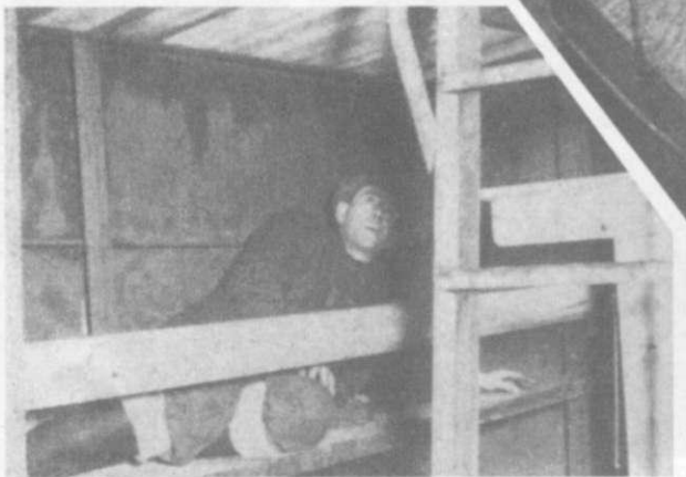
ON THE REFUGE-BUOY below deck four bunks are installed. No one was aboard this buoy when it drifted ashore. Right may be seen the steel watertight hatch by which the cabin is reached.
