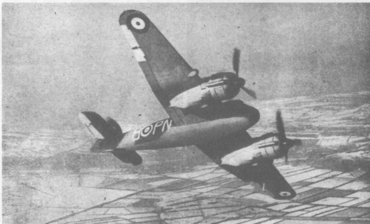
THE BRISTOL BEAUFIGHTER (above) is a twin-engined, high speed, heavily-armed fighter monoplane produced by the Bristol Aeroplane Co., the firm responsible for the Beaufort, Blenheim and Bombay aircraft. The Beaufighter is suitable for use either as a day or night interceptor, and has proved a very useful weapon against the German night bombers. This is the first photo of a Beaufighter to be officially released.
