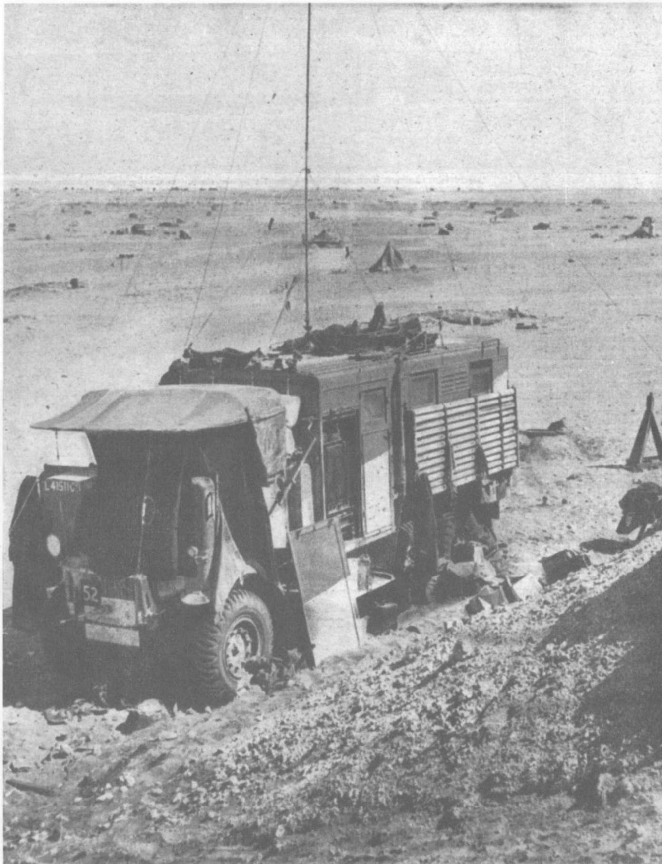
BRITISH MOBILE RADIO CAR in action somewhere in the Western Desert. The nerve centre of operations, this type of car can remain in the desert as long as necessary and open up communications by Morse at the rate of about thirty words a minute, or by telephony. It has a range of over a thousand miles. In the background as far as the horizon are military tents, but no soldiers are to be seen. They have probably taken refuge from the intense heat.
