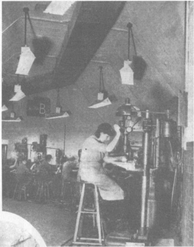
Section of a drilling shop already in operation in what was once a chalk mine. Air conditioning plant is installed, and all vital departments of underground factories are immune from enemy action.
