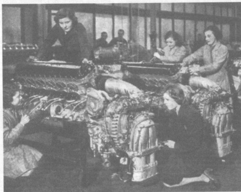
ROLLS-ROYCE MERLIN XX aero-engines in production. Women war-workers have quickly adapted themselves to precision engineering, and these girls are seen at work in a corner of the assembly shop.
