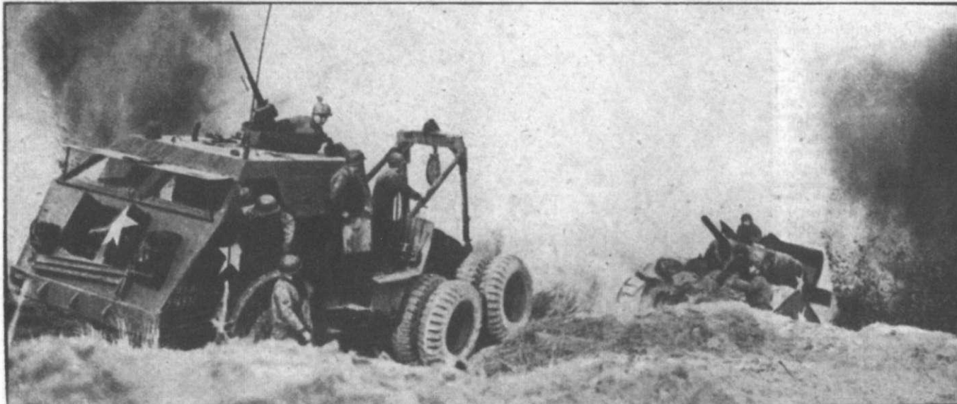
GIANT RESCUER OF DISABLED TANKS or other heavy Army vehicles is the American M-25, seen here during manoeuvres in Britain hauling a tank out of a bomb crater, while actual explosions simulate real war conditions. This tank recovery vehicle, completely enclosed in armour, has a crew of 7 highly skilled technicians; it can carry up to 40 tons at a speed of 28 m.p.h. and is armed against attack. It is equipped with comprehensive repair equipment, and can move through water. Photo, U.S. Official
