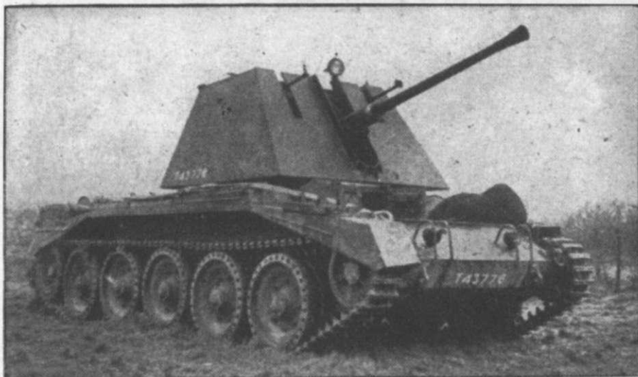
CRUSADER BOFORS A.A. TANK , in operation against the enemy in Europe, is a development of the Bofors 40-mm. S.P. (self-propelled) gun mentioned in this page. Designed primarily for the protection of convoys on the move against low-flying aircraft, it fires 2-lb. shells at the rate of 120 per minute. Photo, British Official
