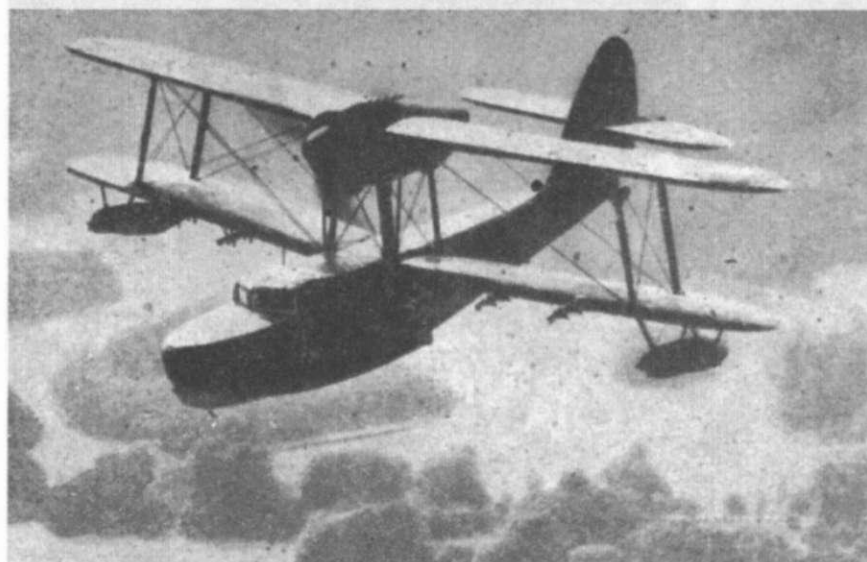
VICKERS-ARMSTRONG SEA-OTTER MARK I , seen in flight, is a single-engined amphibian biplane designed for naval reconnaissance and air-sea rescue purposes. It has catapult equipment and is powered with a Bristol Mercury 30 engine of 870 h.p.; is armed with three Vickers "K" guns and carries a crew of three or four.
