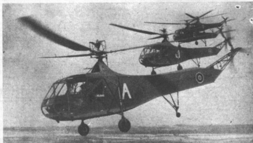
SIKORSKY R4B HELICOPTERS OF THE R.A.F., photographed for the first time flying in formation, at an R.A.F. training school. Capable of rising vertically, flying backwards, forwards or sideways, and hovering to drop or pick up passengers, these aircraft are expected to play an important part in Britain's post-war aerial development. Photo, Planet News
