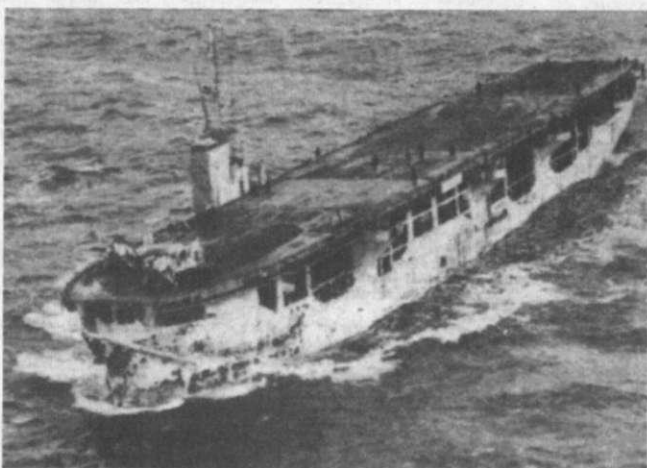
THE M.A.C. ANCYLUS, a British merchant ship equipped with flight deck for the launching and landing of Fleet Air Arm fighter aircraft during the most critical period of the Battle of the Atlantic, as described by Capt. Frank H. Shaw in this page. Photo, British Official
