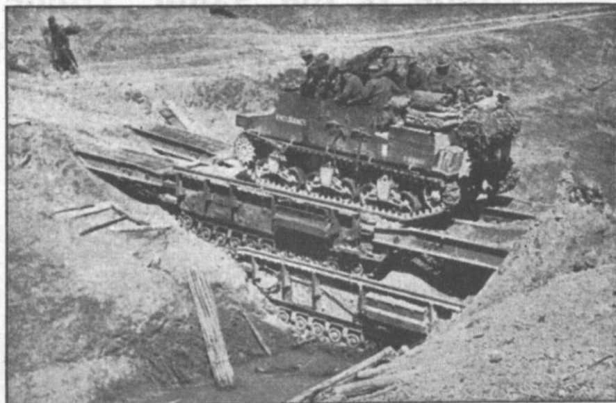
SPECIAL BRIDGING DEVICE KNOWN AS THE ARK , which helped us defeat Germany and is being used in Burma, can now be revealed as a tank on which are mounted two ramps for dropping down at front and rear. Here, two of these ingenious bridging-tanks are ditched one on top of the other, and the ramps have been lowered, enabling British armour to cross a shellhole in Germany. See also illus. page 229. Photo, British Official
